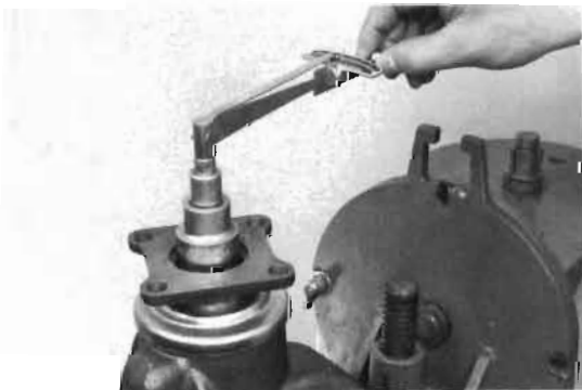
Adjusting Shim and Washer Thickness
