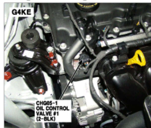
36. Right Front of Engine Room
