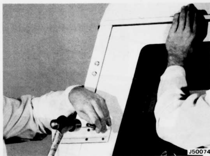
Fig. 2-22 Marking Hole Locations for Upper Male-Half Hinges
