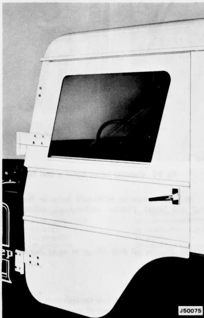
Fig. 2-7 Door and Hinges Installed
