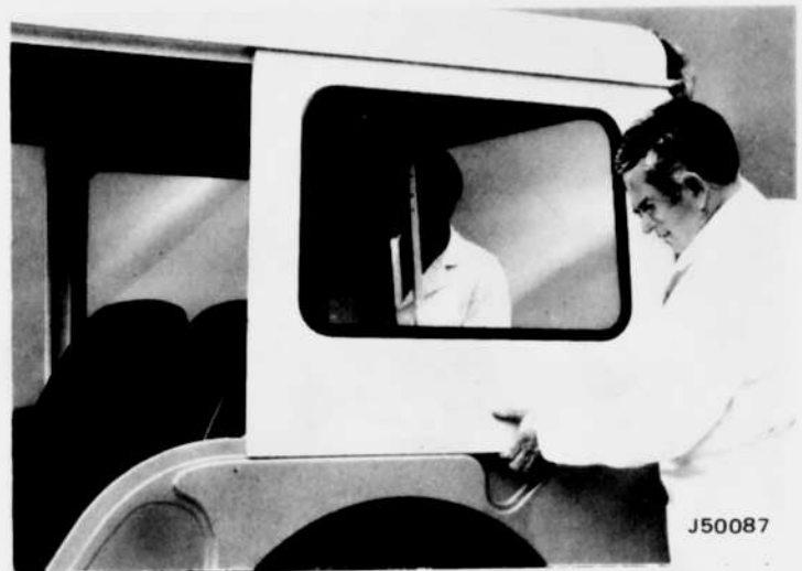
Fig. 2-19 Mounting Roof-Quarter Panel Assembly on Body
