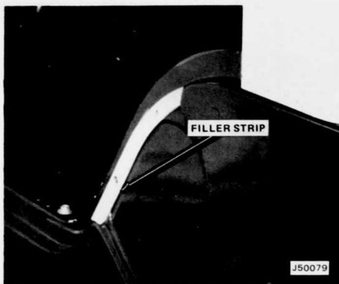
Fig. 2-11 Filler Strip Installed
