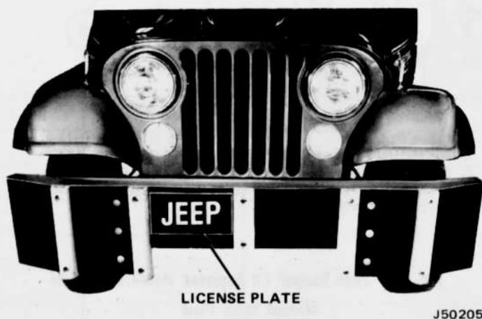
Fig. 3-4 Push Bumper Installed
