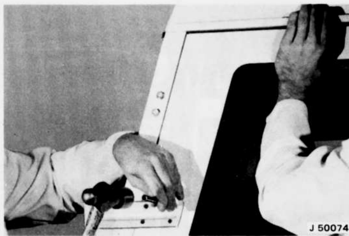
Fig. 2-6 Marking Hole Locations for Half-Hinges
