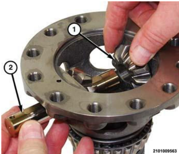
Fig. 553: Removing/Installing Pinion Gear 1 Courtesy of CHRYSLER GROUP, LLC
