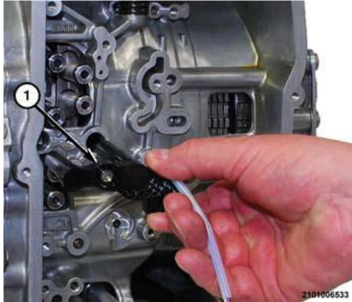
Fig. 186: Removing/Installing Speed Sensor Courtesy of CHRYSLER GROUP, LLC
