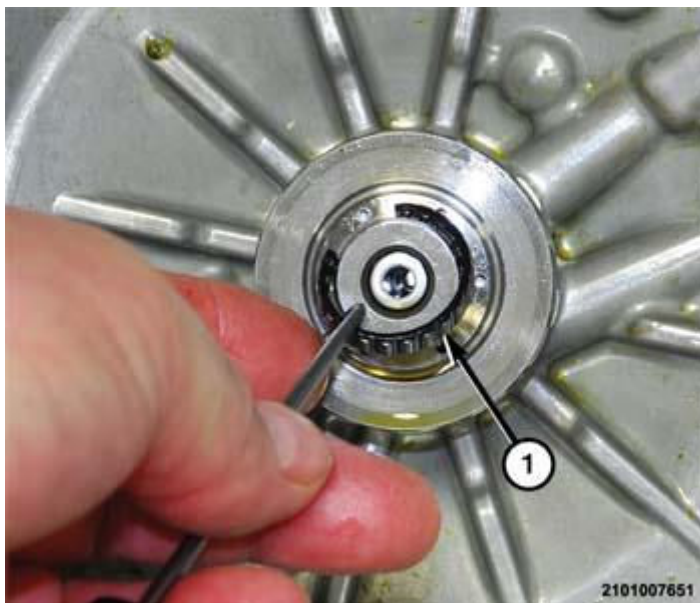
Fig. 122: Removing/Installing Split Roller Bearing Courtesy of CHRYSLER GROUP, LLC
