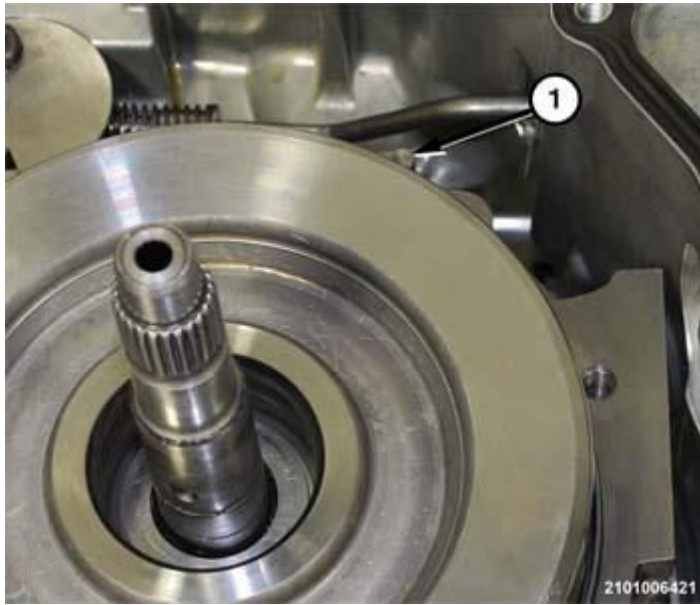
Fig. 181: Checking Guide Pin Alignment Courtesy of CHRYSLER GROUP, LLC
