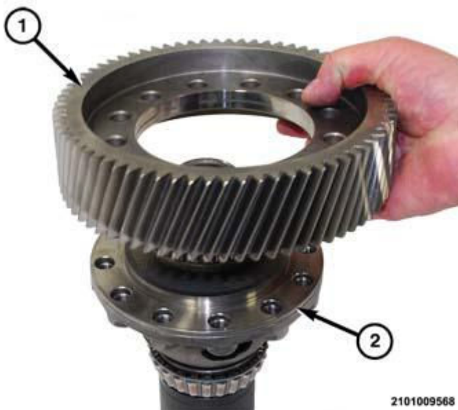
Fig. 499: View Of Ring Gear & Differential Unit Courtesy of CHRYSLER GROUP, LLC
