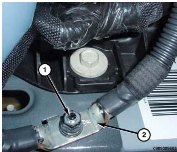
Fig. 33: Nut & Wire Harness Courtesy of CHRYSLER GROUP, LLC
