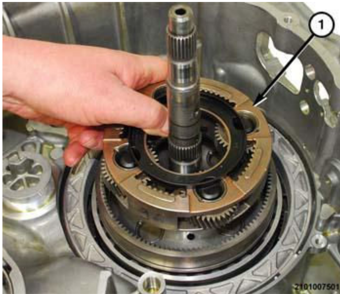
Fig. 167: Gear 4 Planetary Pinion Carrier Courtesy of CHRYSLER GROUP, LLC
