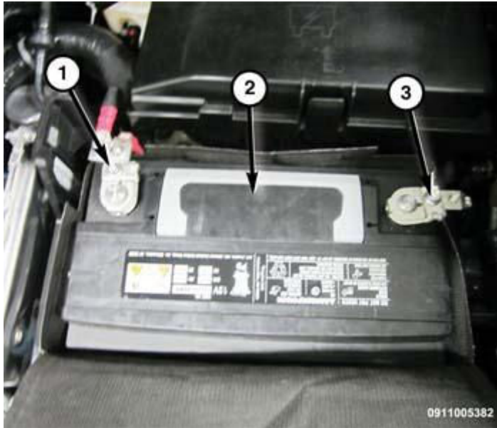
Fig. 135: Battery & Cables Courtesy of CHRYSLER GROUP, LLC
