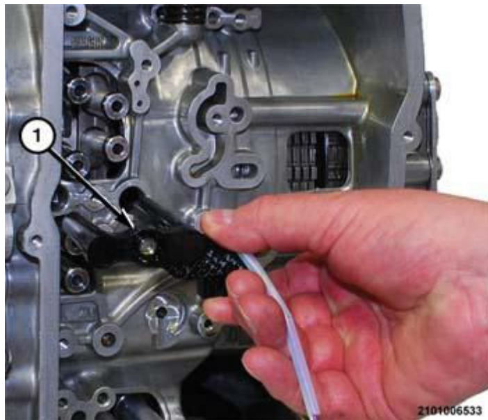
Fig. 664: Removing/Installing Speed Sensor Courtesy of CHRYSLER GROUP, LLC
