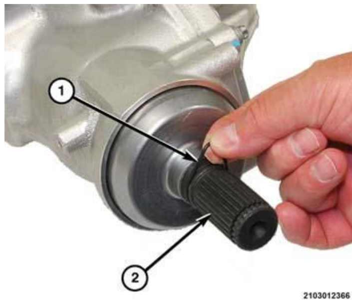
Fig. 63: Removing/Installing O-Ring At Rear Output Shaft Courtesy of CHRYSLER GROUP, LLC
