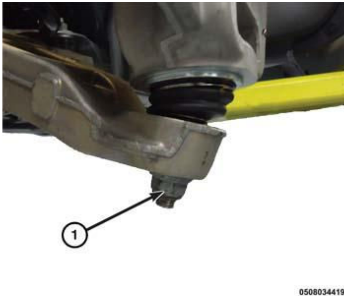
Fig. 35: Identifying Lower Ball Joint Nut Courtesy of CHRYSLER GROUP, LLC
