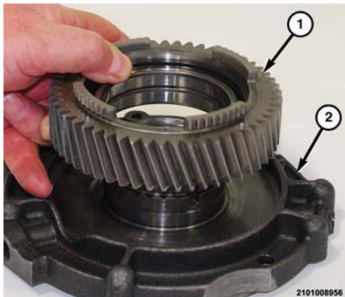
Fig. 481: Removing/Installing Output Gear Courtesy of CHRYSLER GROUP, LLC
