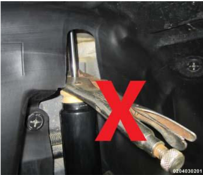
Fig. 39: Identifying Pliers On Chrome Machined Surface Of Shock/Strut Rod Courtesy of CHRYSLER GROUP, LLC
