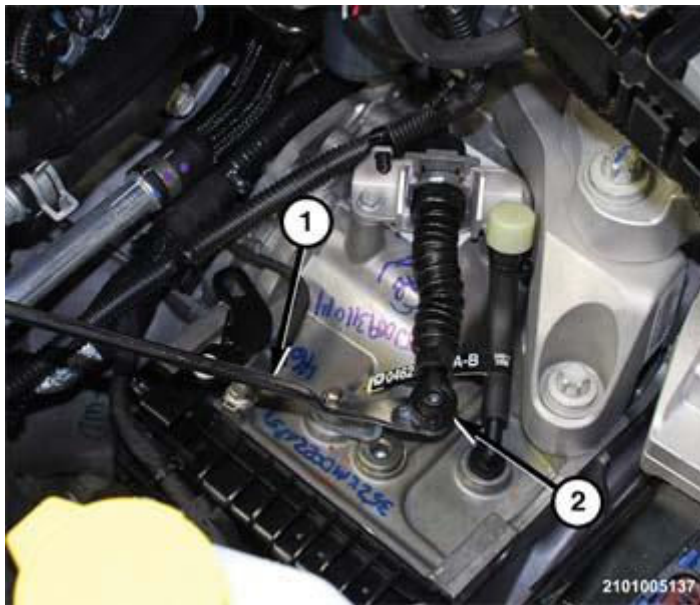
Fig. 574: View Of Ground Cable & Shift Cable Courtesy of CHRYSLER GROUP, LLC
