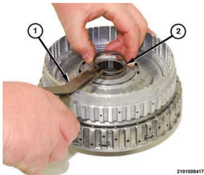
Fig. 104: Remove/Install Snap-Ring Courtesy of CHRYSLER GROUP, LLC
