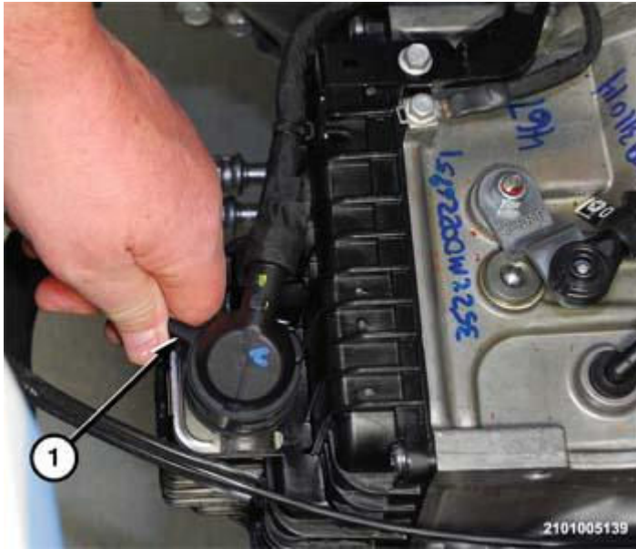
Fig. 42: Transmission Valve Body Solenoid Connector Courtesy of CHRYSLER GROUP, LLC
