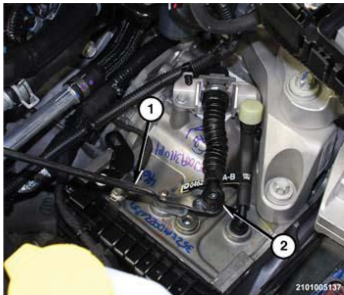
Fig. 223: View Of Ground Cable & Shift Cable Courtesy of CHRYSLER GROUP, LLC
