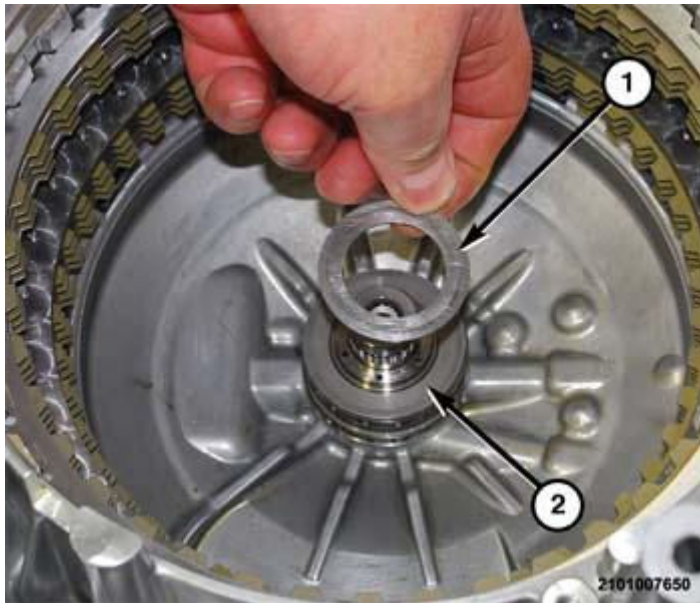
Fig. 137: Removing/Installing Input Shaft Rear Support Selective Thrust Washer Courtesy of CHRYSLER GROUP, LLC
