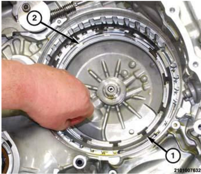
Fig. 116: C-Clutch Bellville Spring & C-Clutch Piston Courtesy of CHRYSLER GROUP, LLC
