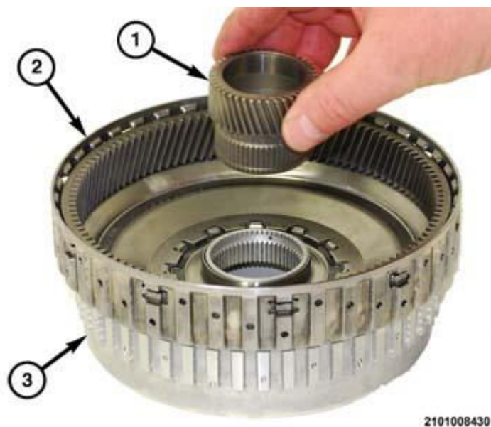
Fig. 105: Annulus Gear 2, D And C-Clutch Hub (3) & Sun Gear 1 Courtesy of CHRYSLER GROUP, LLC
