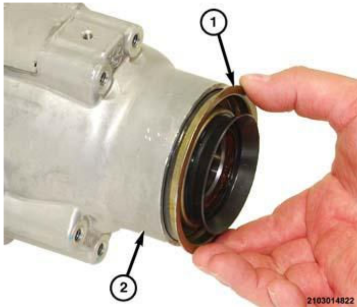
Fig. 49: Placing New Lip Seal Into Position On PTU Housing Courtesy of CHRYSLER GROUP, LLC
