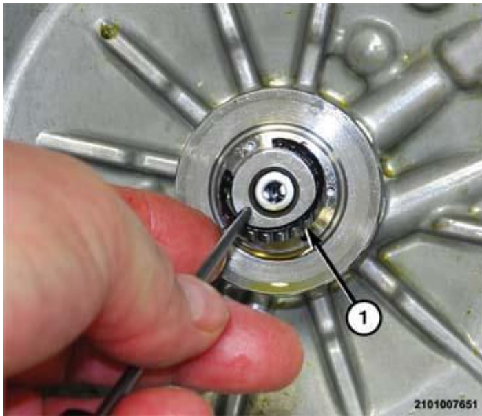
Fig. 121: Removing/Installing Split Roller Bearing Courtesy of CHRYSLER GROUP, LLC
