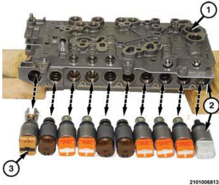
Fig. 734: Solenoid Valves & Outer Valve Body Courtesy of CHRYSLER GROUP, LLC
