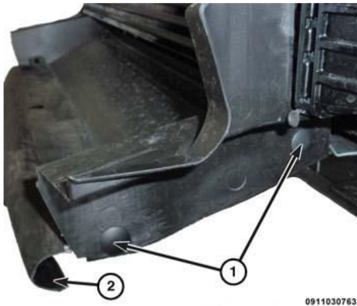
Fig. 333: Left Side Air Deflector Pushpin Retainers Courtesy of CHRYSLER GROUP, LLC
