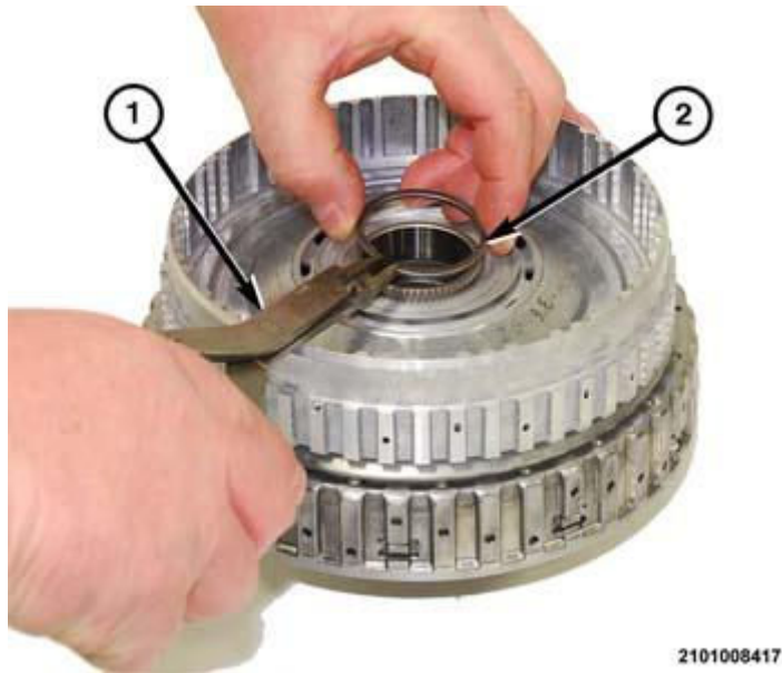
Fig. 144: Remove/Install Snap-Ring Courtesy of CHRYSLER GROUP, LLC
