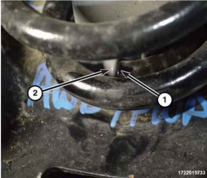
Fig. 34: Identifying Lower End Of Spring & Spring Isolator Courtesy of CHRYSLER GROUP, LLC
