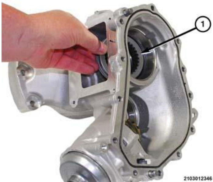
Fig. 13: Locating Dog Clutch Sleeve Courtesy of CHRYSLER GROUP, LLC
