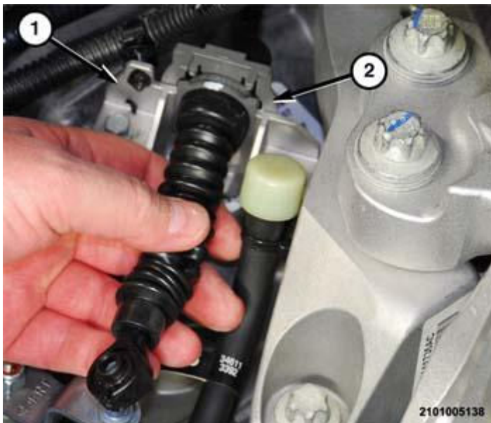
Fig. 43: View Of Shift Cable Housing & Mount Bracket Courtesy of CHRYSLER GROUP, LLC
