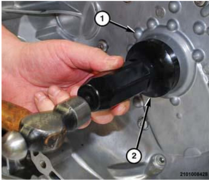
Fig. 662: Installing Seal Into Bellhousing Courtesy of CHRYSLER GROUP, LLC
