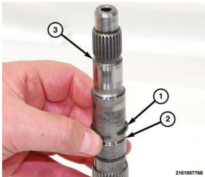
Fig. 101: Remove/Install Input Shaft Seal-Rings Courtesy of CHRYSLER GROUP, LLC
