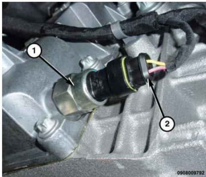
Fig. 7: Reverse Lamp Sensor & Wire Harness Connector Courtesy of CHRYSLER GROUP, LLC
