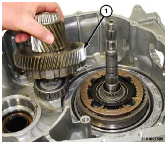
Fig. 337: Removing/Installing Transfer Gear Courtesy of CHRYSLER GROUP, LLC
