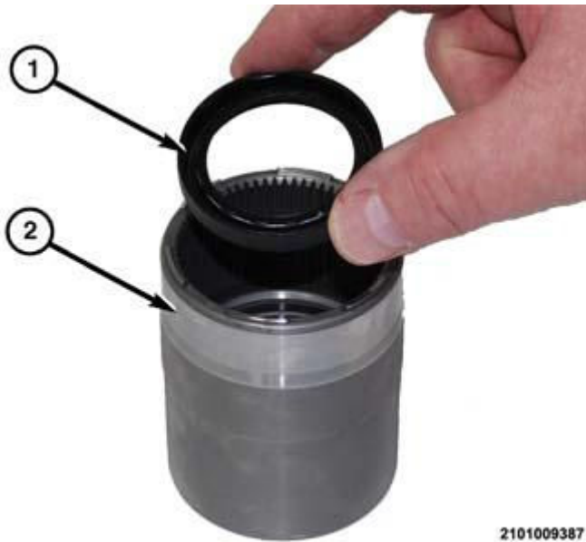
Fig. 653: Inserting Lip Seal Into Adapter Sleeve Courtesy of CHRYSLER GROUP, LLC
