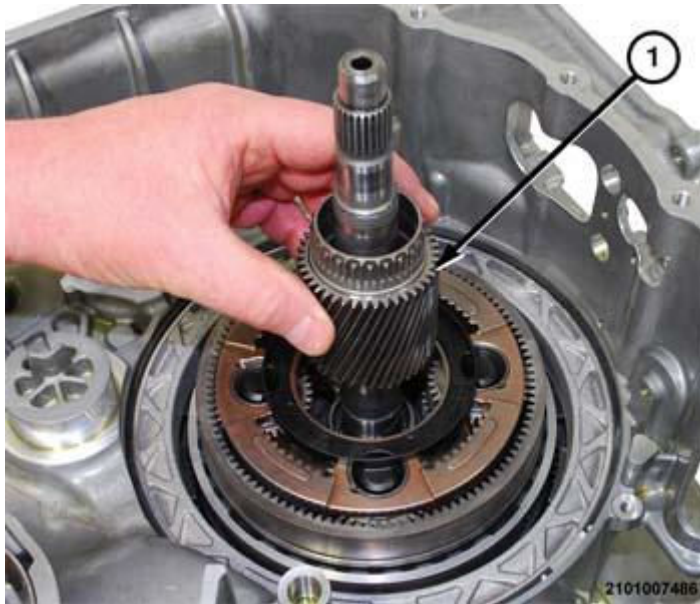
Fig. 81: Removing/Installing Sun Gear 3, 4 And Dog Clutch-F At Gear 4 Planetary Pinion Carrier Courtesy of CHRYSLER GROUP, LLC
