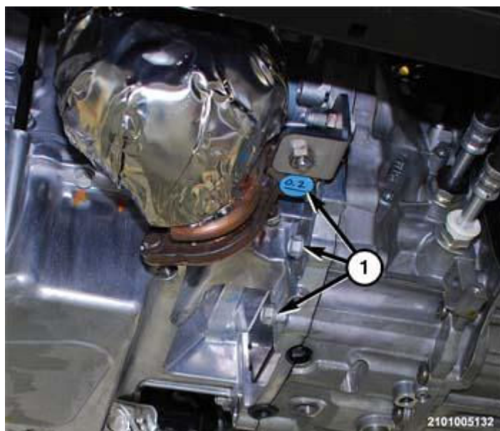
Fig. 39: Removing/Installing Transmission Bellhousing Bolts Courtesy of CHRYSLER GROUP, LLC
