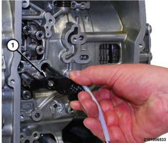
Fig. 352: Removing/Installing Speed Sensor Courtesy of CHRYSLER GROUP, LLC
