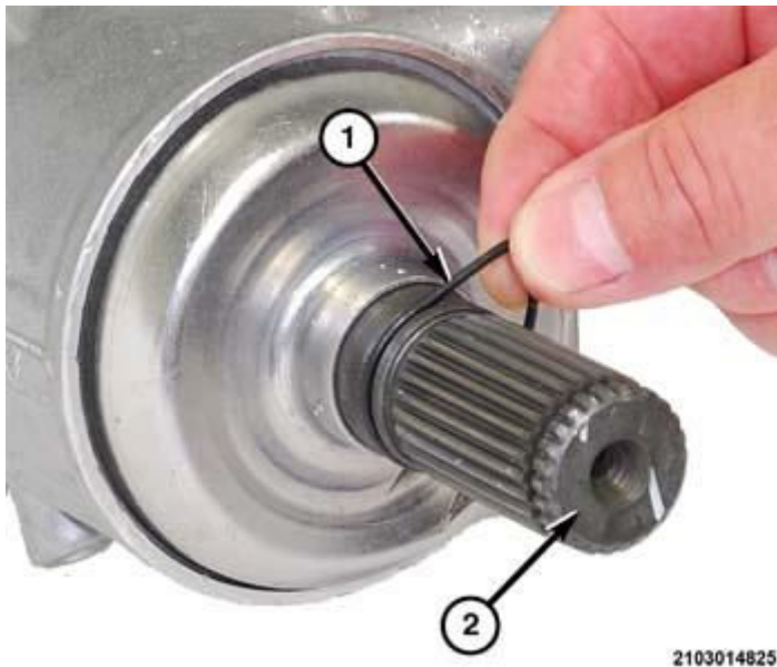
Fig. 69: Removing/Installing O-Ring At Rear Output Shaft Courtesy of CHRYSLER GROUP, LLC
