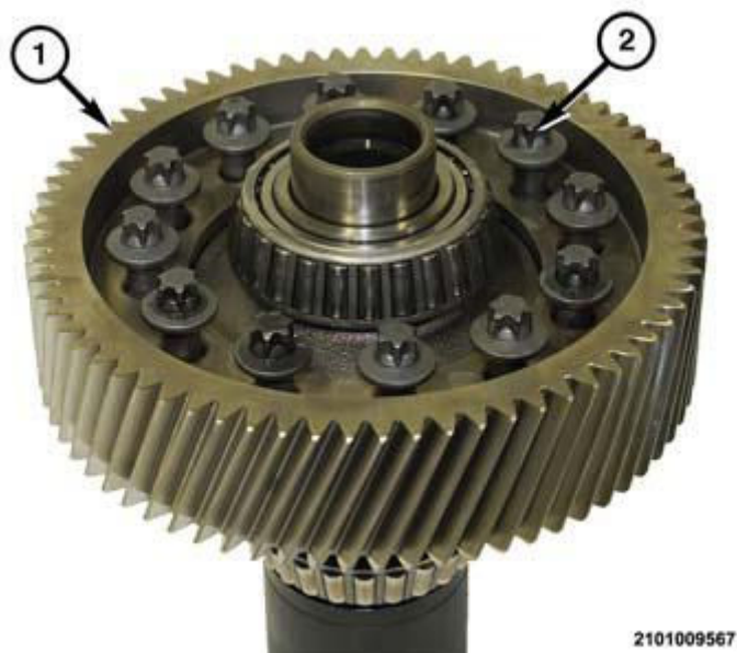
Fig. 498: View Of Ring Gear To Differential Unit & Bolts Courtesy of CHRYSLER GROUP, LLC
