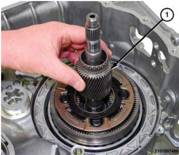
Fig. 323: Removing/Installing Sun Gear 3, 4 And Dog Clutch-F At Gear 4 Planetary Pinion Carrier Courtesy of CHRYSLER GROUP, LLC
