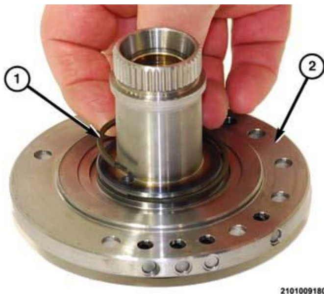
Fig. 675: Removing/Installing Seal Ring At Ring Land In Outer Reaction Shaft Hub
