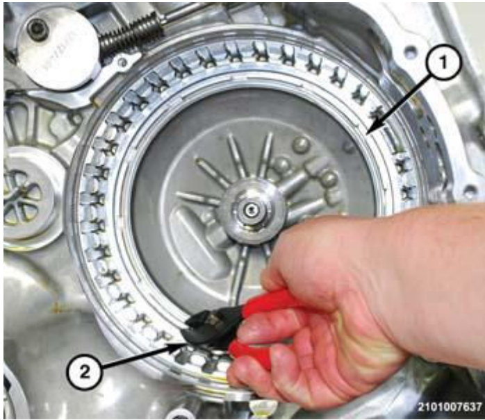
Fig. 127: Removing/Installing C-Clutch Piston Courtesy of CHRYSLER GROUP, LLC
