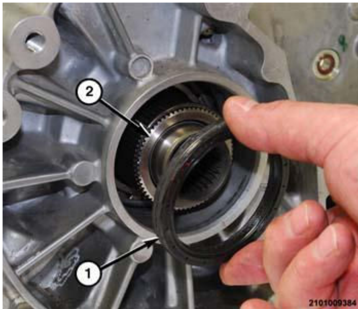
Fig. 659: Inserting Lip Seal Into Transmission Courtesy of CHRYSLER GROUP, LLC
