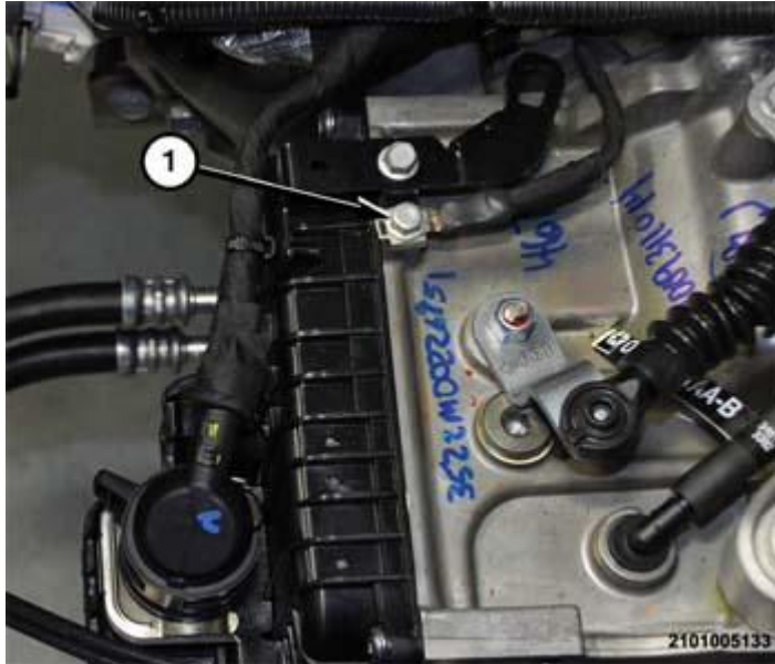
Fig. 41: Ground Cable At Top Transmission Courtesy of CHRYSLER GROUP, LLC
