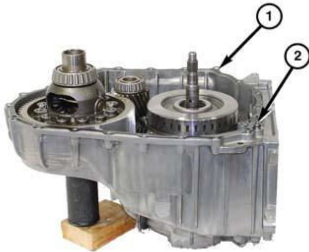
Fig. 177: Sealing Surface Of Transmission Housing Courtesy of CHRYSLER GROUP, LLC
