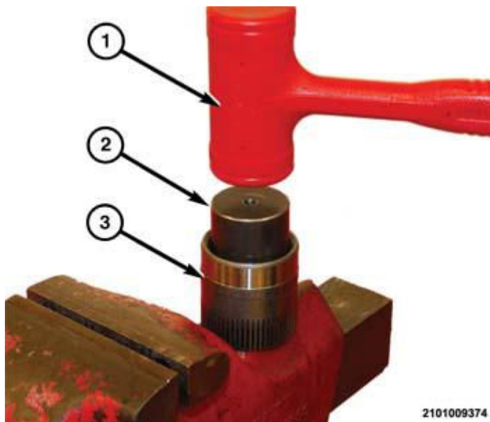
Fig. 654: Installing Seal Into Adapter Sleeve Courtesy of CHRYSLER GROUP, LLC
