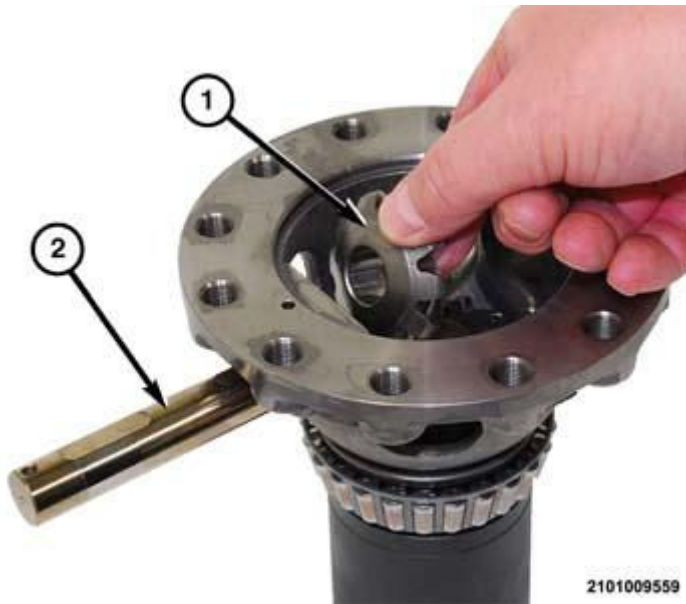
Fig. 493: Removing/Installing Pinion Shaft & Pinion Gear 2 Courtesy of CHRYSLER GROUP, LLC
