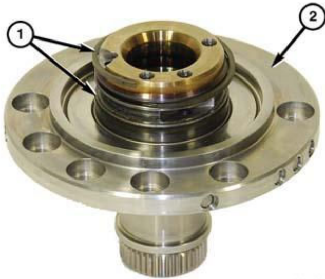
Fig. 676: Removing/Installing Seal Rings At Ring Land In Inner Reaction Shaft Hub Courtesy of CHRYSLER GROUP, LLC
