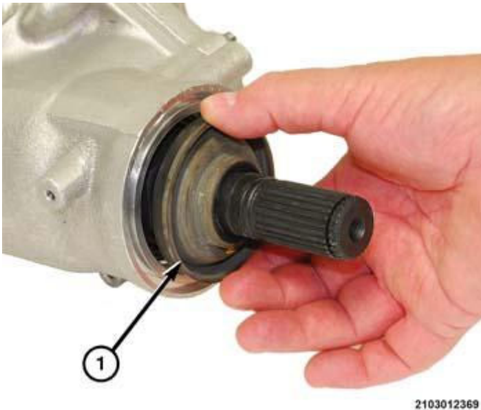
Fig. 59: Placing New Seal In Position On PTU Output Shaft Courtesy of CHRYSLER GROUP, LLC
