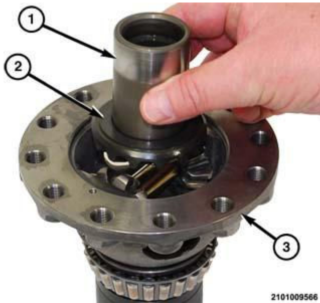
Fig. 532: Differential Side Gear & Thrust Washer Courtesy of CHRYSLER GROUP, LLC
