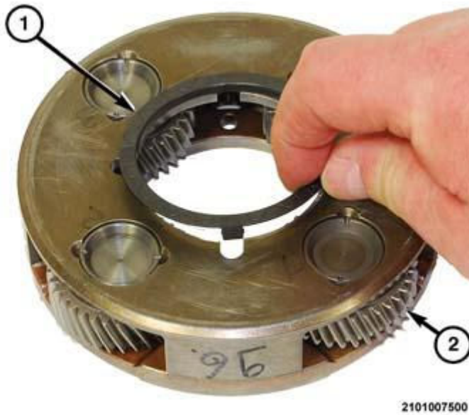
Fig. 332: Thrust Spacer & Underside Of Gear 4 Planetary Pinion Carrier Courtesy of CHRYSLER GROUP, LLC
