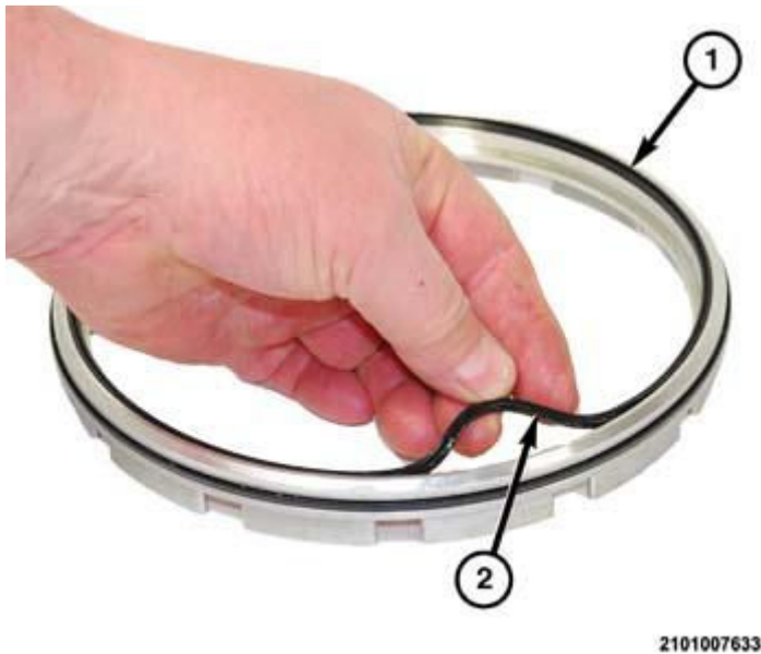
Fig. 125: Installing Inner Seal On C-Clutch Piston Courtesy of CHRYSLER GROUP, LLC
