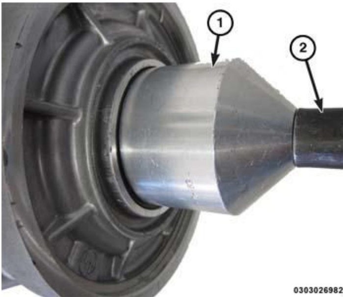
Fig. 45: Installing The Output Seal Using Special Tool Courtesy of CHRYSLER GROUP, LLC
