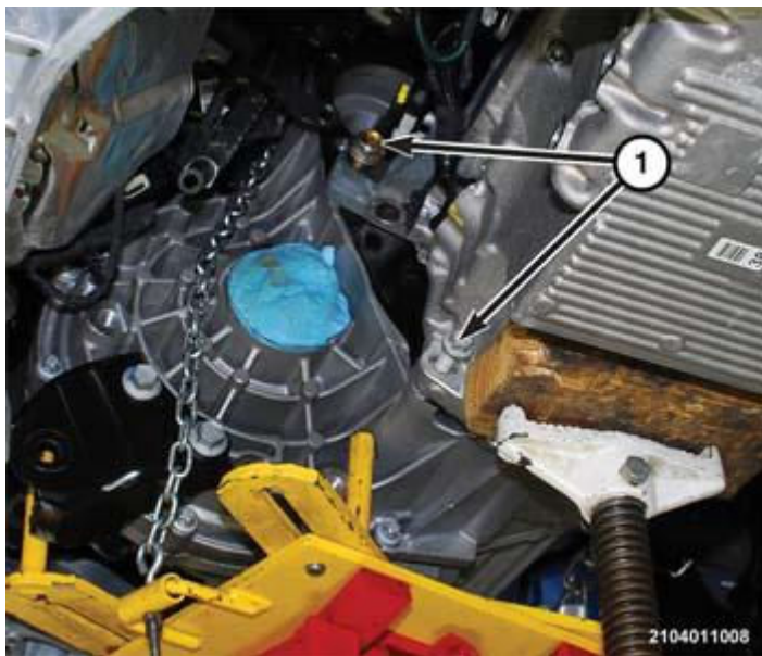
Fig. 21: Locating Bolts Holding Engine Block To Transmission Bellhousing & Bellhousing To Oil Pan
