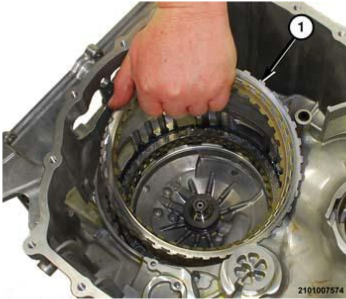
Fig. 110: Removing D-Clutch Friction Discs & Steel Plates From Transmission Housing Courtesy of CHRYSLER GROUP, LLC
