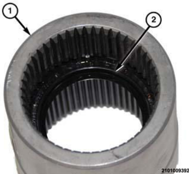
Fig. 648: View of Adapter Sleeve Seal Tension Spring Courtesy of CHRYSLER GROUP, LLC
