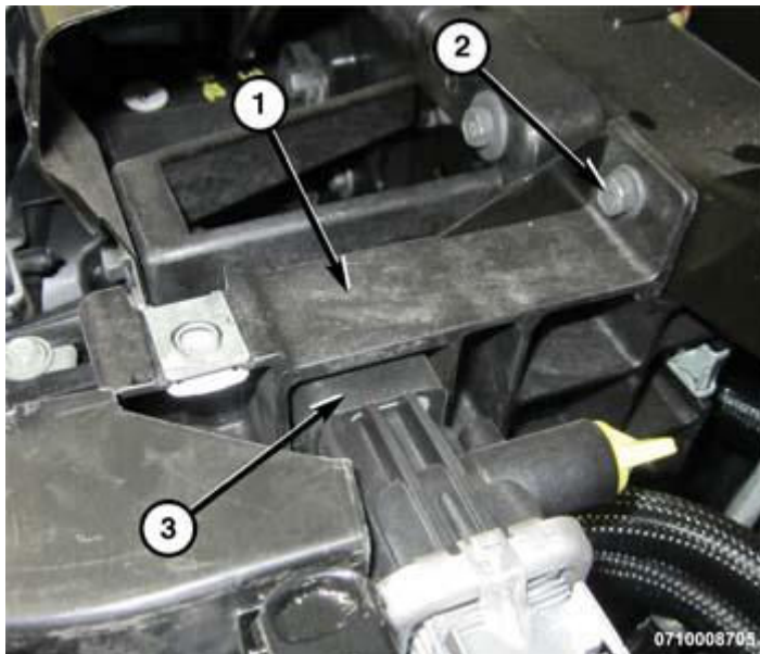
Fig. 94: Removing/Installing Upper Radiator Mounts
