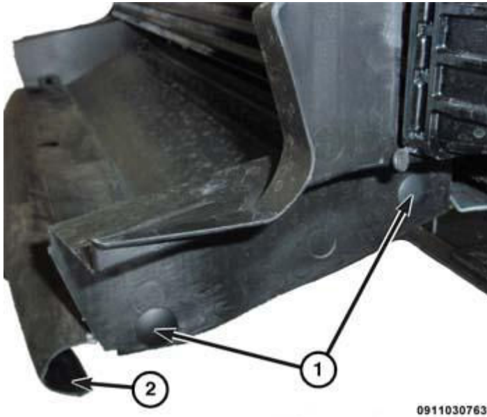
Fig. 344: Left Side Air Deflector Pushpin Retainers Courtesy of CHRYSLER GROUP, LLC
