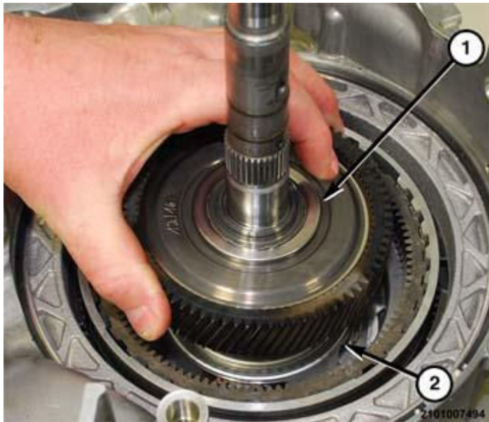
Fig. 161: Annulus Gear 1 Planetary Hub & Carrier Gear 1 And 2 Courtesy of CHRYSLER GROUP, LLC
