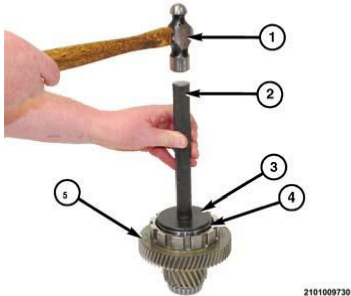
Fig. 367: Installing Bearing Race Into Transfer Gear Until Courtesy of CHRYSLER GROUP, LLC
