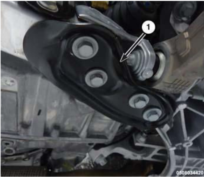
Fig. 75: Identifying Lower Load Beam Bracket Courtesy of CHRYSLER GROUP, LLC
