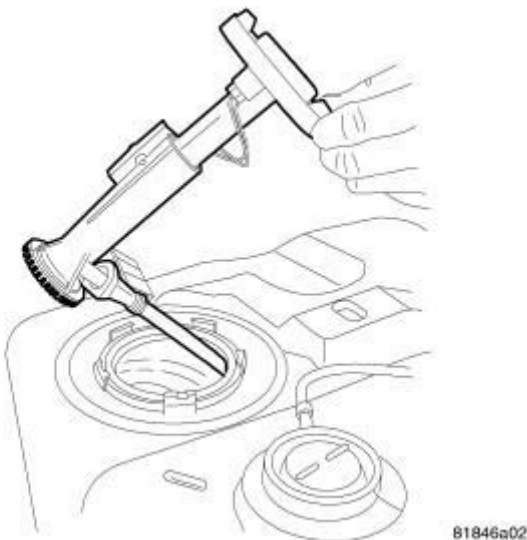
Fig. 170: Auxiliary Fuel Pump Module Internal Fuel Line Courtesy of CHRYSLER GROUP, LLC
