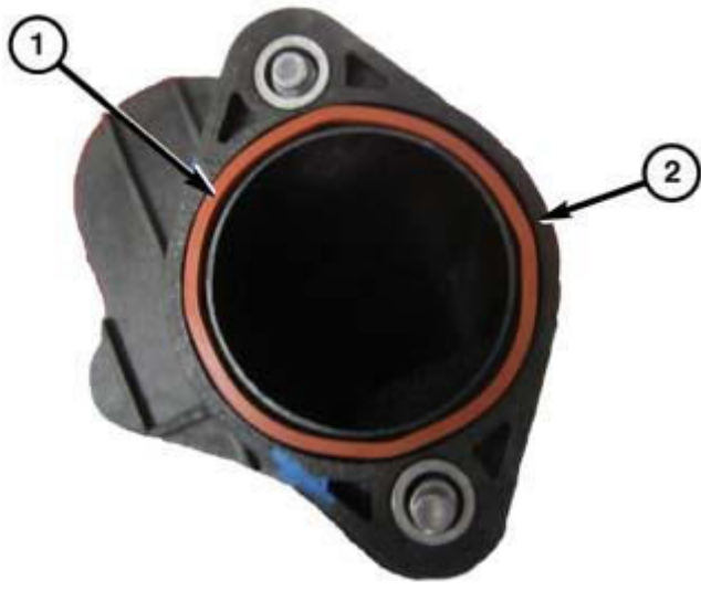
Fig. 354: CAC Tube & O-Ring Seal Courtesy of CHRYSLER GROUP, LLC
