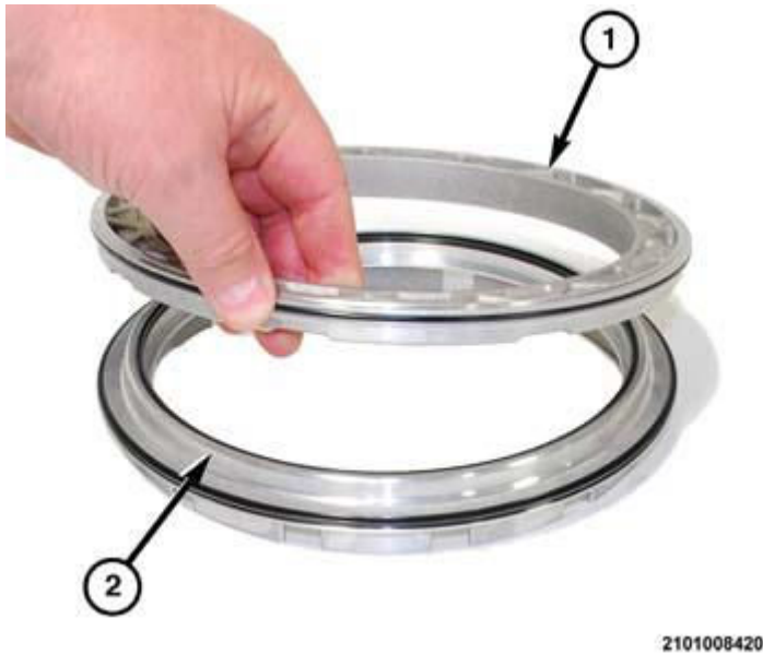
Fig. 96: D-Clutch Piston & Retainer Courtesy of CHRYSLER GROUP, LLC
