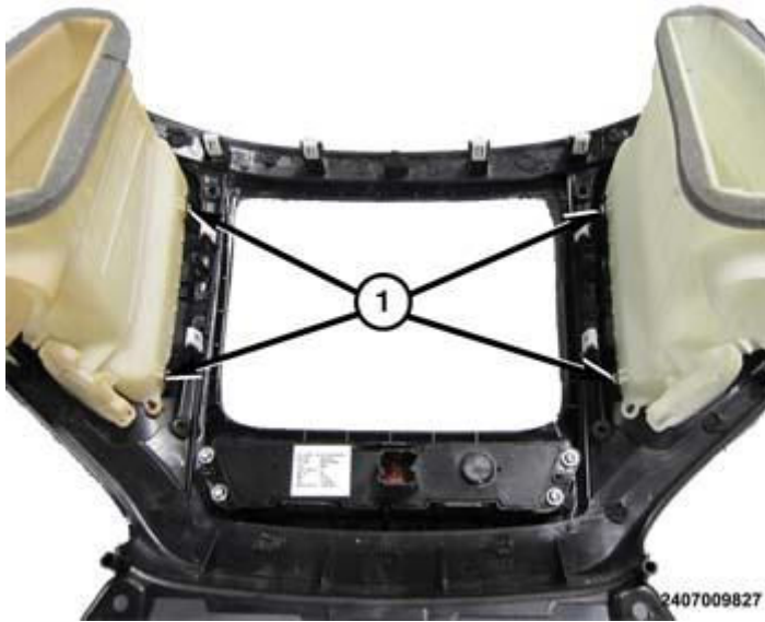
Fig. 57: Center Bezel & Front Center Air Outlets Courtesy of CHRYSLER GROUP, LLC
