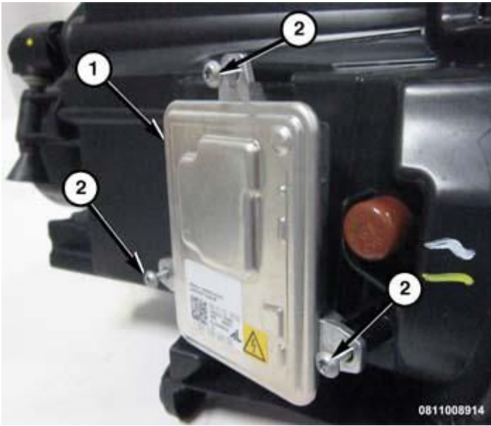
Fig. 5: Electronic Ballast Module & Screws Courtesy of CHRYSLER GROUP, LLC
