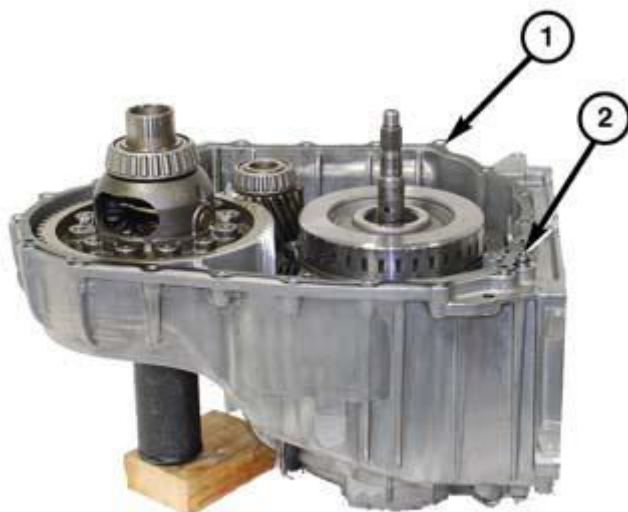
Fig. 344: Sealing Surface Of Transmission Housing Courtesy of CHRYSLER GROUP, LLC
