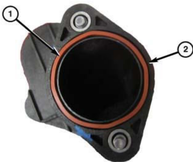
Fig. 369: CAC Tube & O-Ring Seal
