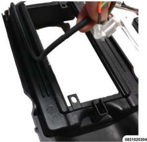
Fig. 29: Peeling Harness Out Of Channel Courtesy of CHRYSLER GROUP, LLC
