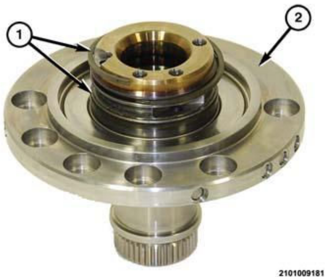
Fig. 673: Removing/Installing Seal Rings At Ring Land In Inner Reaction Shaft Hub Courtesy of CHRYSLER GROUP, LLC
