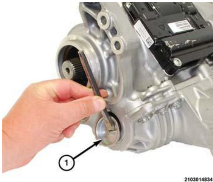
Fig. 45: Separating Plug From PTU Courtesy of CHRYSLER GROUP, LLC
