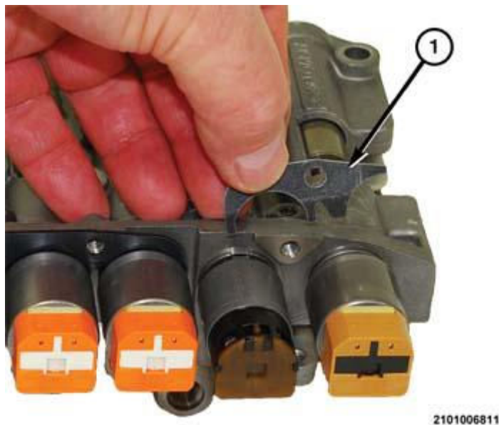
Fig. 737: View Of Solenoid Valve Small Retainer Courtesy of CHRYSLER GROUP, LLC
