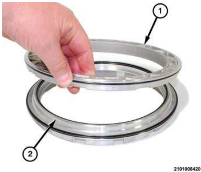
Fig. 153: D-Clutch Piston & Retainer Courtesy of CHRYSLER GROUP, LLC
