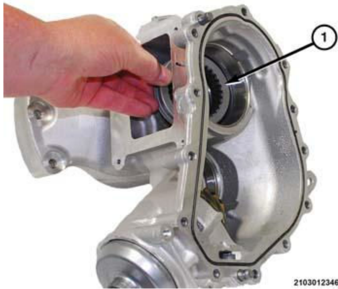
Fig. 20: Locating Dog Clutch Sleeve Courtesy of CHRYSLER GROUP, LLC
