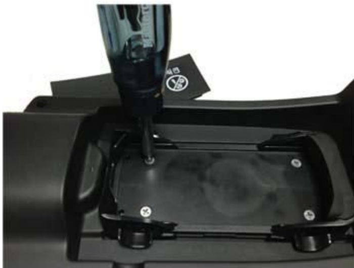
Fig. 40: Removing Screws Using A Phillips #2 Screwdriver Courtesy of CHRYSLER GROUP, LLC
