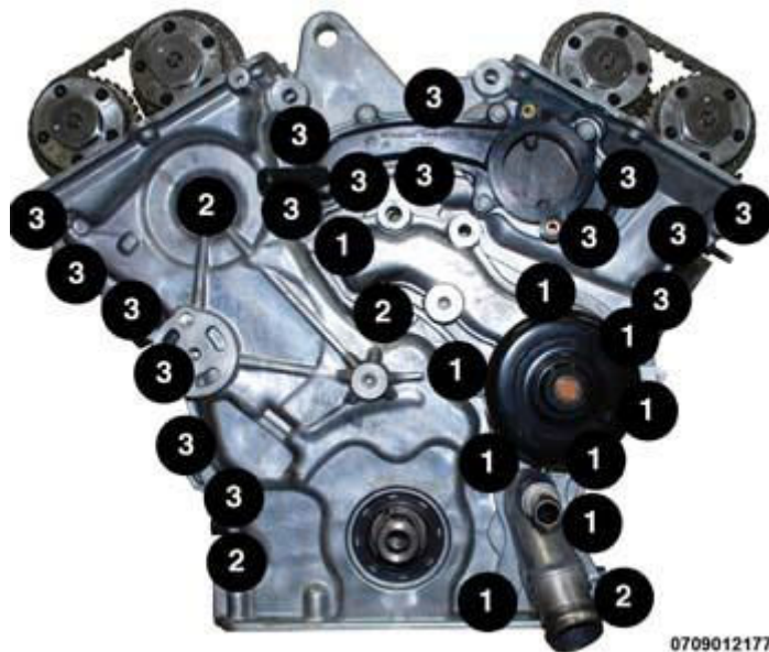
Fig. 621: Engine Timing Cover(s) Bolts Removing/Tightening Sequence Courtesy of CHRYSLER GROUP, LLC
