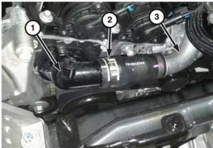
Fig. 604: Removing/Installing Thermostat Housing Courtesy of CHRYSLER GROUP, LLC
