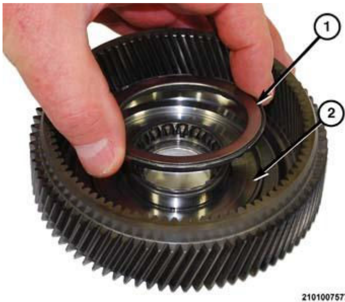
Fig. 87: Thrust Bearing & Annulus Gear 1 Planetary Hub Courtesy of CHRYSLER GROUP, LLC
