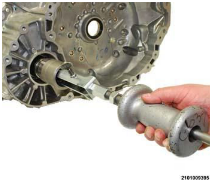
Fig. 507: Removing Differential Adapter Sleeve Courtesy of CHRYSLER GROUP, LLC
