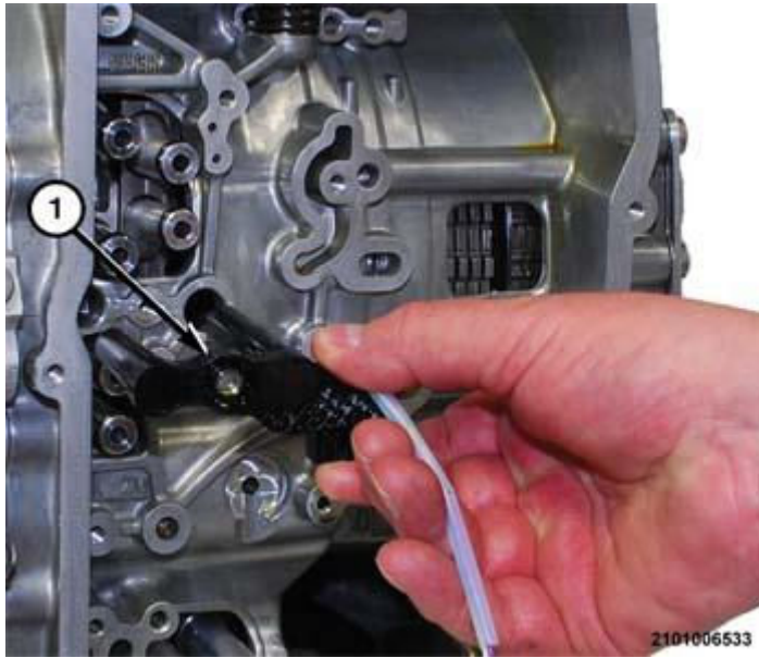
Fig. 378: Removing/Installing Speed Sensor Courtesy of CHRYSLER GROUP, LLC
