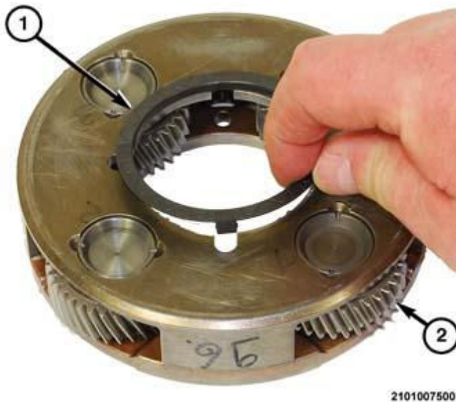
Fig. 165: Thrust Spacer & Underside Of Gear 4 Planetary Pinion Carrier Courtesy of CHRYSLER GROUP, LLC
