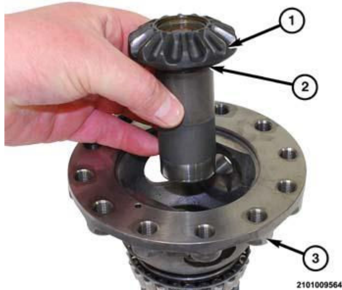
Fig. 550: Removing/Installing Differential Side Gear & Thrust Washer Courtesy of CHRYSLER GROUP, LLC
