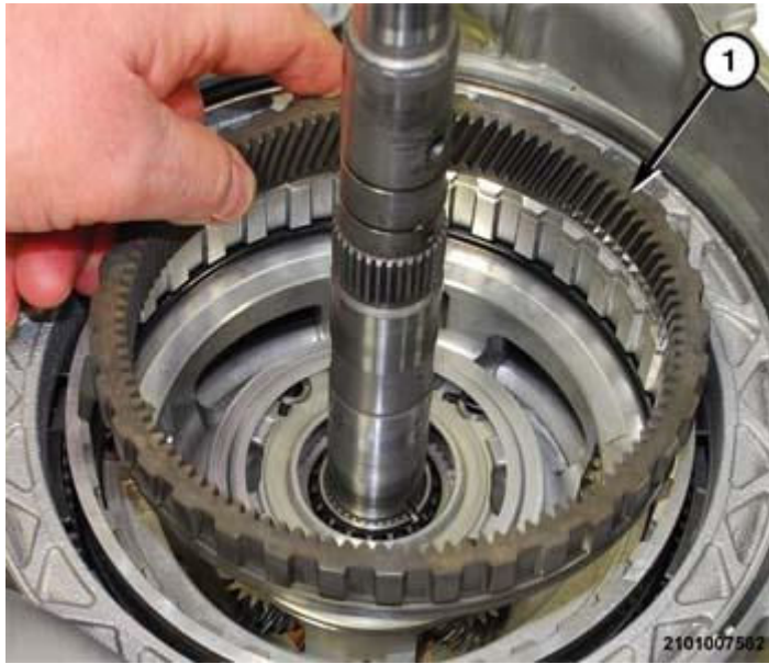
Fig. 90: Annulus Gear 3 & Carrier Gear 1&2 Courtesy of CHRYSLER GROUP, LLC
