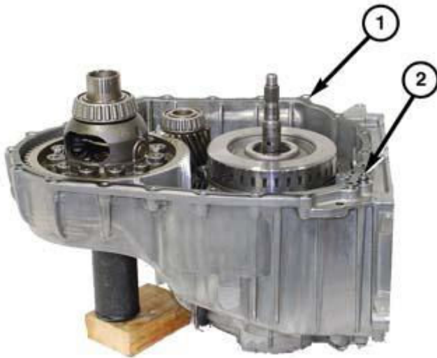
Fig. 179: Sealing Surface Of Transmission Housing Courtesy of CHRYSLER GROUP, LLC
