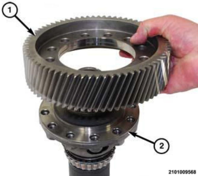
Fig. 487: View Of Ring Gear & Differential Unit Courtesy of CHRYSLER GROUP, LLC
