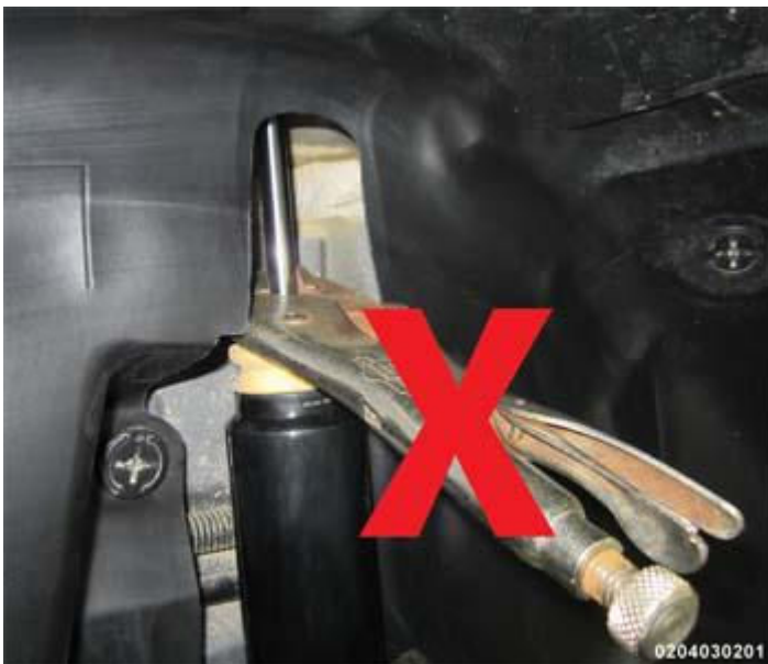
Fig. 25: Identifying Pliers On Chrome Machined Surface Of Shock/Strut Rod
