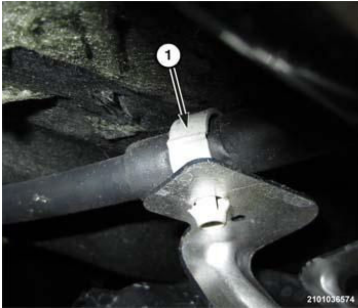
Fig. 262: Shifter Cable Clip Courtesy of CHRYSLER GROUP, LLC
