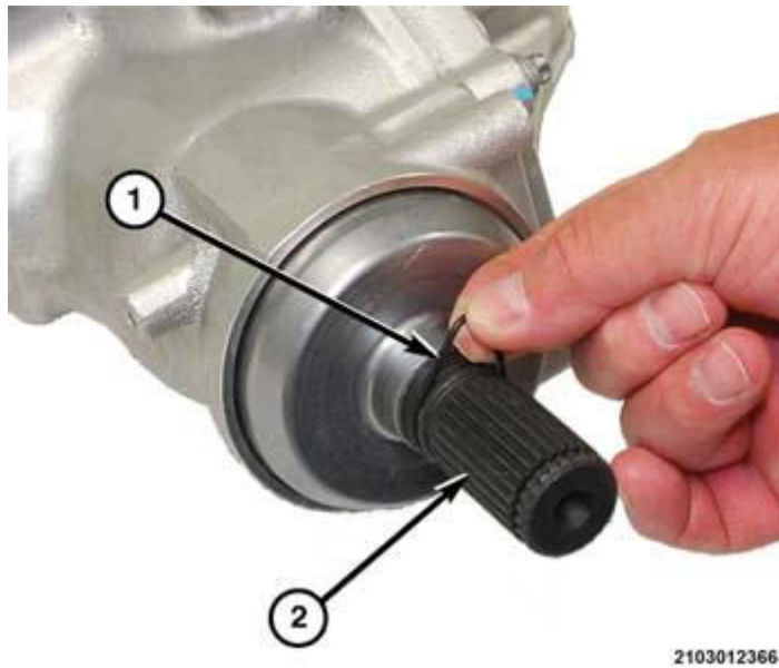
Fig. 52: Removing/Installing O-Ring At Rear Output Shaft Courtesy of CHRYSLER GROUP, LLC
