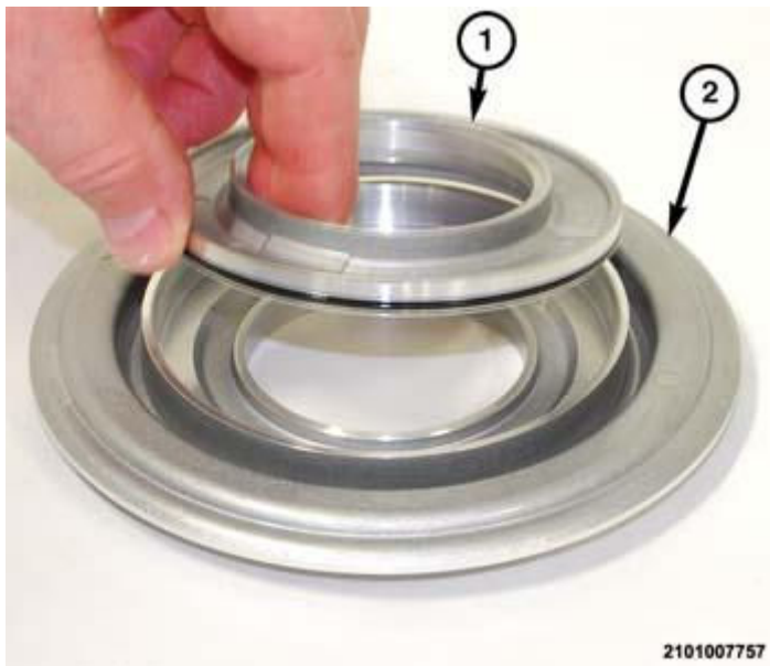
Fig. 422: Remove/Install Balance Piston At B-Clutch Piston Courtesy of CHRYSLER GROUP, LLC
