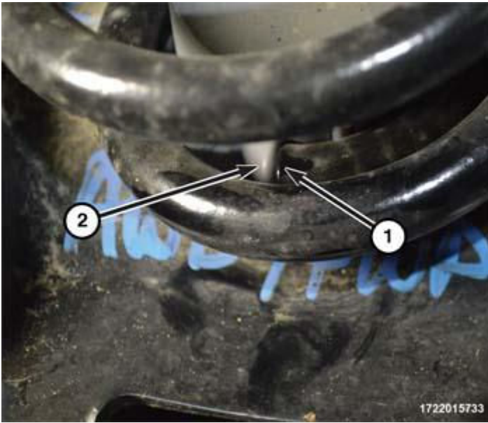
Fig. 52: Identifying Lower End Of Spring & Spring Isolator Courtesy of CHRYSLER GROUP, LLC
