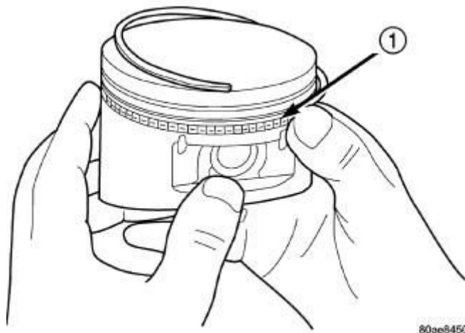
Fig. 259: Removing/Installing Piston Ring Side Rail Courtesy of CHRYSLER GROUP, LLC
