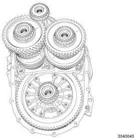
Fig. 4: Three Gear Shafts In Bellhousing Courtesy of CHRYSLER GROUP, LLC
