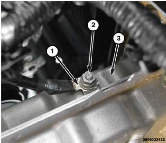
Fig. 31: Ground Wire, Nut & Right Side Upper Frame Courtesy of CHRYSLER GROUP, LLC
