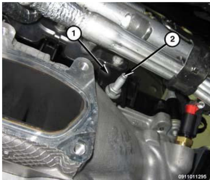
Fig. 214: Intake Manifold Left/Rearward Support Bracket & Stud Bolt Courtesy of CHRYSLER GROUP, LLC
