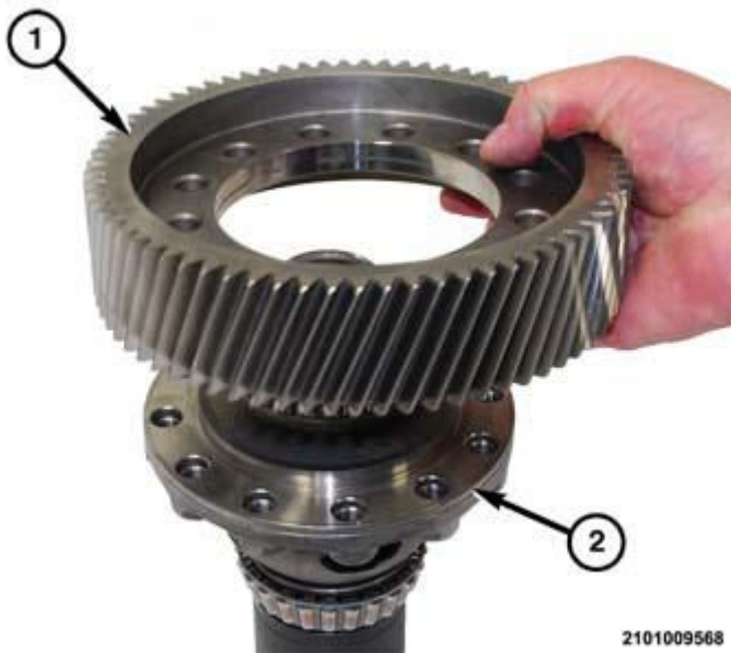
Fig. 558: View Of Ring Gear & Differential Unit Courtesy of CHRYSLER GROUP, LLC
