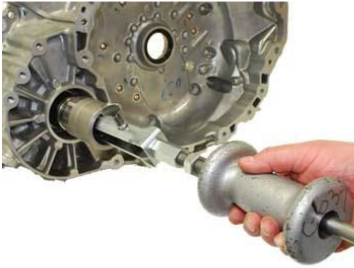
Fig. 496: Removing Differential Adapter Sleeve Courtesy of CHRYSLER GROUP, LLC
