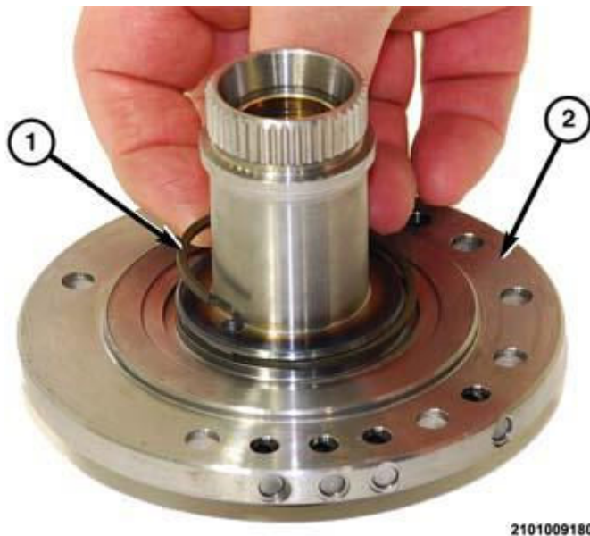
Fig. 674: Removing/Installing Seal Ring At Ring Land In Outer Reaction Shaft Hub Courtesy of CHRYSLER GROUP, LLC
