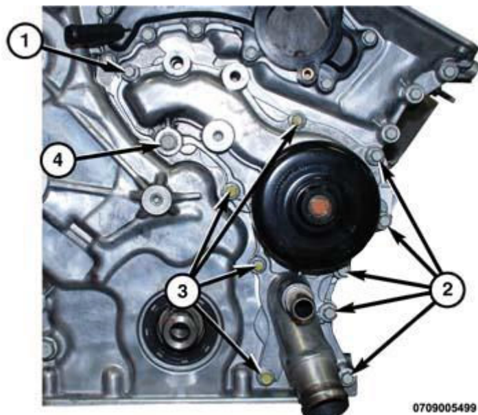
Fig. 612: Removing/Installing Water Pump Courtesy of CHRYSLER GROUP, LLC
