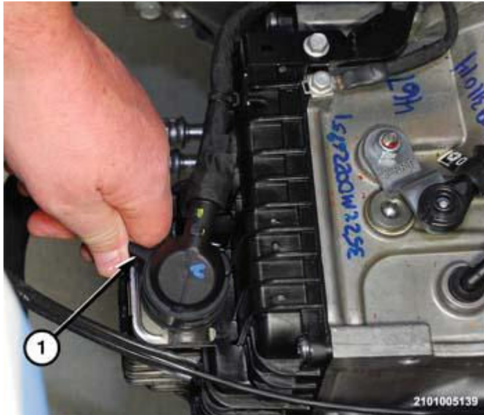
Fig. 221: Transmission Valve Body Solenoid Connector Courtesy of CHRYSLER GROUP, LLC
