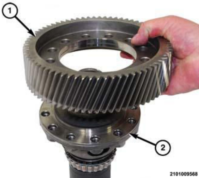
Fig. 534: View Of Ring Gear & Differential Unit Courtesy of CHRYSLER GROUP, LLC
