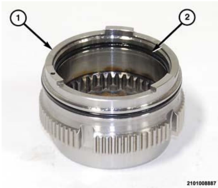
Fig. 471: Installing New Inner O-Ring Seal Into The Dog F-Clutch Piston Courtesy of CHRYSLER GROUP, LLC
