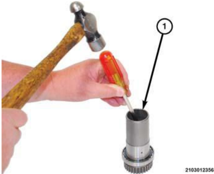
Fig. 16: Removing Seal(s) From Input Shaft Courtesy of CHRYSLER GROUP, LLC
