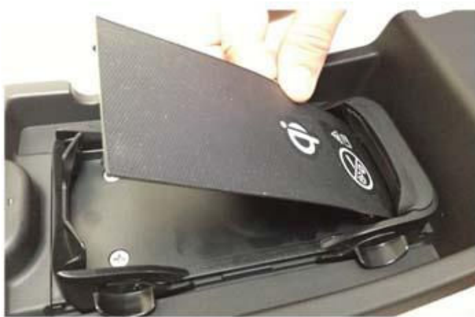
Fig. 42: Ensuring End Stops Are At Full Positions Courtesy of CHRYSLER GROUP, LLC
