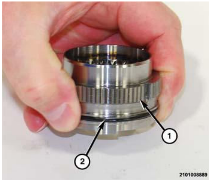
Fig. 472: Installing New Outer O-Ring Seal Into The Dog F-Clutch Piston Courtesy of CHRYSLER GROUP, LLC
