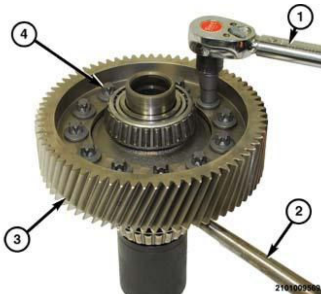
Fig. 547: Tightening Ring Gear Bolts Courtesy of CHRYSLER GROUP, LLC
