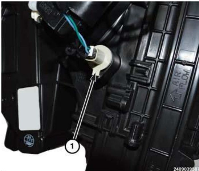
Fig. 29: Evaporator Temperature Sensor Location Courtesy of CHRYSLER GROUP, LLC
