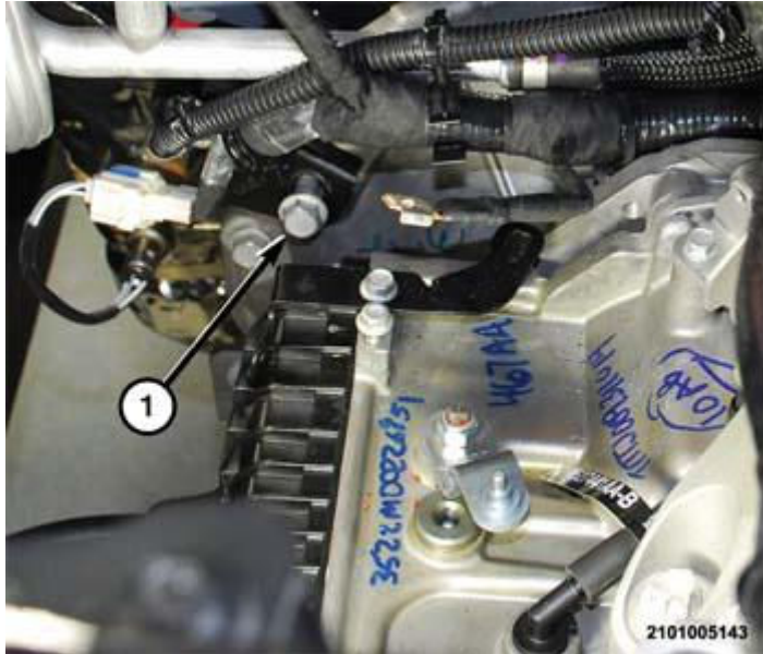
Fig. 48: Wire Harness Bracket & Bellhousing Bolt Courtesy of CHRYSLER GROUP, LLC
