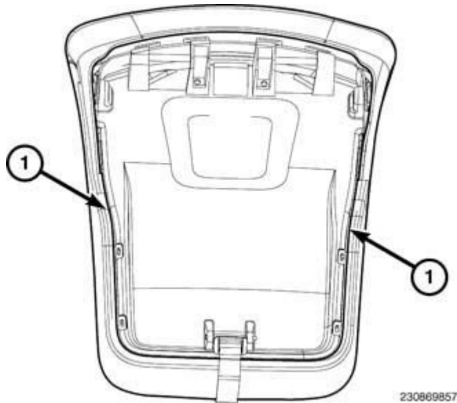
Fig. 593: Storage Bin Lid Cover Attachment Clips Courtesy of CHRYSLER GROUP, LLC
