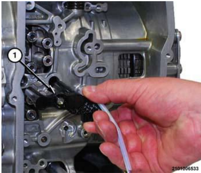
Fig. 309: Removing/Installing Speed Sensor Courtesy of CHRYSLER GROUP, LLC
