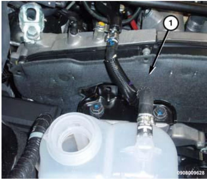
Fig. 231: Upper Timing Cover Insulator Courtesy of CHRYSLER GROUP, LLC
