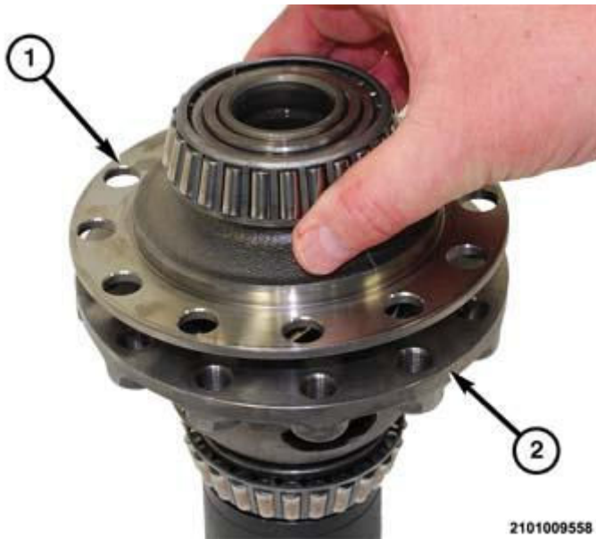
Fig. 544: View Of Upper Half Housing & Lower Differential Housing Courtesy of CHRYSLER GROUP, LLC
