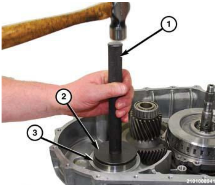
Fig. 296: Installing Bearing Race Courtesy of CHRYSLER GROUP, LLC
