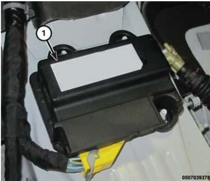
Fig. 1: Identifying Occupant Restraint Controller Courtesy of CHRYSLER GROUP, LLC
