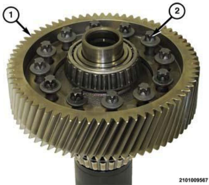
Fig. 486: View Of Ring Gear To Differential Unit & Bolts Courtesy of CHRYSLER GROUP, LLC
