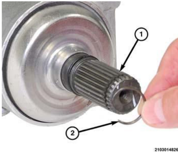
Fig. 55: Removing/Installing Circlip At Rear Output Shaft Courtesy of CHRYSLER GROUP, LLC
