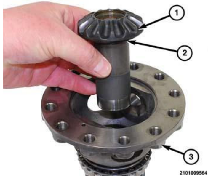
Fig. 525: Removing/Installing Differential Side Gear & Thrust Washer Courtesy of CHRYSLER GROUP, LLC
