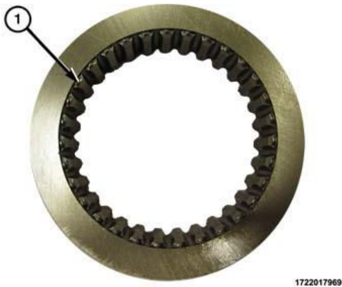
Fig. 21: Ensuring Proper Orientation Of Tapered Splines On Dog Clutch Sleeve Courtesy of CHRYSLER GROUP, LLC
