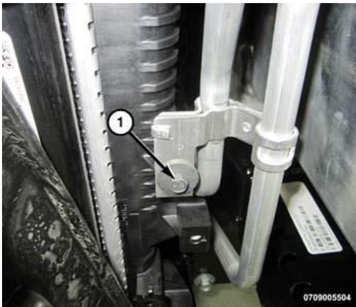
Fig. 79: Removing/Installing Transmission Cooler Line Support Bracket Bolt Courtesy of CHRYSLER GROUP, LLC
