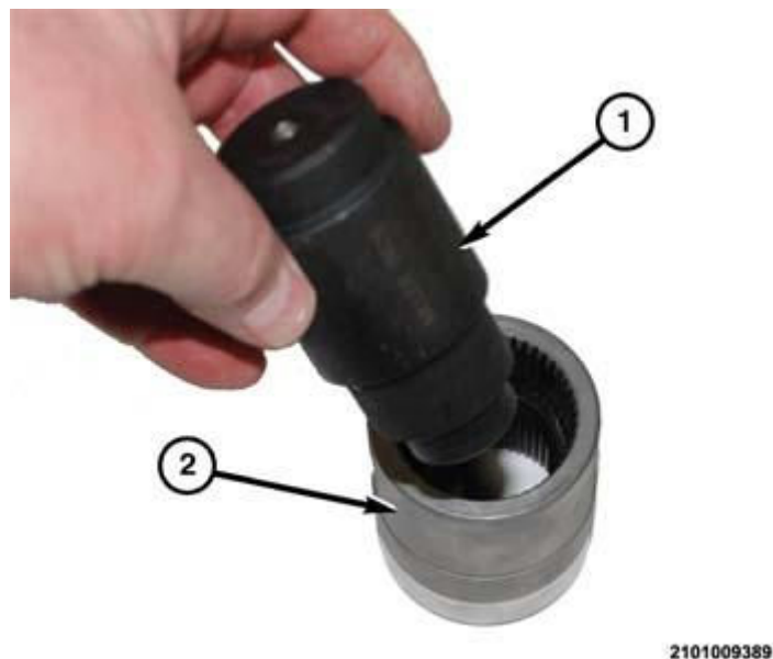
Fig. 649: PTU Side Of Adapter Sleeve And Special Tool Courtesy of CHRYSLER GROUP, LLC
