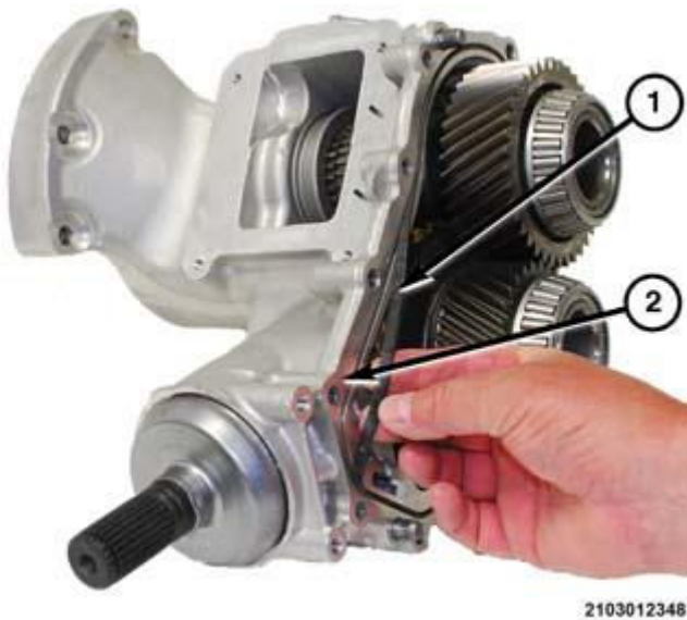
Fig. 23: PTU Housing & Gasket Courtesy of CHRYSLER GROUP, LLC
