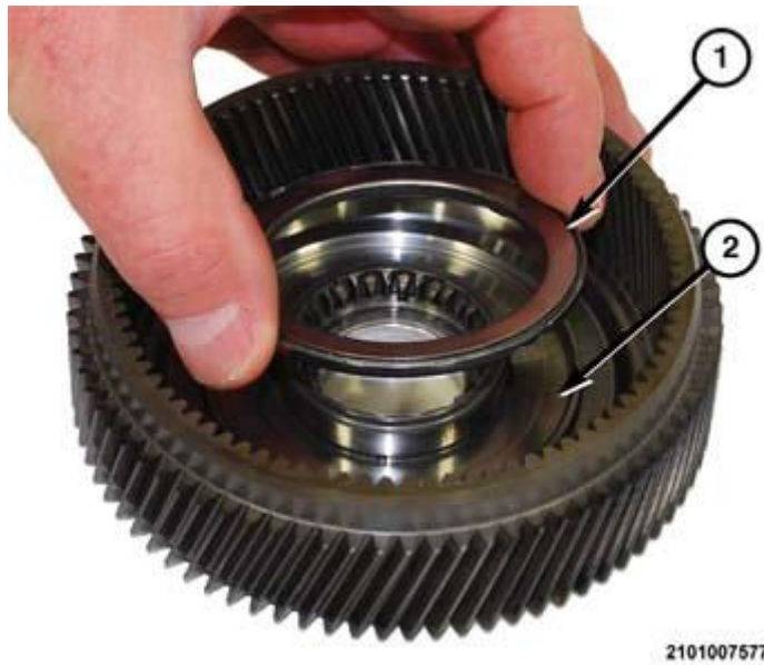
Fig. 160: Thrust Bearing & Annulus Gear 1 Planetary Hub Courtesy of CHRYSLER GROUP, LLC
