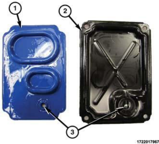
Fig. 61: Identifying Diaphragm Gasket And Hydraulic Fluid Cover Courtesy of CHRYSLER GROUP, LLC
