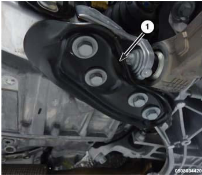
Fig. 73: Identifying Lower Load Beam Bracket Courtesy of CHRYSLER GROUP, LLC
