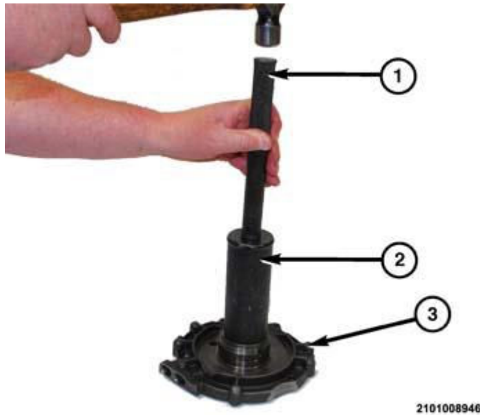
Fig. 480: Installing Dog F-Clutch Thrust Plate Into Output Gear Support Hub Courtesy of CHRYSLER GROUP, LLC
