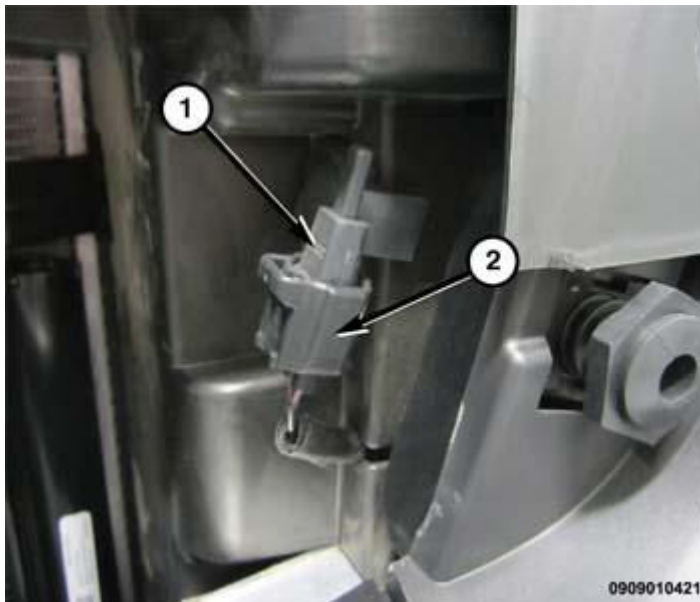
Fig. 165: Ambient Air Temperature Sensor & Wire Harness Connector Courtesy of CHRYSLER GROUP, LLC
