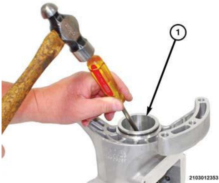
Fig. 15: Removing Seal(s) From PTU Housing Courtesy of CHRYSLER GROUP, LLC
