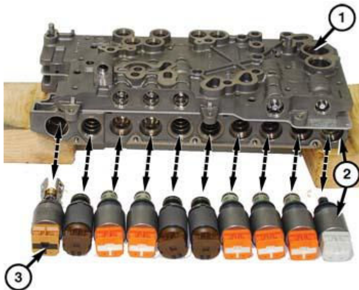
Fig. 731: Solenoid Valves & Outer Valve Body Courtesy of CHRYSLER GROUP, LLC
