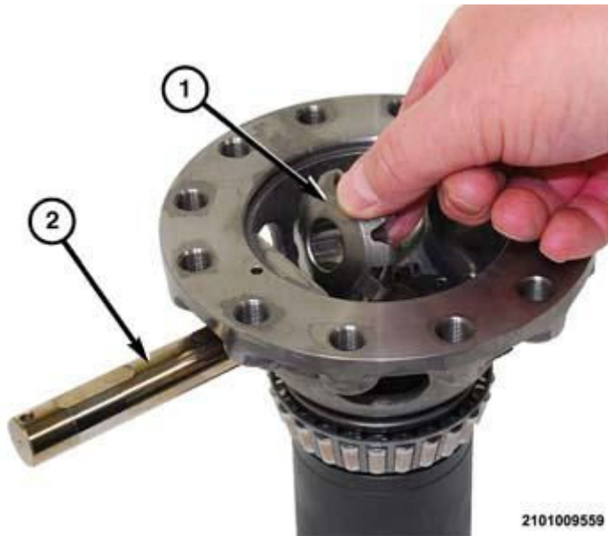
Fig. 528: Removing/Installing Pinion Shaft & Pinion Gear 2 Courtesy of CHRYSLER GROUP, LLC
