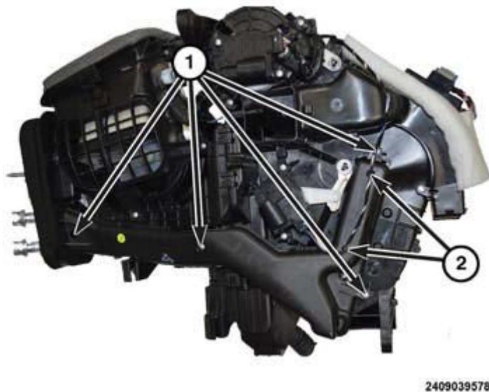
Fig. 125: Removing/Installing Heater Core Tubing Cover Courtesy of CHRYSLER GROUP, LLC
