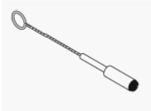
Fig. 282: Special Tool #9717 Injector Bore Brush Courtesy of CHRYSLER GROUP, LLC
