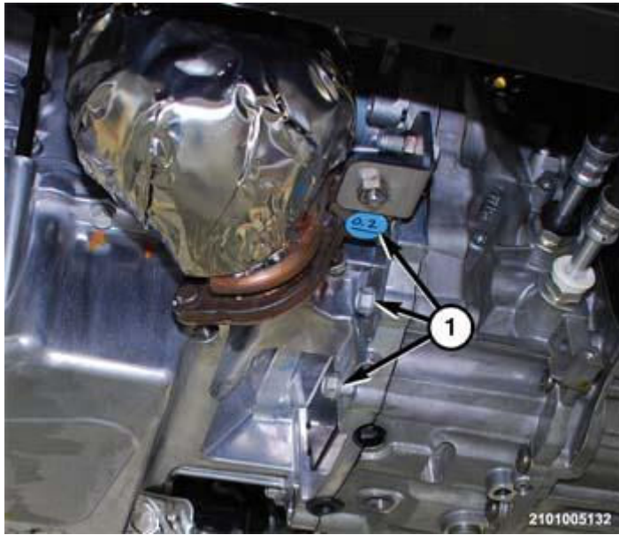
Fig. 226: Removing/Installing Transmission Bellhousing Bolts Courtesy of CHRYSLER GROUP, LLC
