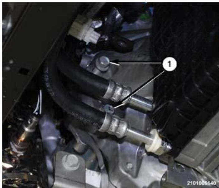
Fig. 212: Starter Bolts (3.2L) Courtesy of CHRYSLER GROUP, LLC
