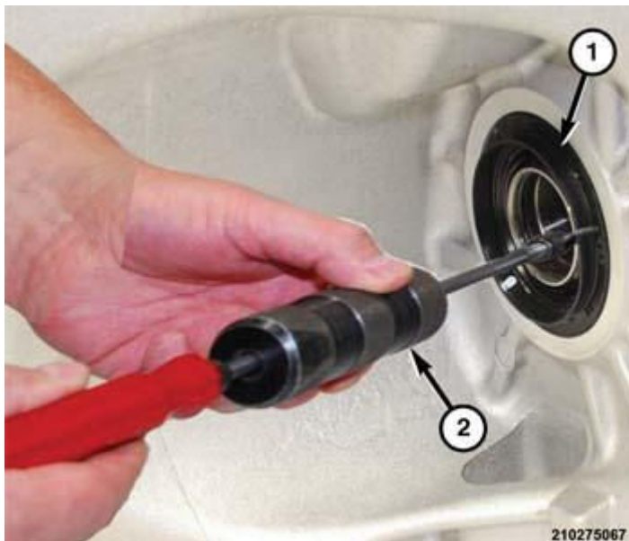
Fig. 640: Slide Hammer & Differential Seal Courtesy of CHRYSLER GROUP, LLC
