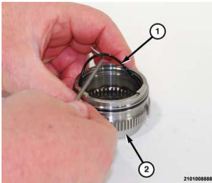
Fig. 468: Dog F-Clutch Piston & Inner O-Ring Seal Courtesy of CHRYSLER GROUP, LLC
