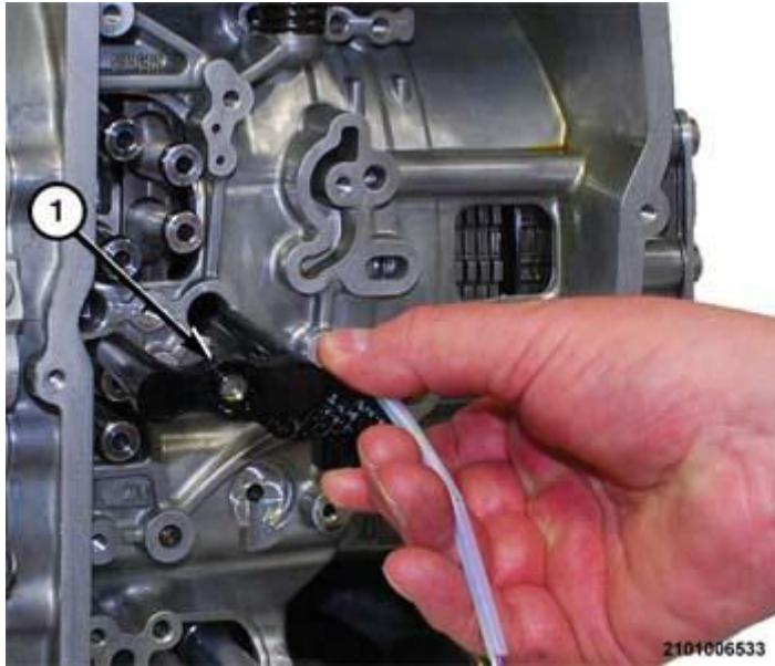
Fig. 665: Removing/Installing Speed Sensor Courtesy of CHRYSLER GROUP, LLC
