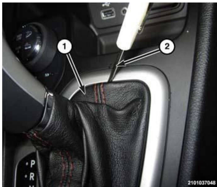
Fig. 740: Removing Shifter Bezel And Boot Assembly Courtesy of CHRYSLER GROUP, LLC
