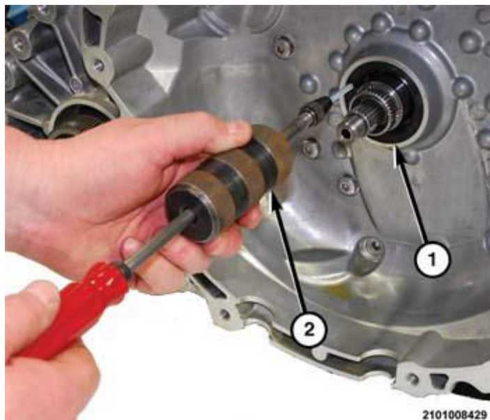
Fig. 661: Removing Seal From Center Of Bellhousing Courtesy of CHRYSLER GROUP, LLC
