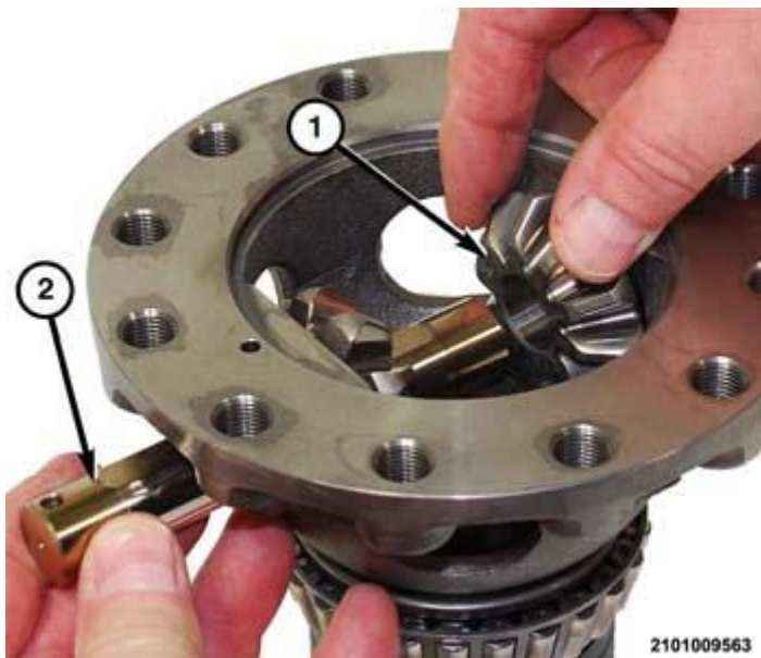
Fig. 492: Removing/Installing Pinion Gear 1 Courtesy of CHRYSLER GROUP, LLC
