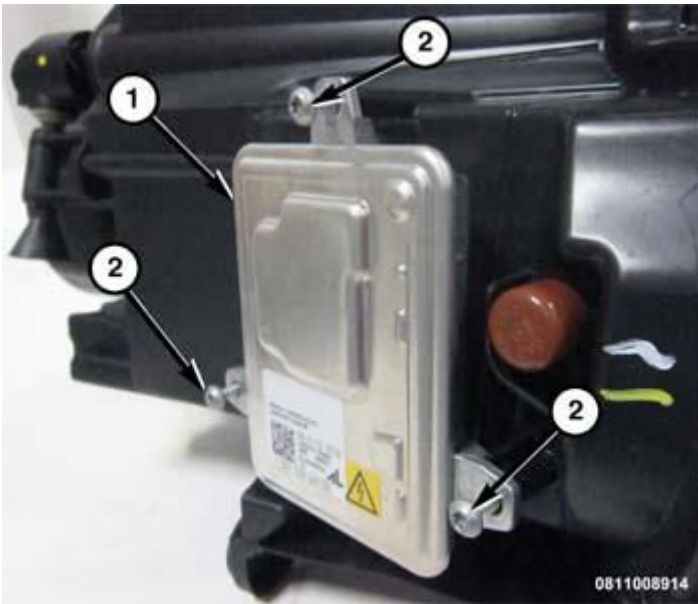
Fig. 4: Electronic Ballast Module & Screws Courtesy of CHRYSLER GROUP, LLC
