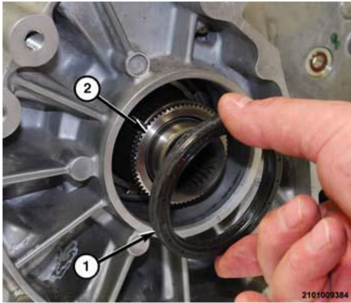
Fig. 655: Inserting Lip Seal Into Transmission Courtesy of CHRYSLER GROUP, LLC
