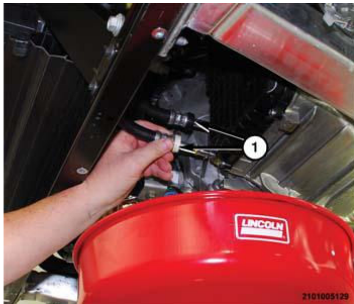
Fig. 234: Transmission Cooler Lines Courtesy of CHRYSLER GROUP, LLC
