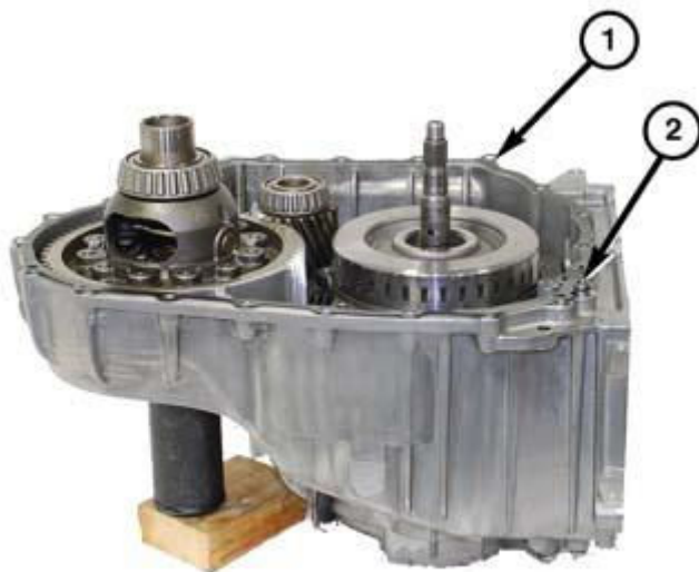
Fig. 384: Sealing Surface Of Transmission Housing Courtesy of CHRYSLER GROUP, LLC
