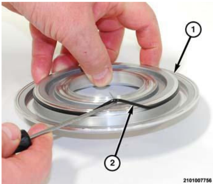
Fig. 419: Removing B-Clutch Piston O-Ring Courtesy of CHRYSLER GROUP, LLC
