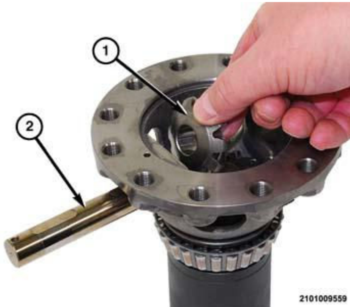
Fig. 552: Removing/Installing Pinion Shaft & Pinion Gear 2 Courtesy of CHRYSLER GROUP, LLC
