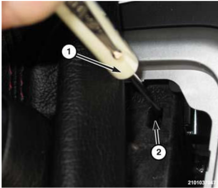
Fig. 741: Holding The Override Release Lever Down Courtesy of CHRYSLER GROUP, LLC
