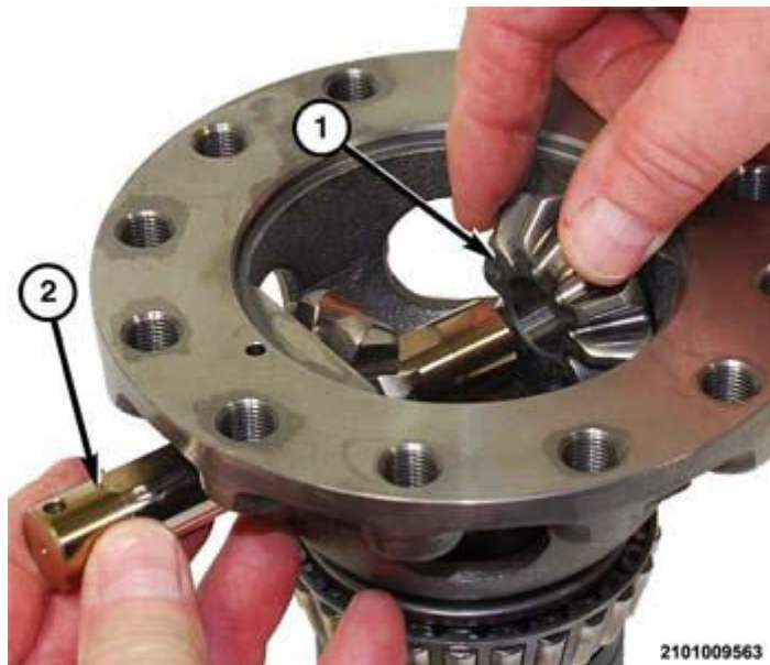
Fig. 529: Removing/Installing Pinion Gear 1 Courtesy of CHRYSLER GROUP, LLC
