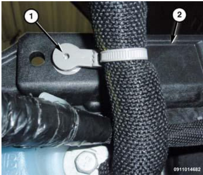
Fig. 42: Battery Tray & Engine Wire Harness Retainer Courtesy of CHRYSLER GROUP, LLC
