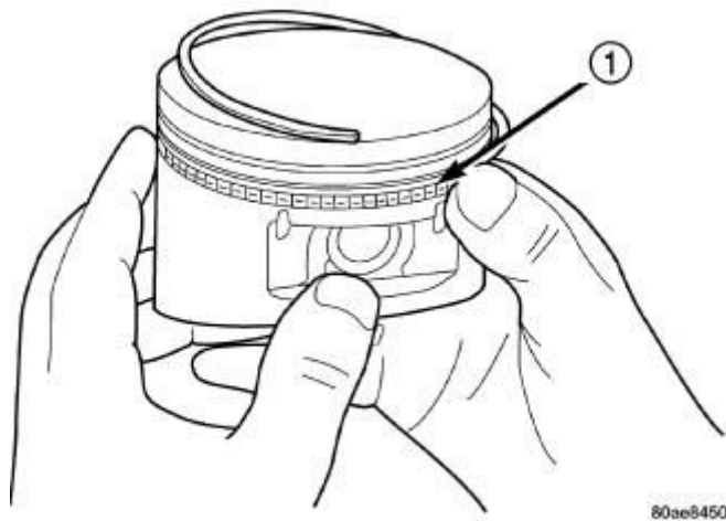
Fig. 257: Removing/Installing Piston Ring Side Rail Courtesy of CHRYSLER GROUP, LLC
