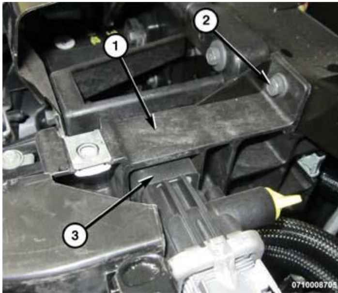
Fig. 81: Removing/Installing Upper Radiator Mounts Courtesy of CHRYSLER GROUP, LLC
