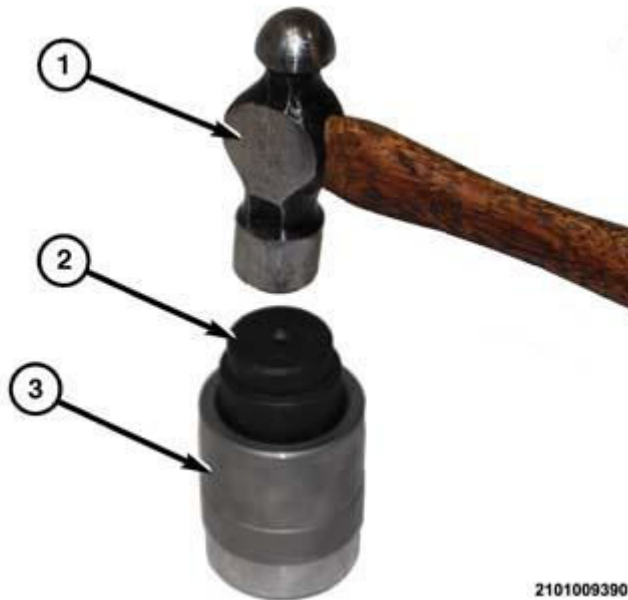
Fig. 650: Removing Seal From Inside Of Adapter Sleeve Courtesy of CHRYSLER GROUP, LLC
