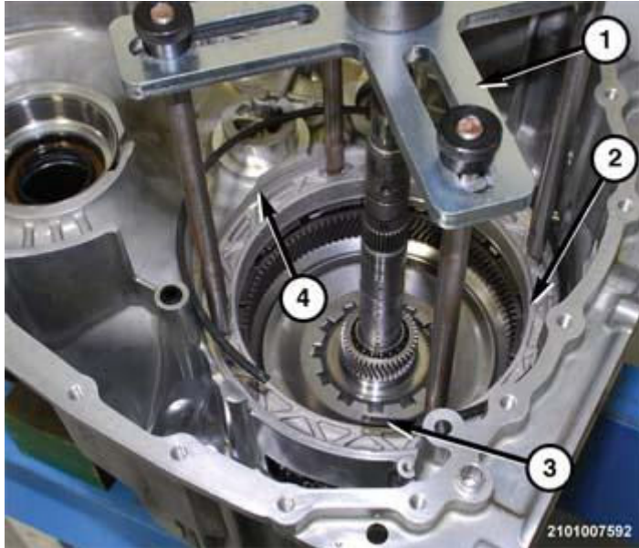
Fig. 93: Gaining Access To Snap Ring-Ring & Groove Courtesy of CHRYSLER GROUP, LLC
