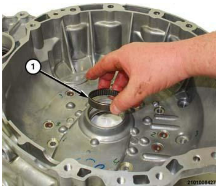
Fig. 593: Installing Oil Pump Sprocket Needle Bearing Into Bellhousing
