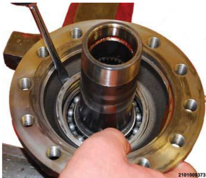
Fig. 501: Removing Snap-Ring Courtesy of CHRYSLER GROUP, LLC
