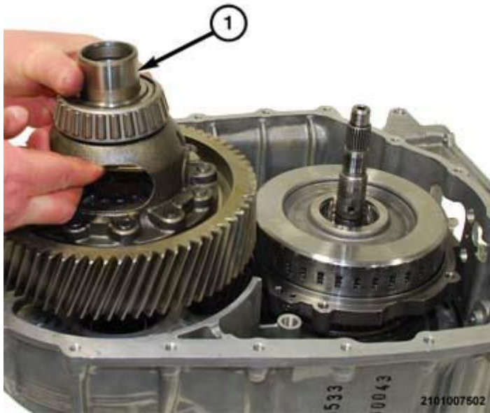
Fig. 537: Removing/Installing Differential Assembly Courtesy of CHRYSLER GROUP, LLC
