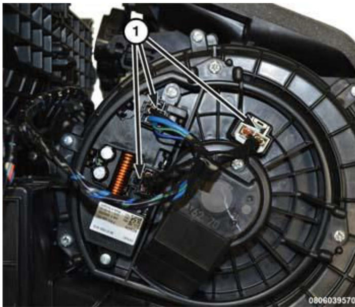
Fig. 20: Blower Motor Power Module And Blower Motor Wiring Harness Connectors Courtesy of CHRYSLER GROUP, LLC
