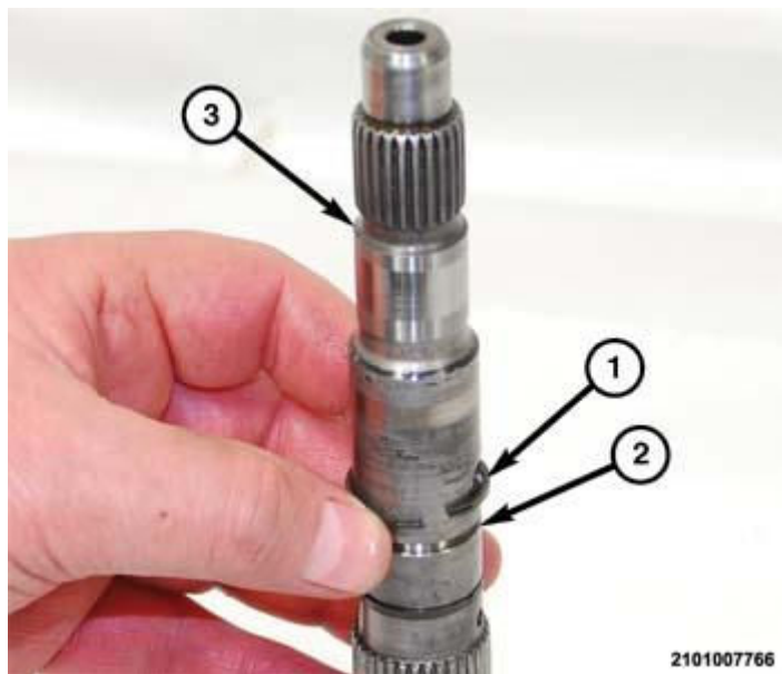
Fig. 145: Remove/Install Input Shaft Seal-Rings Courtesy of CHRYSLER GROUP, LLC
