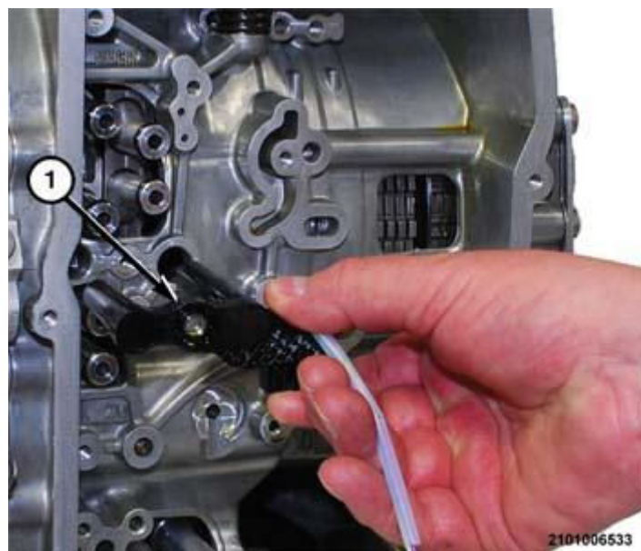
Fig. 391: Removing/Installing Speed Sensor Courtesy of CHRYSLER GROUP, LLC
