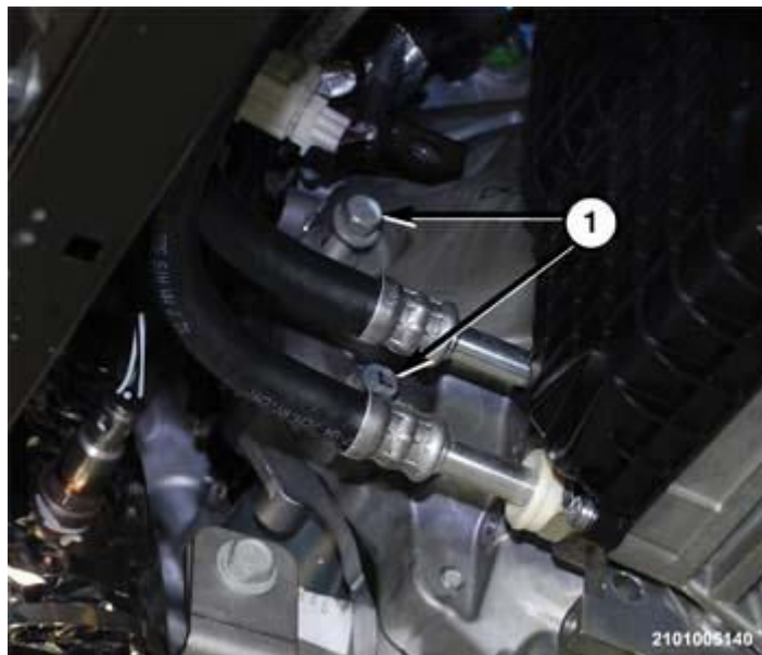
Fig. 231: Starter Bolts (3.2L) Courtesy of CHRYSLER GROUP, LLC
