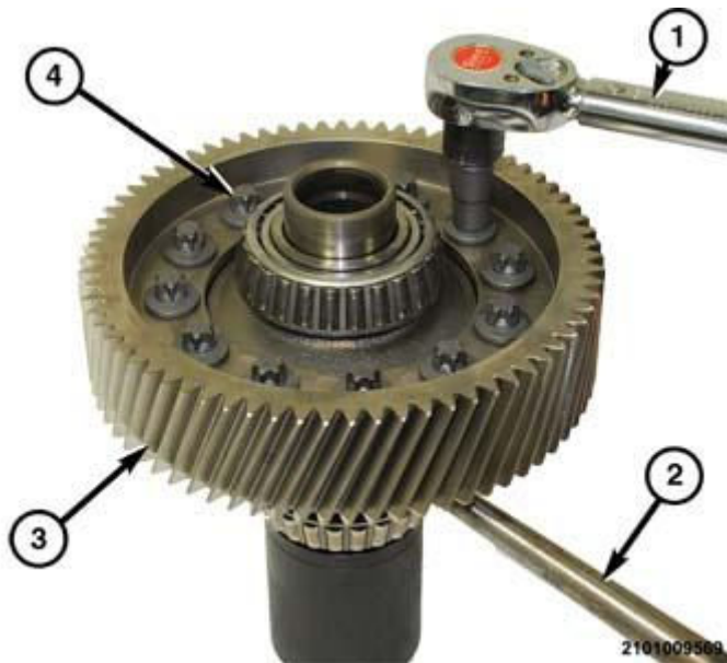
Fig. 560: Tightening Ring Gear Bolts Courtesy of CHRYSLER GROUP, LLC
