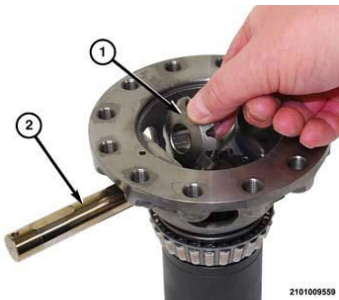
Fig. 516: Removing/Installing Pinion Shaft & Pinion Gear 2 Courtesy of CHRYSLER GROUP, LLC
