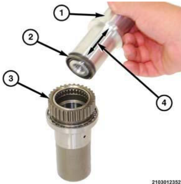
Fig. 17: Installing Outer Seal In Input Gear Courtesy of CHRYSLER GROUP, LLC
