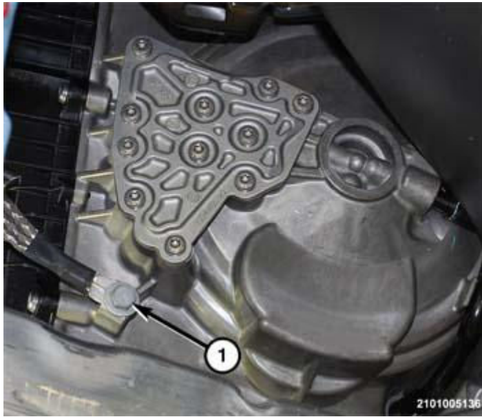
Fig. 23: Transmission End Cover Ground Cable Courtesy of CHRYSLER GROUP, LLC
