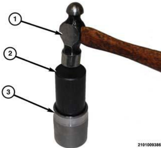
Fig. 658: Installing Seal Into Adapter Sleeve Courtesy of CHRYSLER GROUP, LLC
