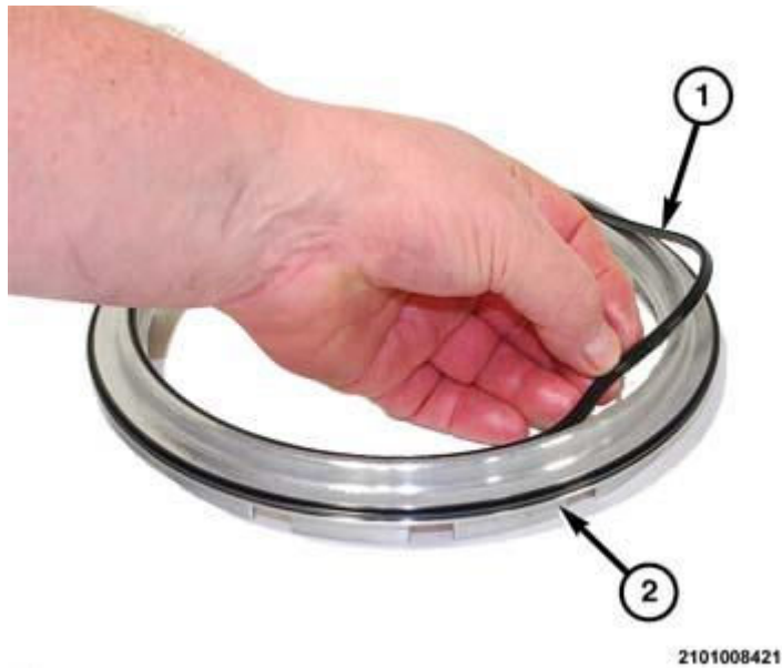
Fig. 152: D-Clutch Piston & Inner Lip Seal Ring Courtesy of CHRYSLER GROUP, LLC
