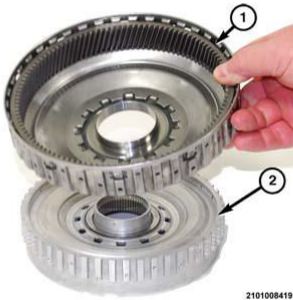
Fig. 106: Annulus Gear 2, D-Clutch Hub & C-Clutch Hub Courtesy of CHRYSLER GROUP, LLC
