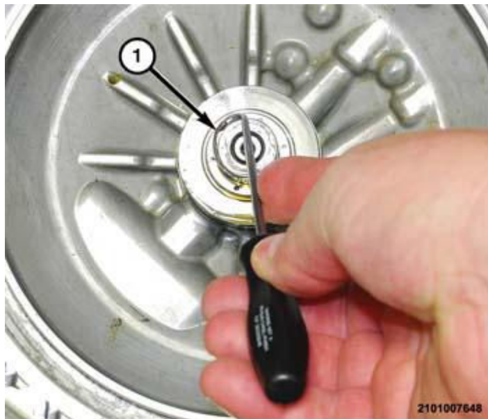
Fig. 124: Removing/Installing Inner Seal-Rings Courtesy of CHRYSLER GROUP, LLC
