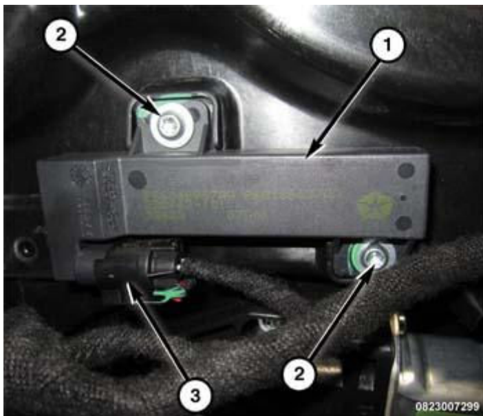
Fig. 8: Antenna, Connector & Screws
