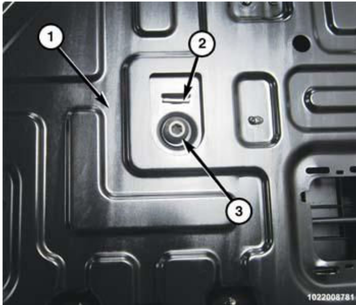
Fig. 89: Rear Center Seat Belt Retractor Fastener Courtesy of CHRYSLER GROUP, LLC
