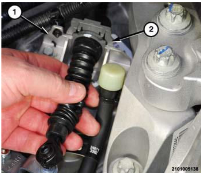
Fig. 222: View Of Shift Cable Housing & Mount Bracket Courtesy of CHRYSLER GROUP, LLC
