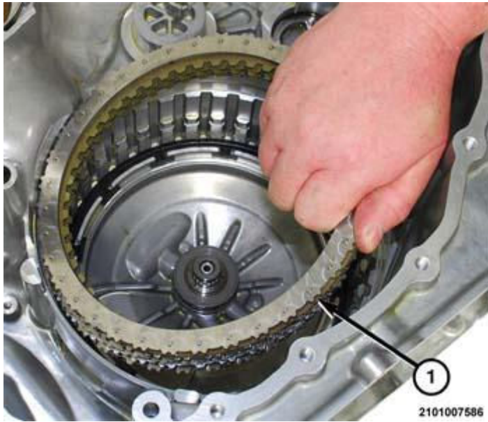
Fig. 112: Removing C-Clutch Friction Discs & Steel Plates From Transmission Housing Courtesy of CHRYSLER GROUP, LLC
