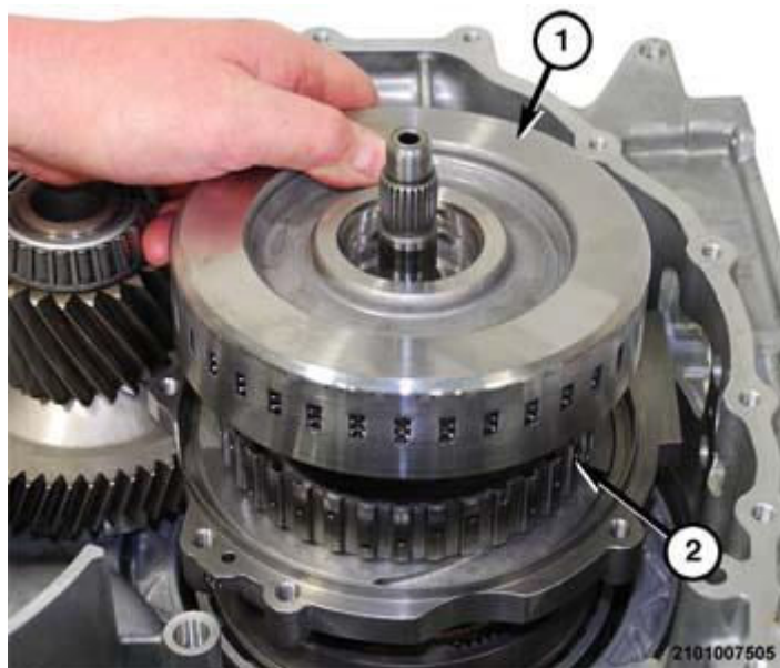
Fig. 317: Removing/Installing E-Clutch At E-Clutch Hub Courtesy of CHRYSLER GROUP, LLC
