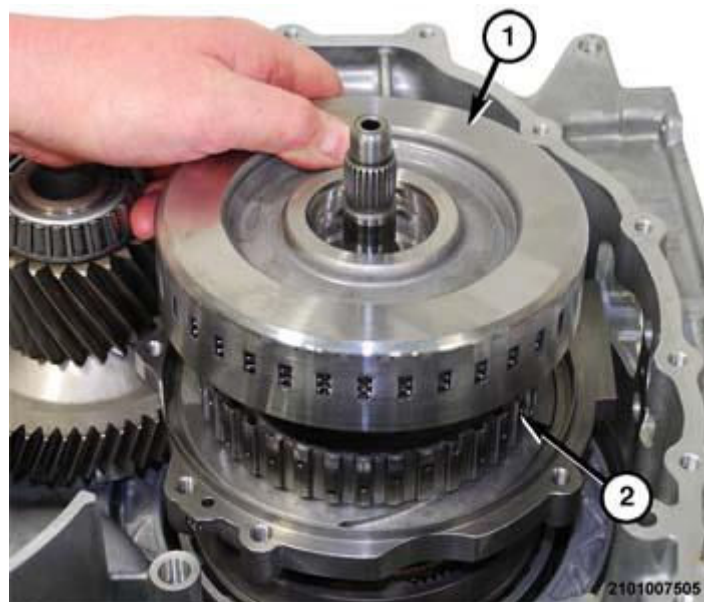
Fig. 341: Removing/Installing E-Clutch At E-Clutch Hub Courtesy of CHRYSLER GROUP, LLC
