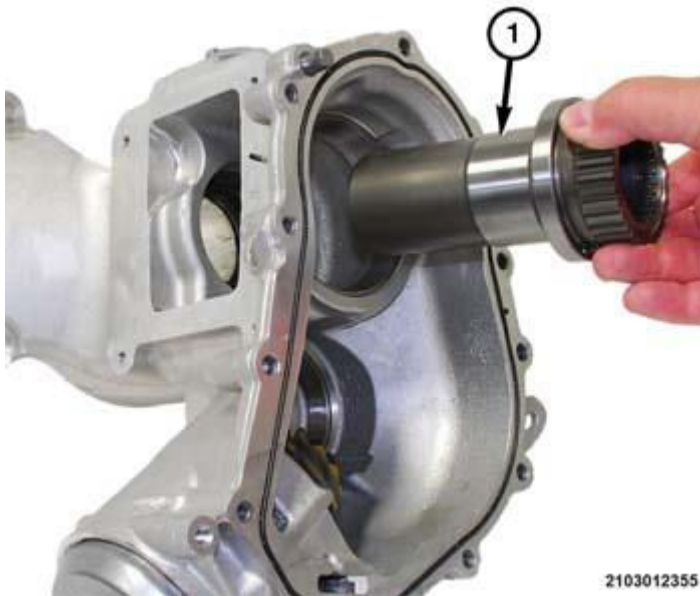
Fig. 14: Removing/Installing Input Shaft & Bearing At PTU Housing Courtesy of CHRYSLER GROUP, LLC
