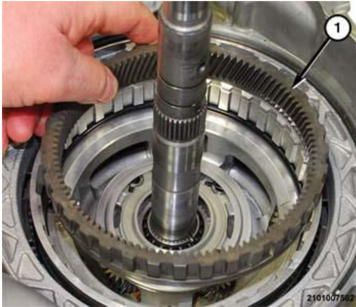
Fig. 158: Annulus Gear 3 & Carrier Gear 1&2 Courtesy of CHRYSLER GROUP, LLC
