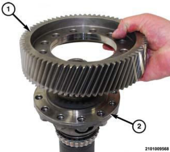
Fig. 510: View Of Ring Gear & Differential Unit Courtesy of CHRYSLER GROUP, LLC
