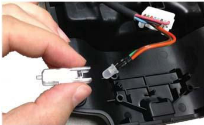
Fig. 28: Squeezing LED Lens Legs Courtesy of CHRYSLER GROUP, LLC
