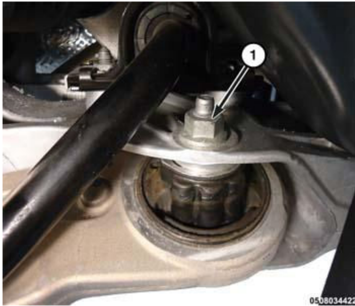
Fig. 4: Identifying Rear Lower Control Arm Nut Courtesy of CHRYSLER GROUP, LLC
