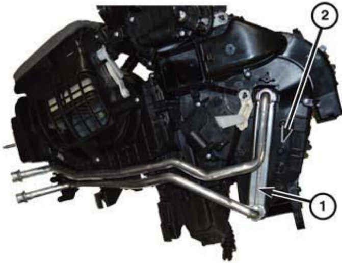
Fig. 127: Removing/Installing Heater Core Courtesy of CHRYSLER GROUP, LLC
