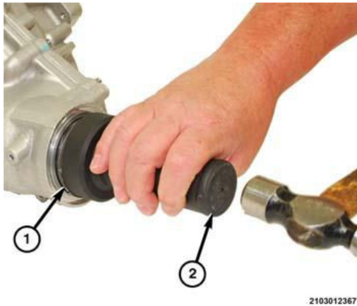
Fig. 60: Installing New Seal Into PTU Housing Courtesy of CHRYSLER GROUP, LLC
