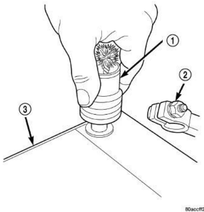
Fig. 3: Cleaning Battery Terminal Post Using Terminal Cleaner Courtesy of CHRYSLER GROUP, LLC
