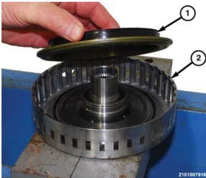
Fig. 450: E-Clutch Retainer & Piston Courtesy of CHRYSLER GROUP, LLC
