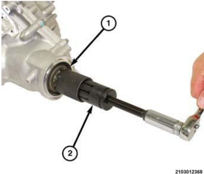
Fig. 54: Removing Seal From PTU Housing Courtesy of CHRYSLER GROUP, LLC
