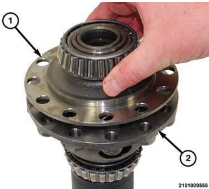
Fig. 533: View Of Upper Half Housing & Lower Differential Housing Courtesy of CHRYSLER GROUP, LLC
