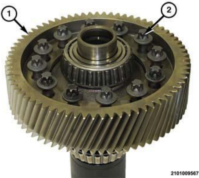
Fig. 535: View Of Ring Gear To Differential Unit & Bolts Courtesy of CHRYSLER GROUP, LLC
