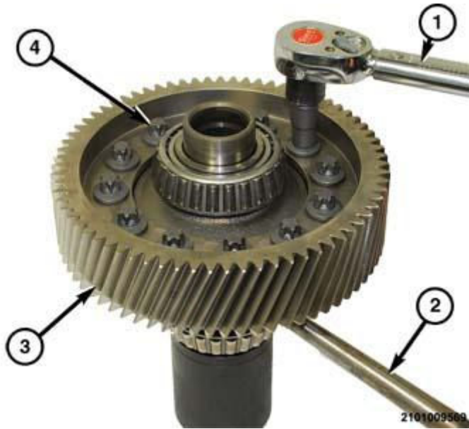
Fig. 536: Tightening Ring Gear Bolts Courtesy of CHRYSLER GROUP, LLC
