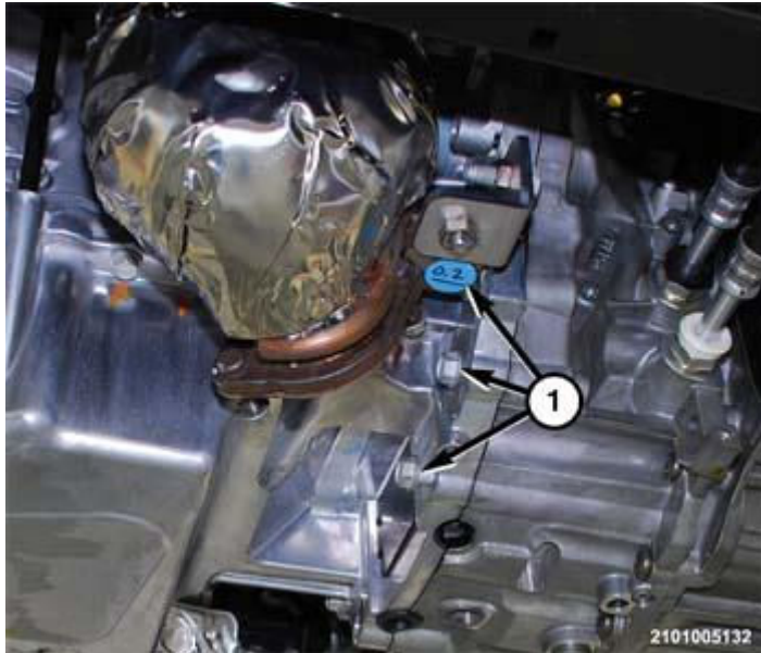
Fig. 58: Removing/Installing Transmission Bellhousing Bolts Courtesy of CHRYSLER GROUP, LLC
