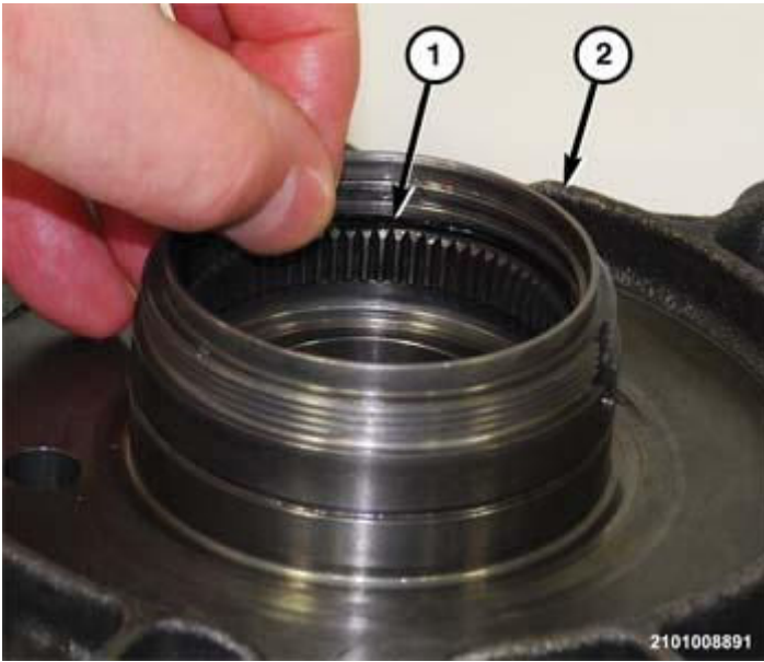
Fig. 470: Installing A New Upper O-Ring Seal To Inside Land Of Output Gear Support Hub Courtesy of CHRYSLER GROUP, LLC
