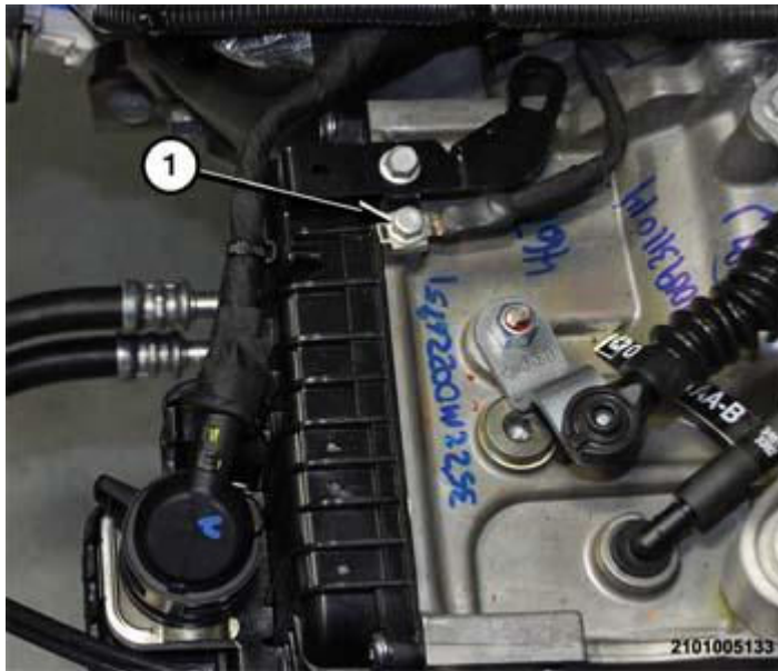
Fig. 244: Ground Cable At Top Transmission Courtesy of CHRYSLER GROUP, LLC
