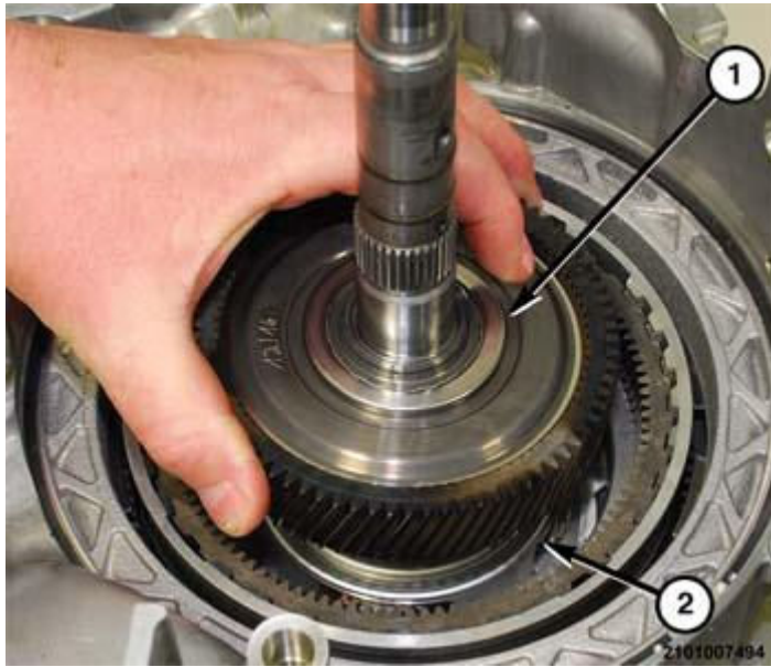
Fig. 86: Annulus Gear 1 Planetary Hub & Carrier Gear 1 And 2 Courtesy of CHRYSLER GROUP, LLC
