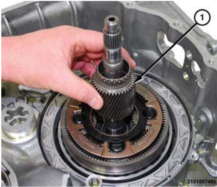
Fig. 168: Removing/Installing Sun Gear 3, 4 And Dog Clutch-F At Gear 4 Planetary Pinion Carrier Courtesy of CHRYSLER GROUP, LLC
