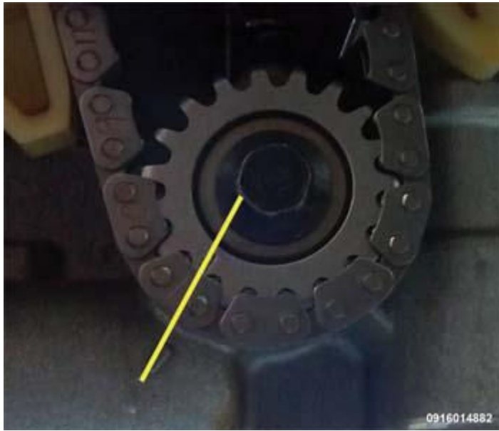
Fig. 375: Aligning Balance Shaft/Oil Pump Drive Gear And Housing Indicator Courtesy of CHRYSLER GROUP, LLC
