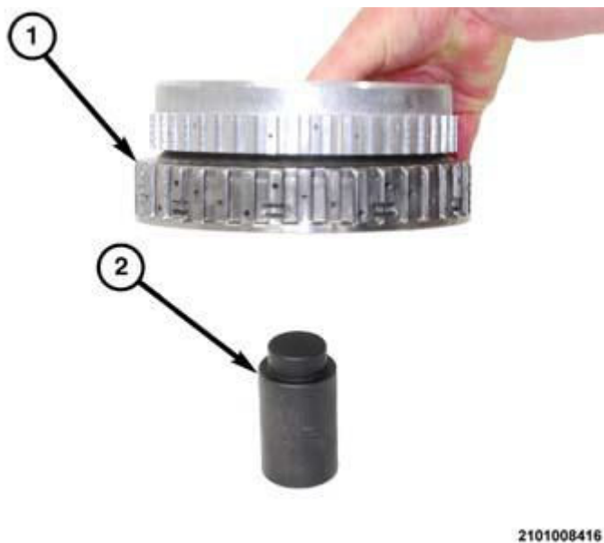
Fig. 143: Annulus Gear 2, D And C-Clutch Hub/B-Clutch Retainer Courtesy of CHRYSLER GROUP, LLC
