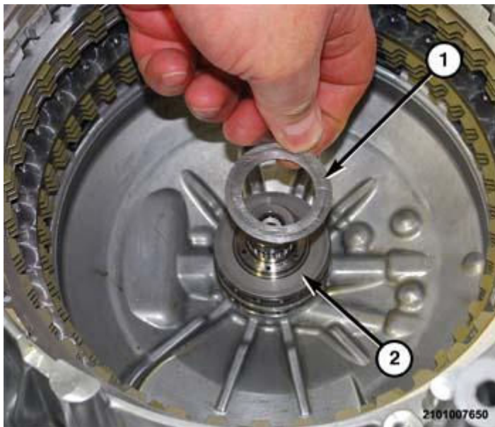
Fig. 109: Removing/Installing Input Shaft Rear Support Selective Thrust Washer Courtesy of CHRYSLER GROUP, LLC
