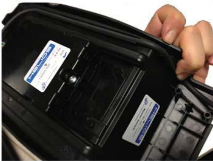
Fig. 39: Holding Down Harness In Channel Courtesy of CHRYSLER GROUP, LLC
