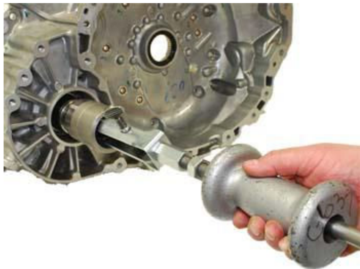
Fig. 646: Removing Differential Adapter Sleeve Courtesy of CHRYSLER GROUP, LLC
