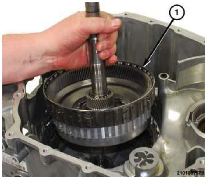
Fig. 100: Annulus Gear 2, D & C-Clutch Hub And Input Shaft Assembly Courtesy of CHRYSLER GROUP, LLC
