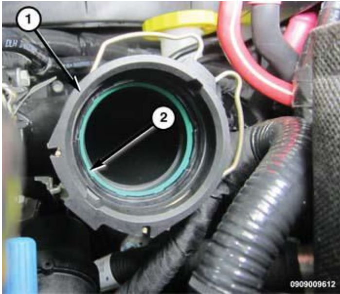
Fig. 51: O-Ring & EGR Air Flow Control Valve Inlet Tube Courtesy of CHRYSLER GROUP, LLC
