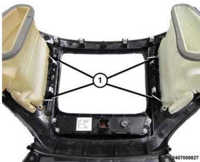
Fig. 58: Center Bezel & Front Center Air Outlets Courtesy of CHRYSLER GROUP, LLC
