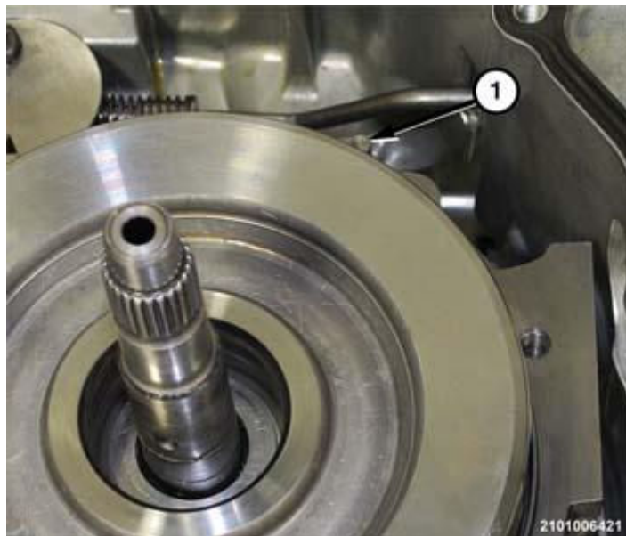
Fig. 347: Checking Guide Pin Alignment
