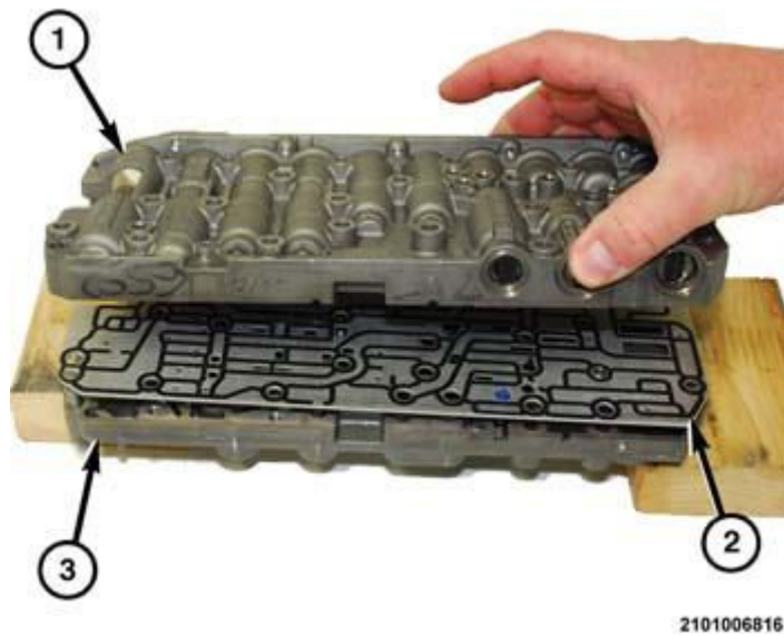
Fig. 713: Outer Valve Body & Separator Plate Courtesy of CHRYSLER GROUP, LLC
