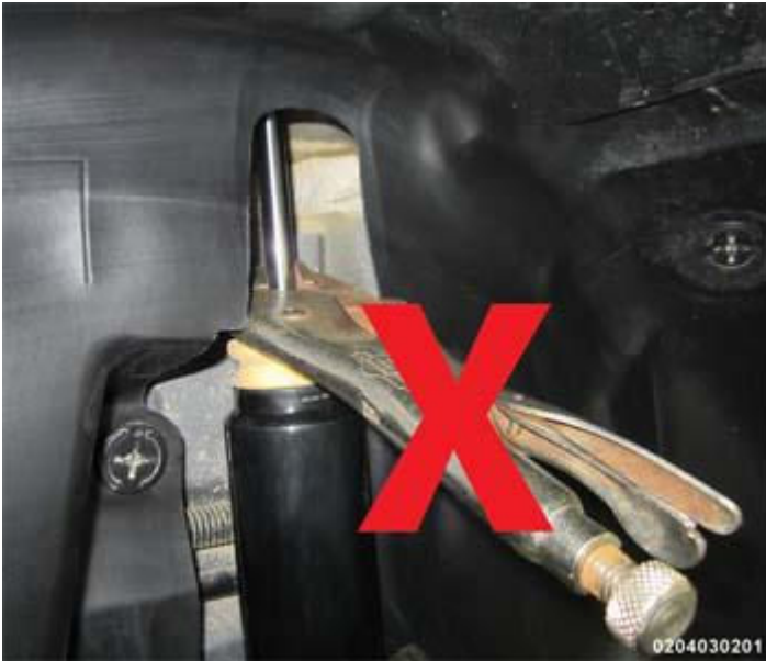
Fig. 42: Identifying Pliers On Chrome Machined Surface Of Shock/Strut Rod Courtesy of CHRYSLER GROUP, LLC
