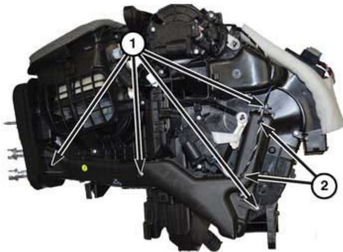
Fig. 128: Removing/Installing Heater Core Tubing Cover Courtesy of CHRYSLER GROUP, LLC
