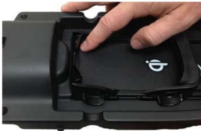
Fig. 45: Pushing Two Pins On Mat Into Blind Bosses Courtesy of CHRYSLER GROUP, LLC
