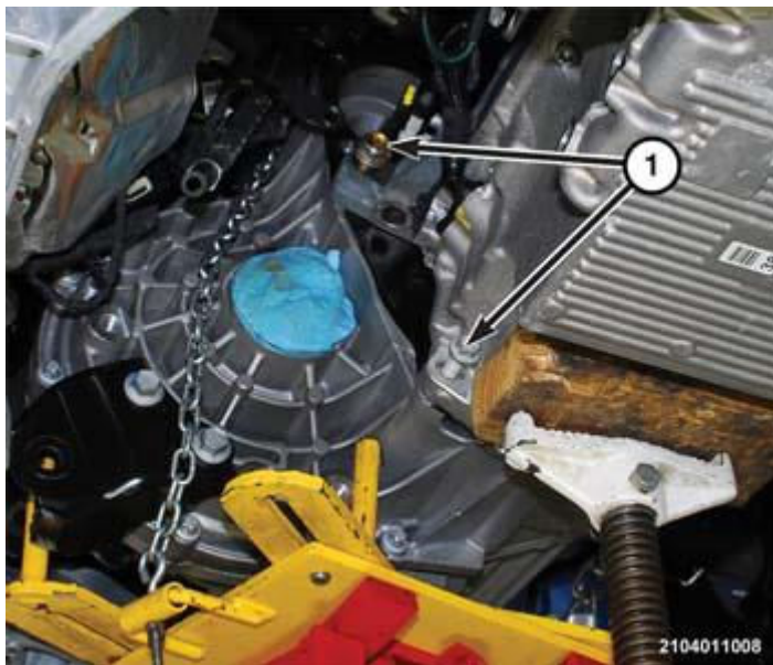
Fig. 78: Locating Bolts Holding Engine Block To Transmission Bellhousing & Bellhousing To Oil Pan
