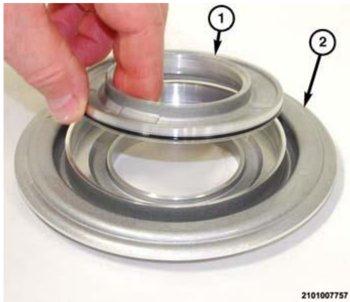
Fig. 417: Remove/Install Balance Piston At B-Clutch Piston Courtesy of CHRYSLER GROUP, LLC
