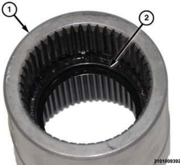
Fig. 643: View of Adapter Sleeve Seal Tension Spring Courtesy of CHRYSLER GROUP, LLC
