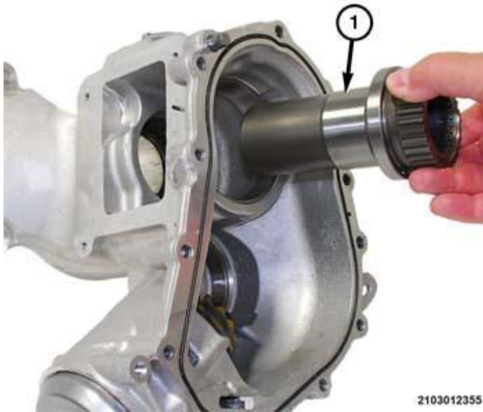
Fig. 19: Removing/Installing Input Shaft & Bearing At PTU Housing Courtesy of CHRYSLER GROUP, LLC
