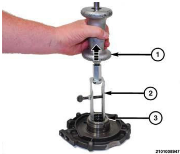
Fig. 463: Removing Dog F-Clutch Thrust Plate Courtesy of CHRYSLER GROUP, LLC
