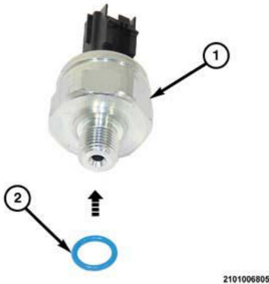
Fig. 635: Fluid Pressure Sensor & O-Ring Courtesy of CHRYSLER GROUP, LLC
