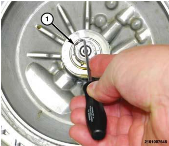
Fig. 119: Removing/Installing Inner Seal-Rings Courtesy of CHRYSLER GROUP, LLC
