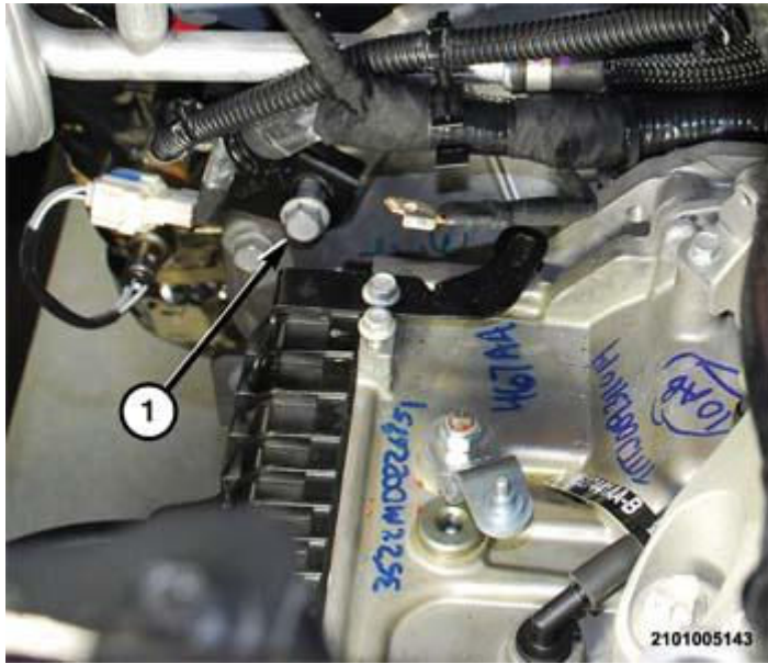
Fig. 25: Wire Harness Bracket & Bellhousing Bolt Courtesy of CHRYSLER GROUP, LLC
