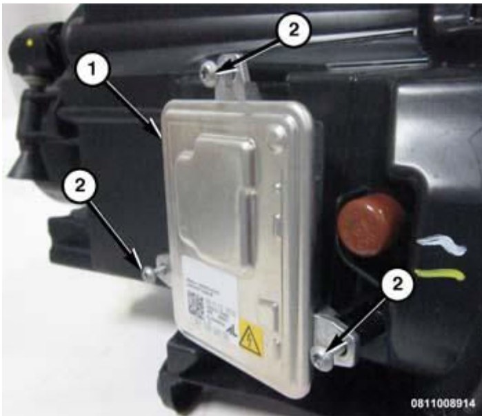
Fig. 6: Electronic Ballast Module & Screws Courtesy of CHRYSLER GROUP, LLC
