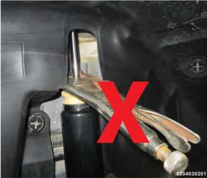
Fig. 27: Identifying Pliers On Chrome Machined Surface Of Shock/Strut Rod Courtesy of CHRYSLER GROUP, LLC
