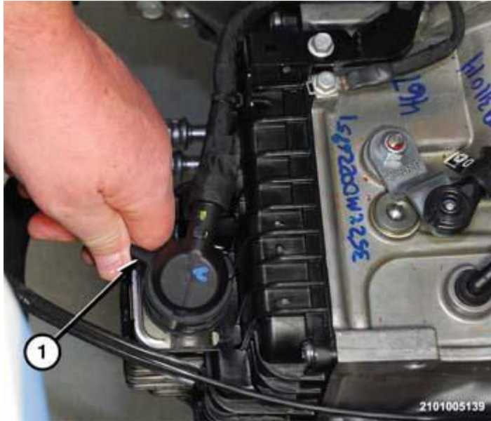
Fig. 20: Transmission Valve Body Solenoid Connector Courtesy of CHRYSLER GROUP, LLC
