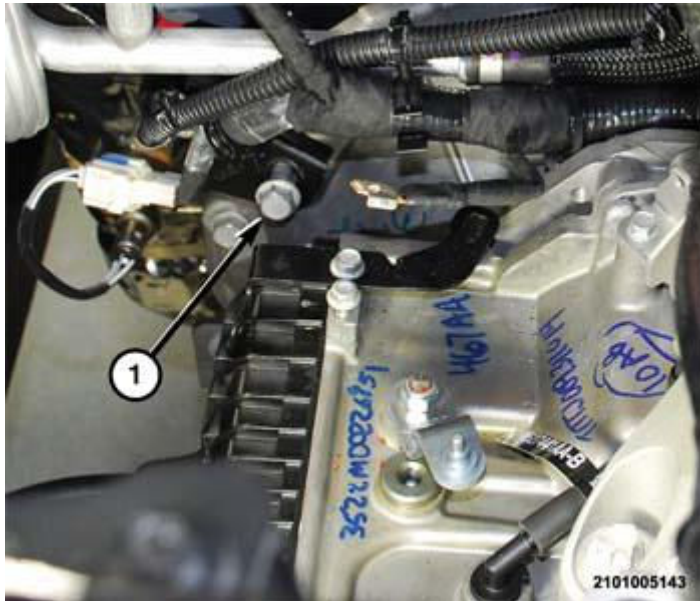
Fig. 216: Wire Harness Bracket & Bellhousing Bolt
