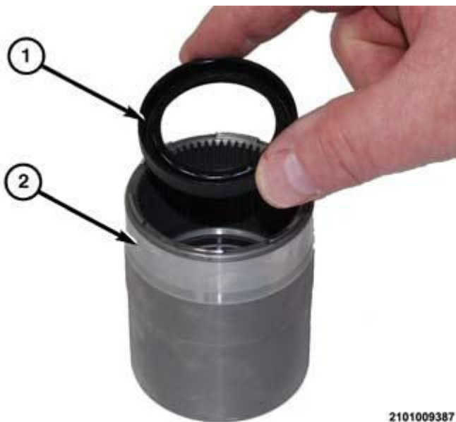
Fig. 657: Inserting Lip Seal Into Adapter Sleeve Courtesy of CHRYSLER GROUP, LLC
