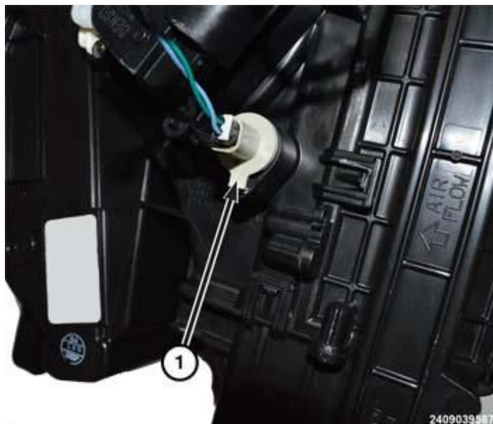
Fig. 26: Evaporator Temperature Sensor Location Courtesy of CHRYSLER GROUP, LLC
