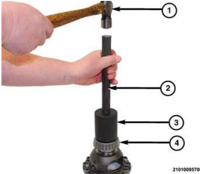
Fig. 289: Installing Differential Side Bearing Courtesy of CHRYSLER GROUP, LLC
