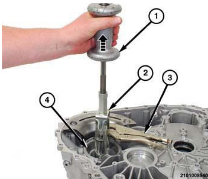
Fig. 286: Remove Bearing Race From Bellhousing Courtesy of CHRYSLER GROUP, LLC
