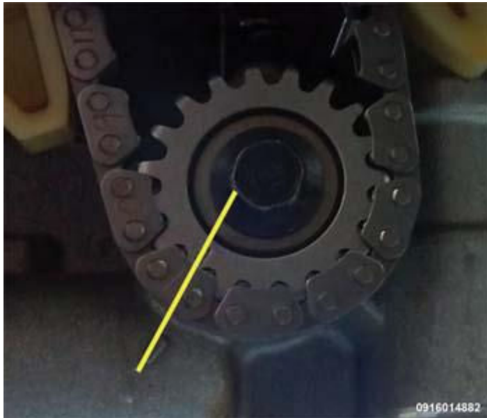
Fig. 370: Aligning Balance Shaft/Oil Pump Drive Gear And Housing Indicator Courtesy of CHRYSLER GROUP, LLC
