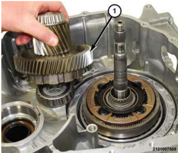
Fig. 79: Removing/Installing Transfer Gear Courtesy of CHRYSLER GROUP, LLC
