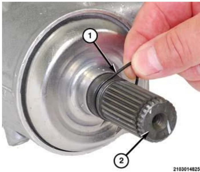
Fig. 56: Removing/Installing O-Ring At Rear Output Shaft Courtesy of CHRYSLER GROUP, LLC
