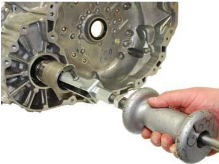
Fig. 641: Removing Differential Adapter Sleeve Courtesy of CHRYSLER GROUP, LLC
