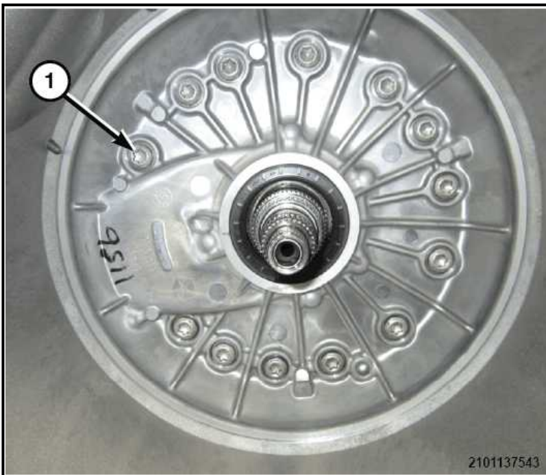
1 - Oil Pump Housing Bolts
