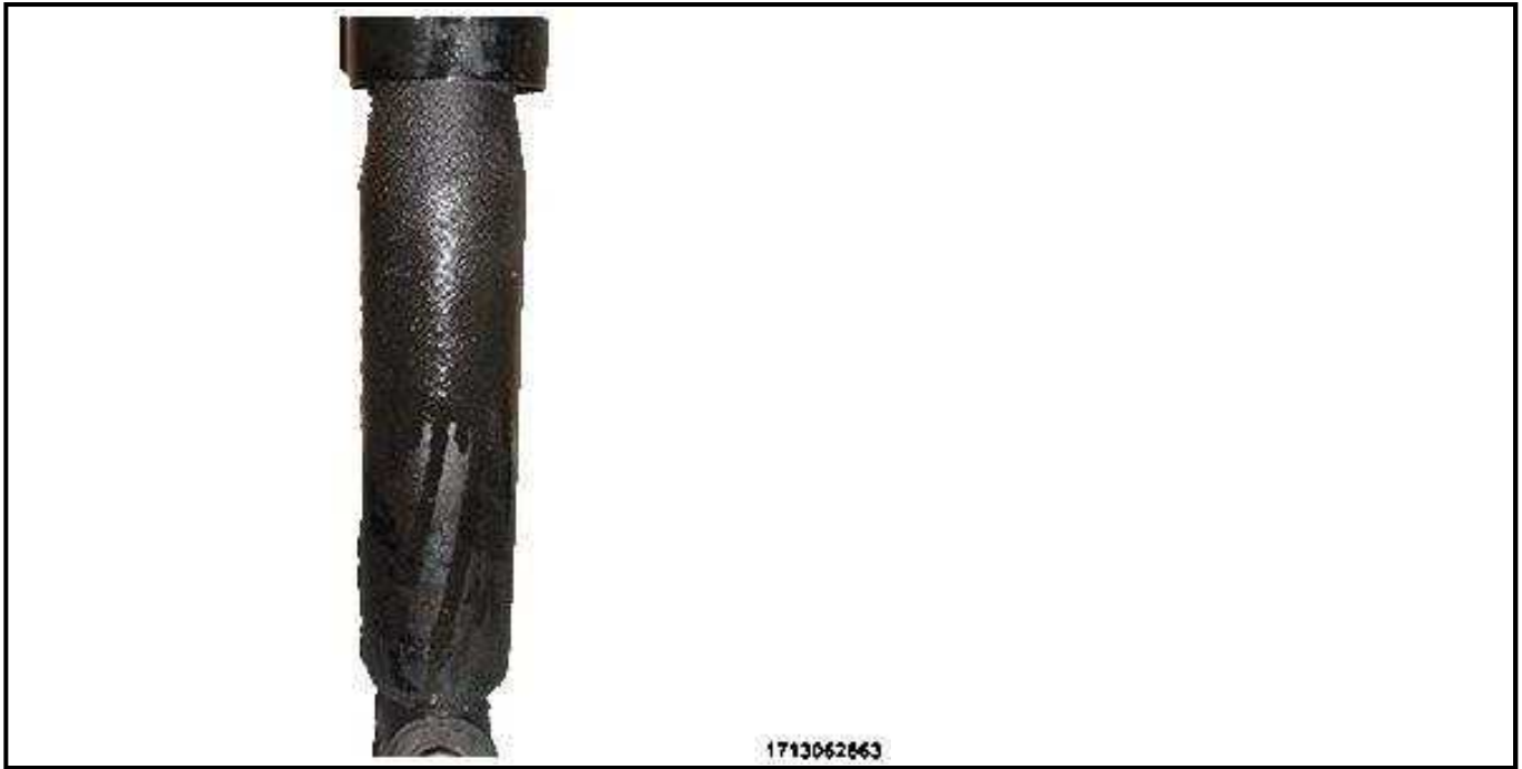
FAILED LEAKING SHOCK (REPLACE)
