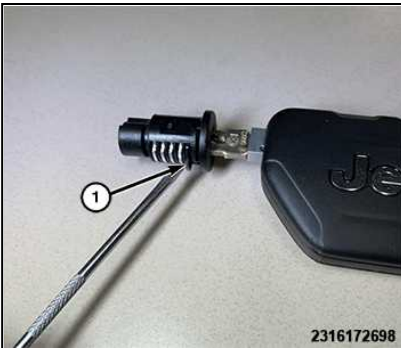
1 - Lock Cylinder Release Tab
