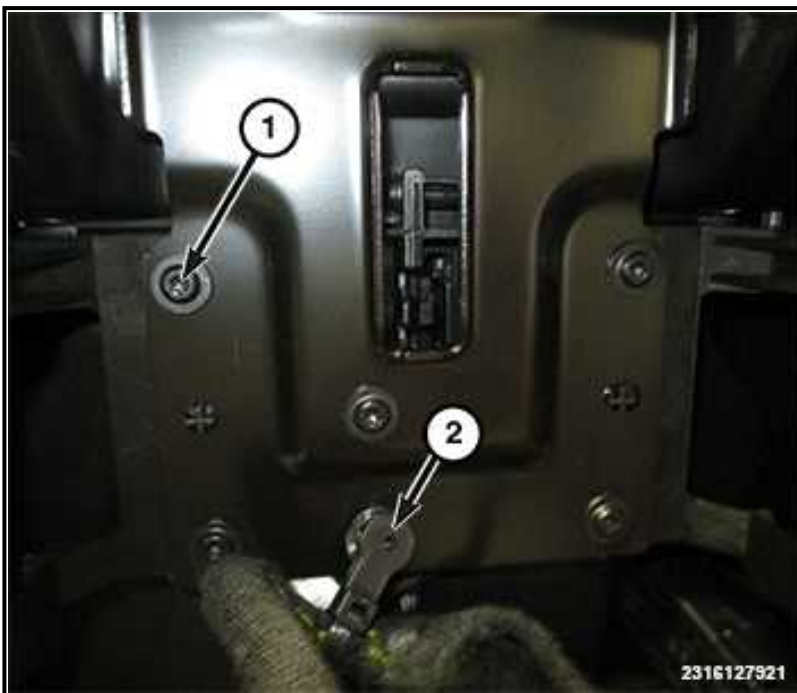
1 - Screws 2 - Wire Harness Retaining Clip
