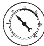
LATE VALVE TIMING, VACUUM LEAK AT IDLE
