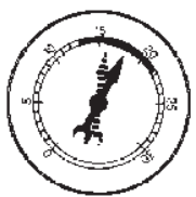
POOR VALVE SEATING AT IDLE
