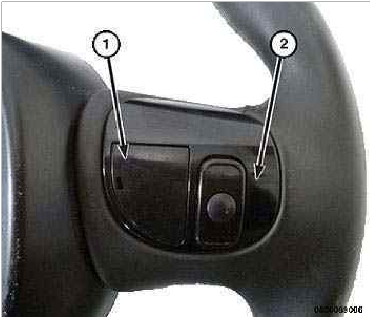
Fig 3: Remote Radio Switch & Cover
