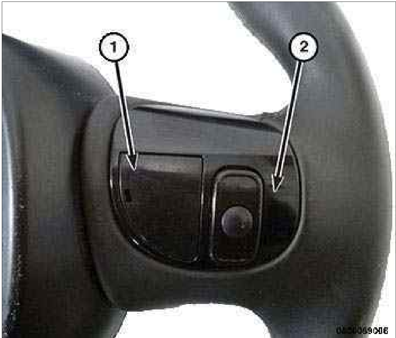
Fig 1: Remote Radio Switch & Cover
