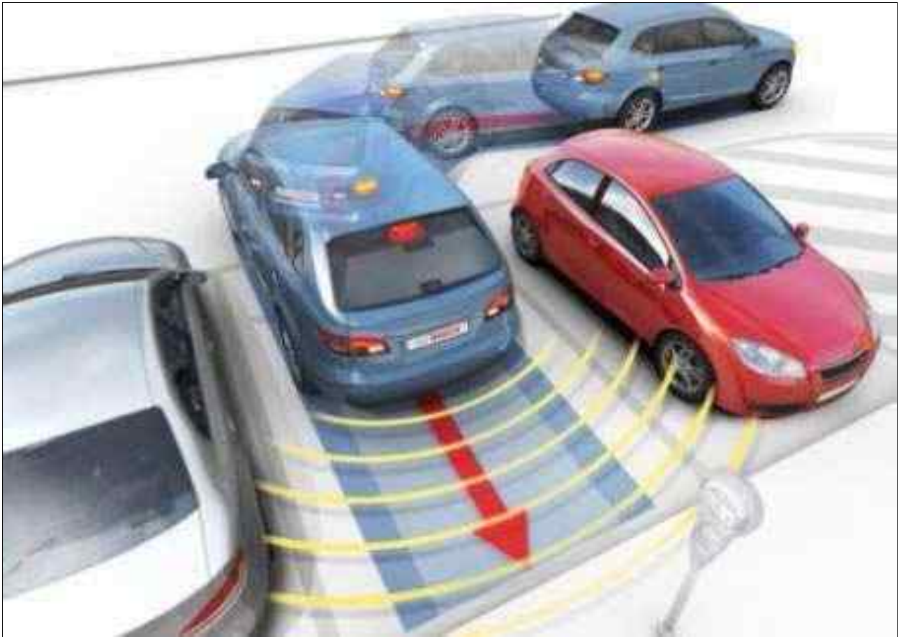
Fig 5: Semi-Automatic Parking Assist System (Perpendicular Parking)
