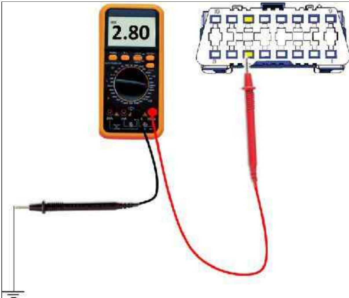
Fig 3: Checking Voltage On CAN-C1 (High +)
