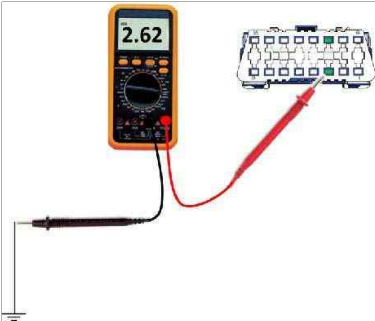
Fig 7: Checking Voltage On CAN-BH (High +)
