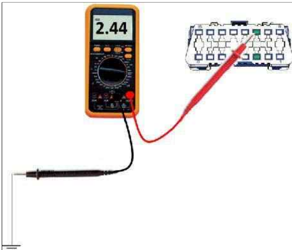
Fig 8: Checking Voltage On CAN-BH (Low -)
