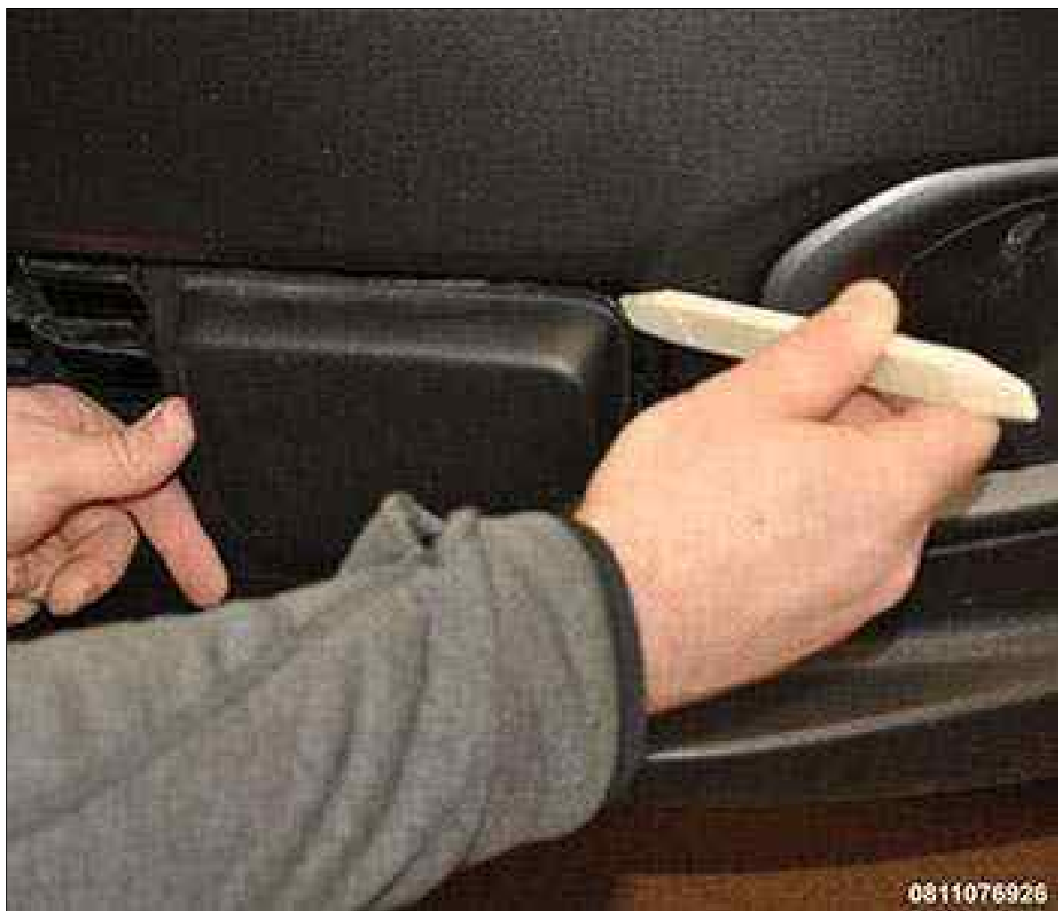
Fig 8: Removing Trim Cover
