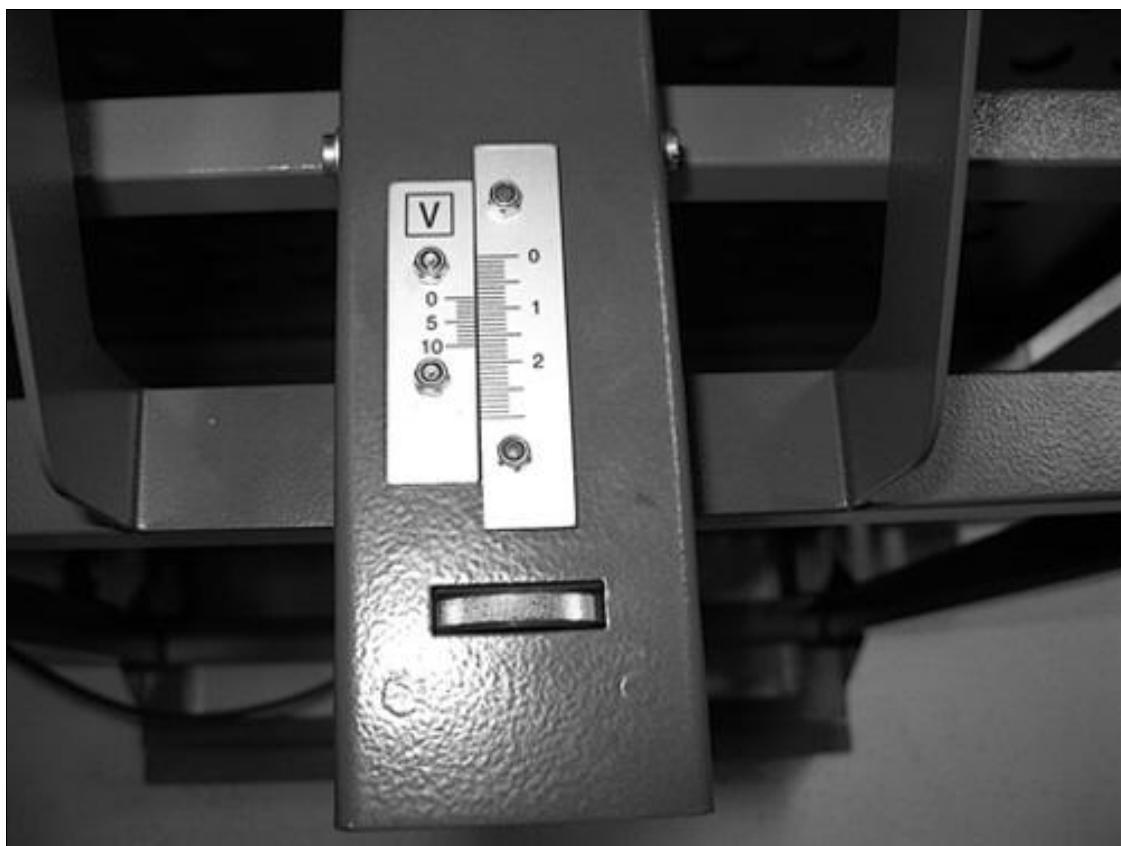
Fig 9: Vertical Adjustment Thumbscrew
