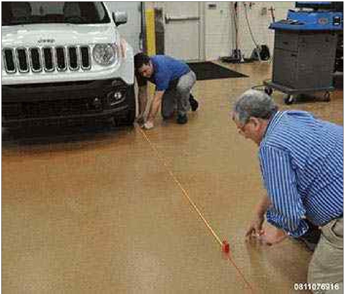
Fig 6: Measuring Distance From Front Wheel
