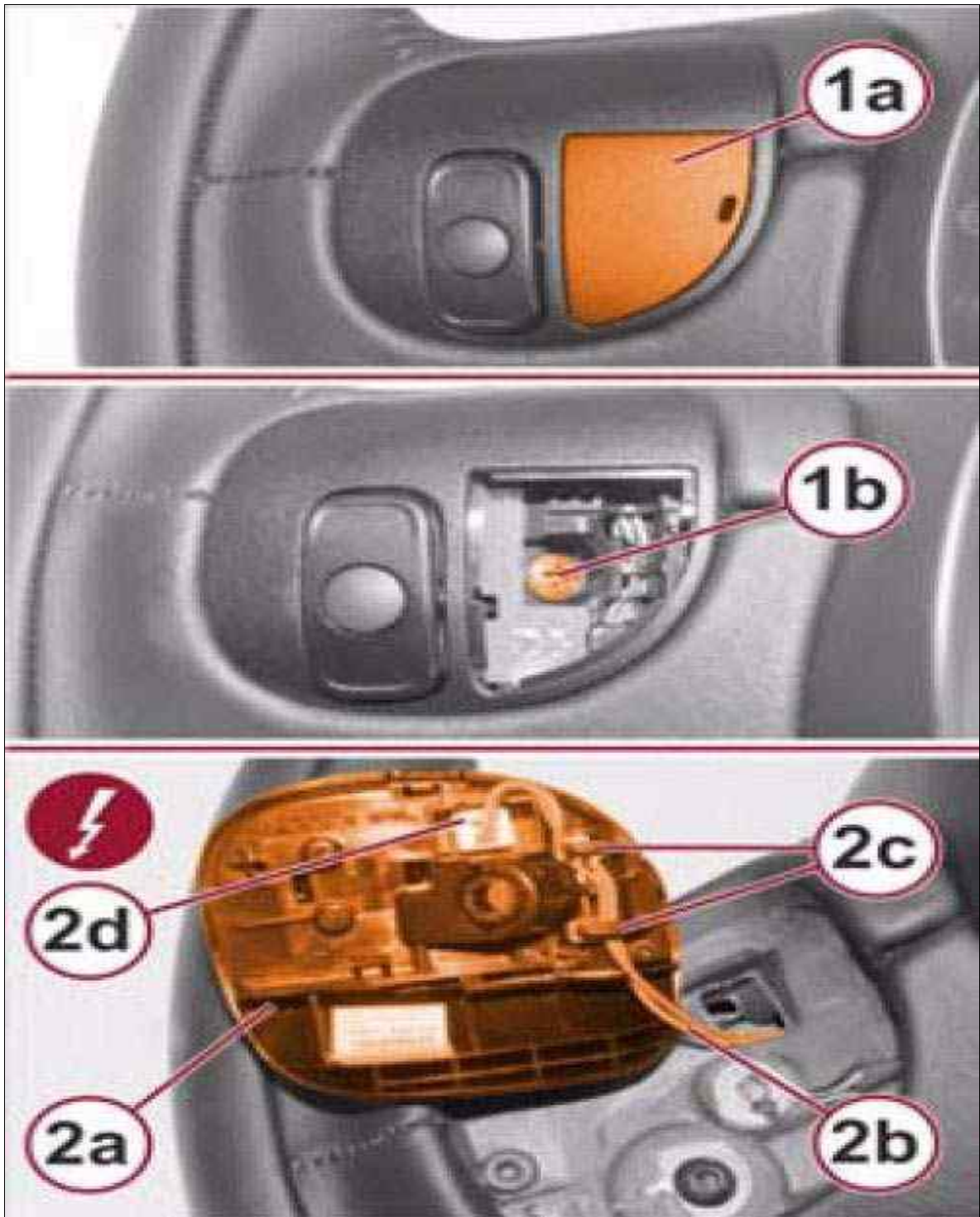
Fig 3: Cover, Screw, Module, Wiring, Retainers & Connector
