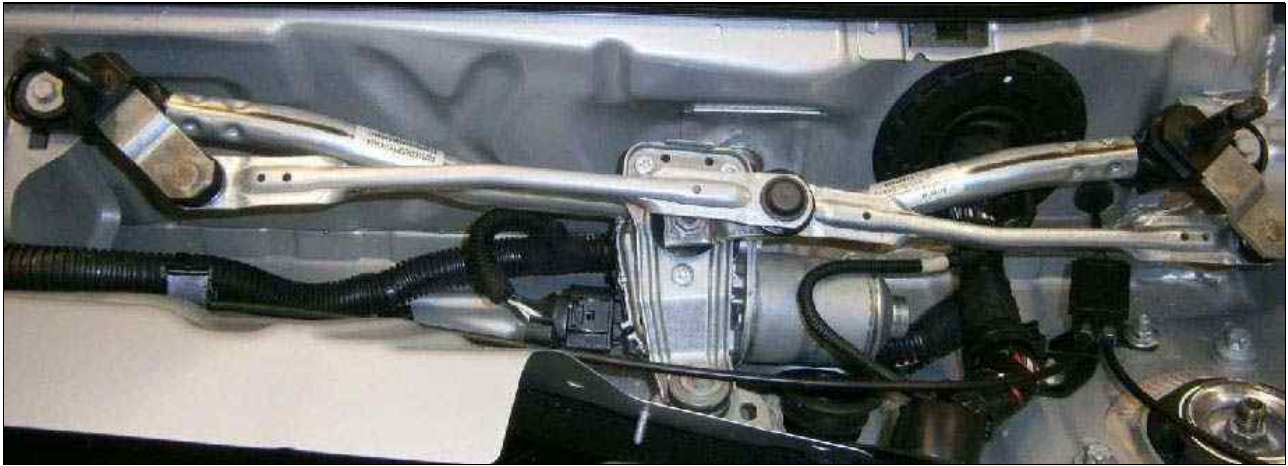
Fig 1: Front Electric Motor Connected To Front Wiper Mechanism
