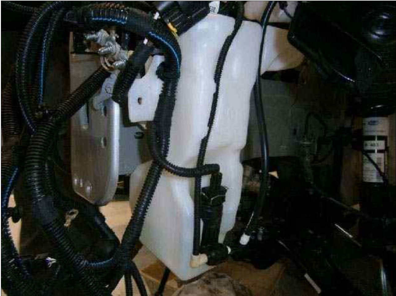
Fig 1: Two-Way Electric Pump & Washer Fluid Reservoir
