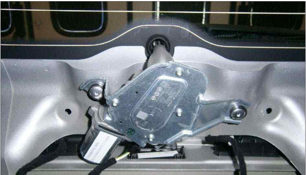
Fig 2: Rear Electric Motor Connected To Rear Wiper Mechanism
