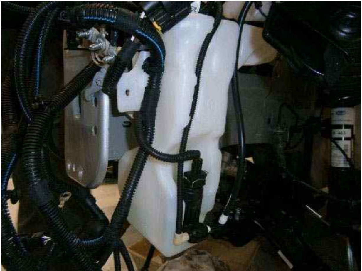
Fig 4: Two-Way Electric Pump & Washer Fluid Reservoir
