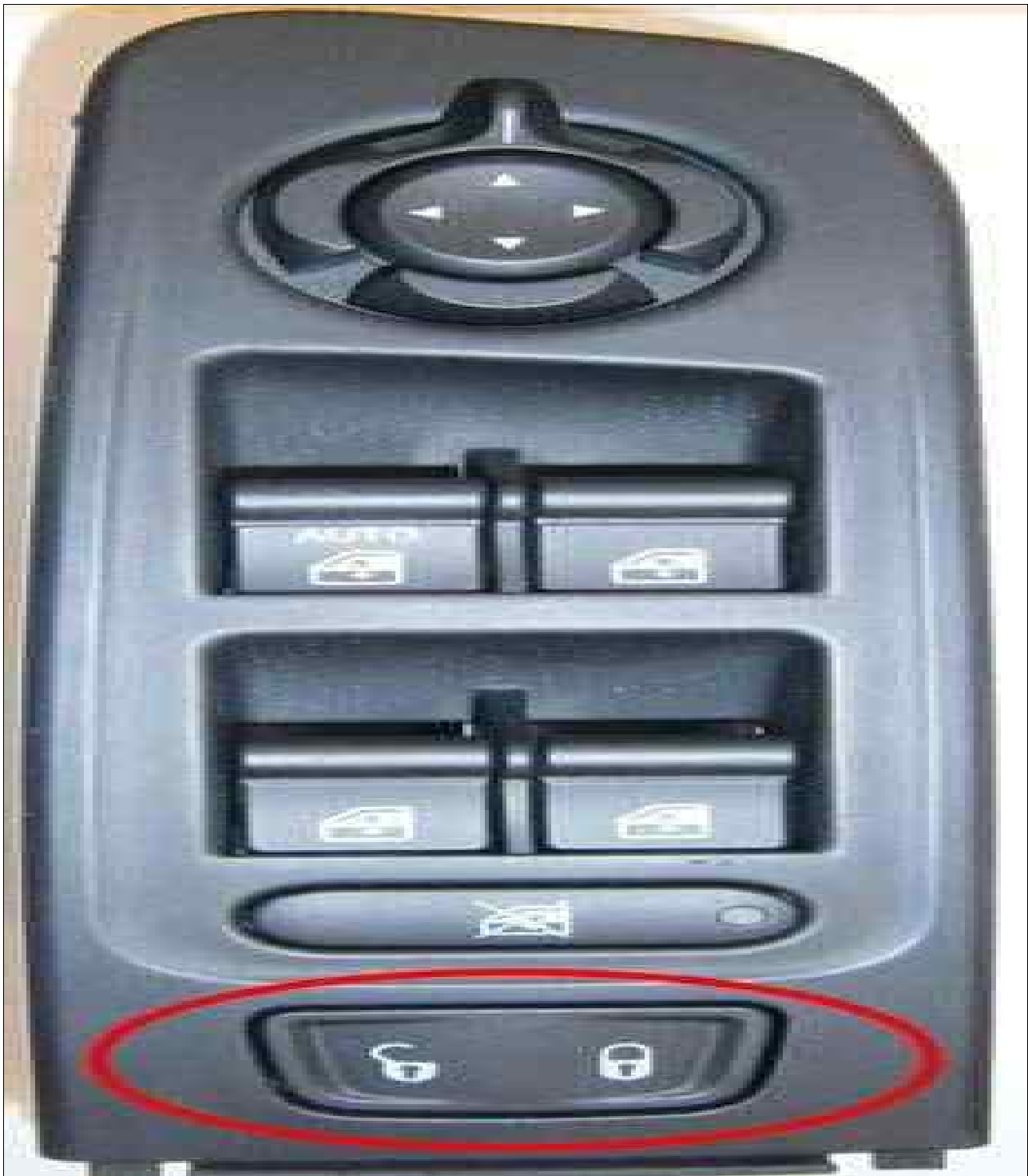
Fig 1: Door Lock And Unlock Switch
