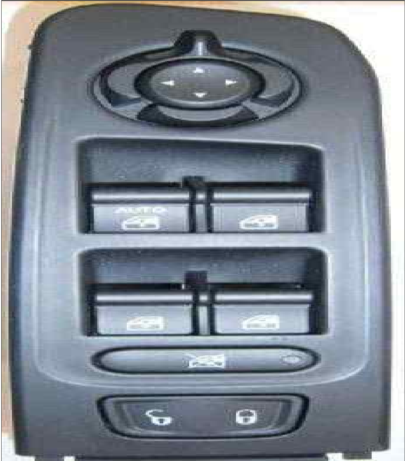
Fig 1: Power Window Switch Module
