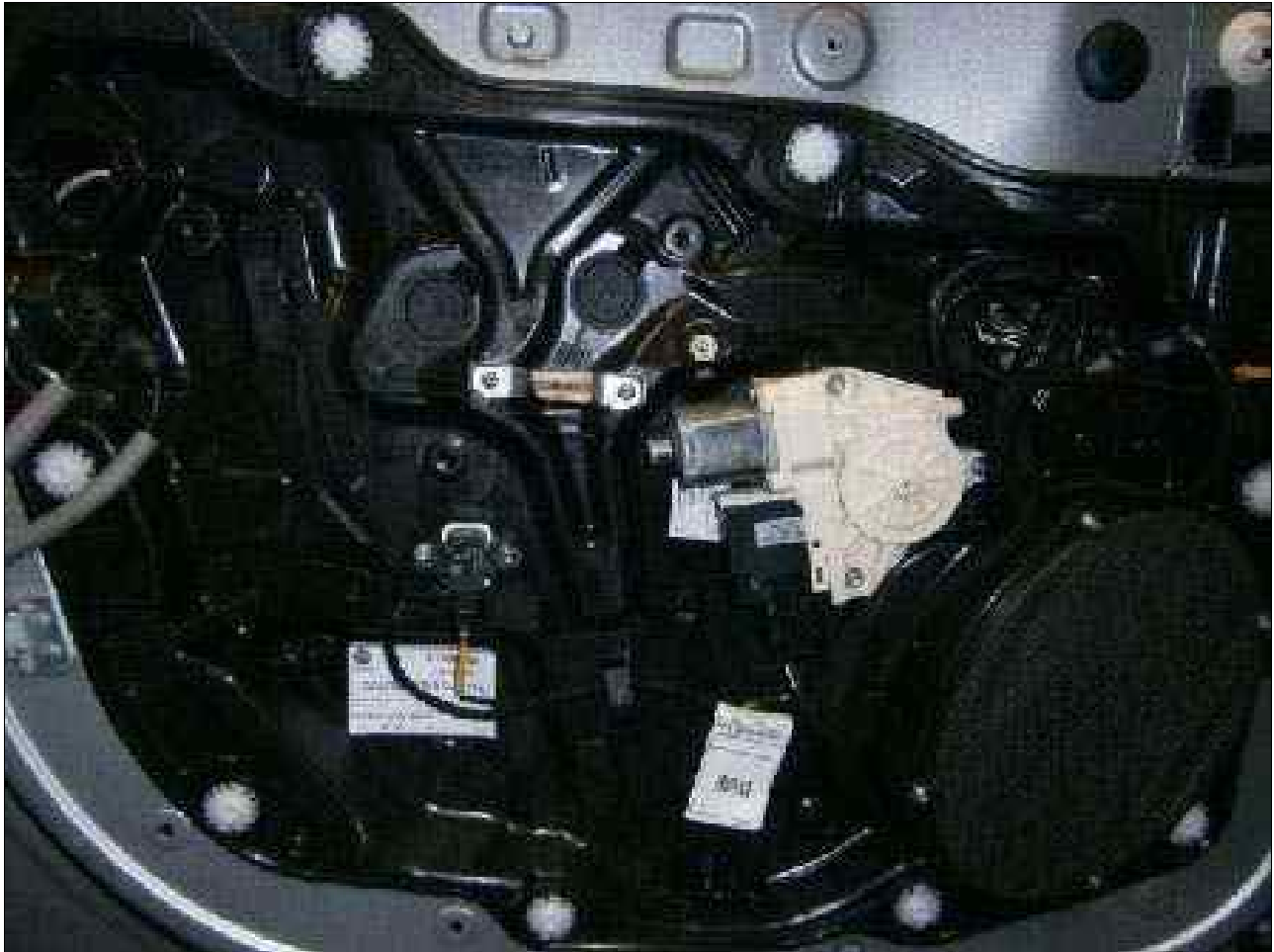
Fig 2: Window Movement Mechanism & Carrier
