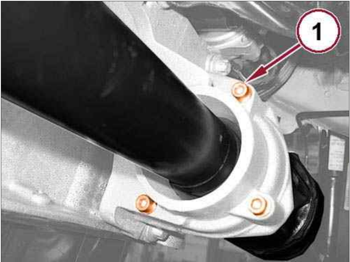
Fig 6: Intermediate Shaft Bearing Bolts
