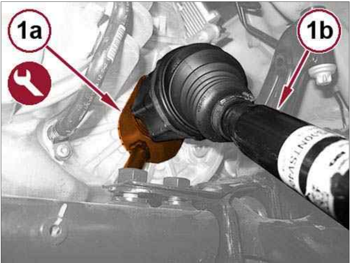
Fig 6: Removing Halfshaft With Special Tool
