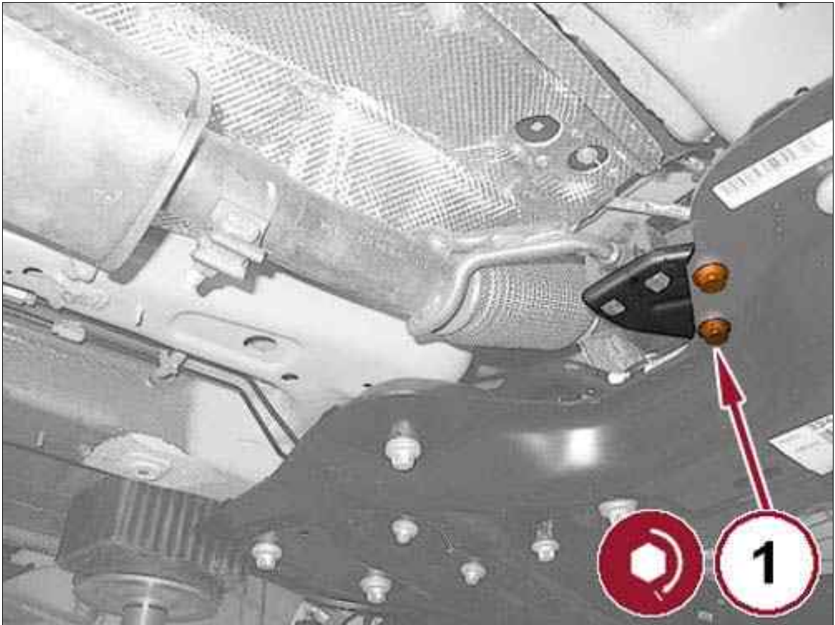
Fig 5: Exhaust Pipe Mounting Bracket Screws
