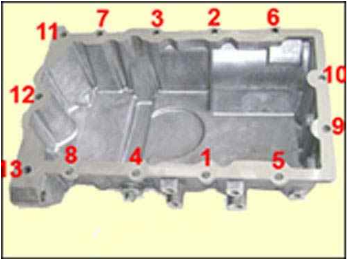
Fig 43: Oil Pan Bolt Tightening Sequence
