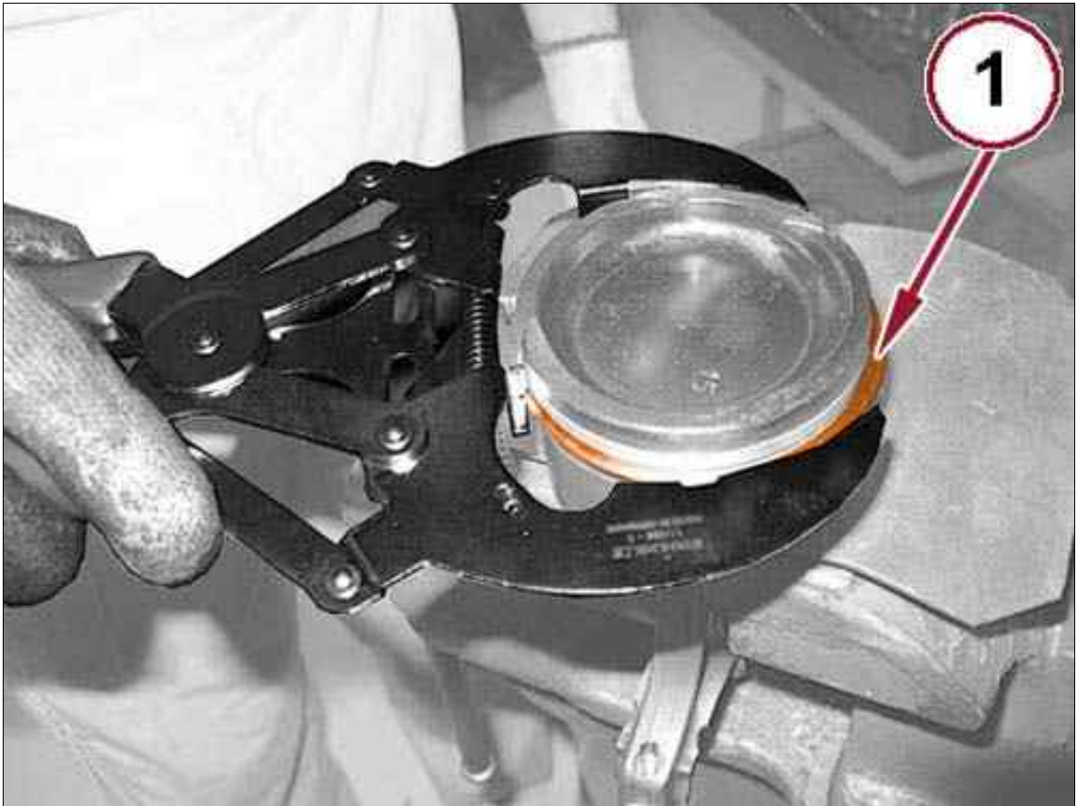
Fig 1: Removing Sealing Rings From Piston
