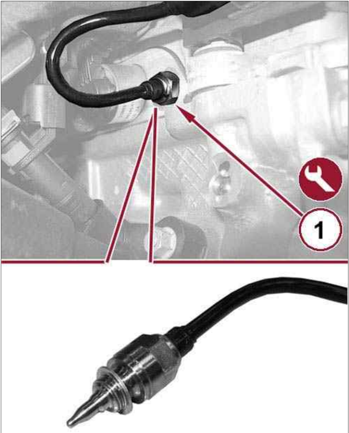
Fig 2: Removing & Installing Oil Temperature Sensor At MULTIAIR Actuator
