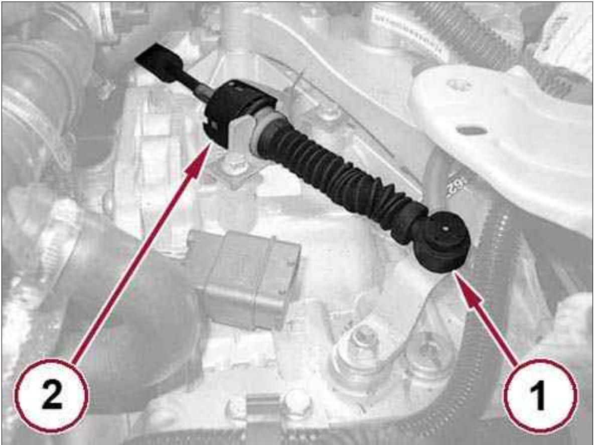
Fig 18: Gear Selector Cable At Gear Change Lever & Lock Slider
