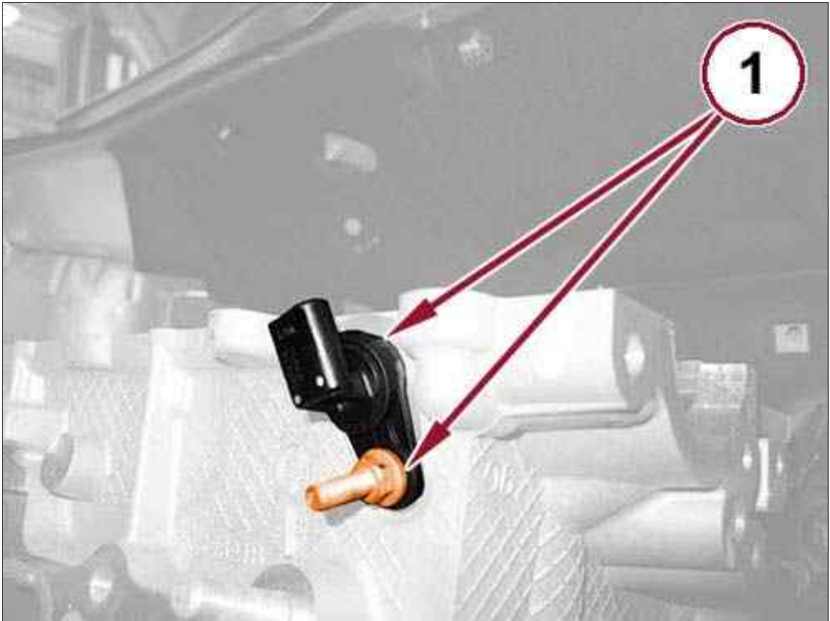
Fig 4: Cam Angle Sensor & Bolt
