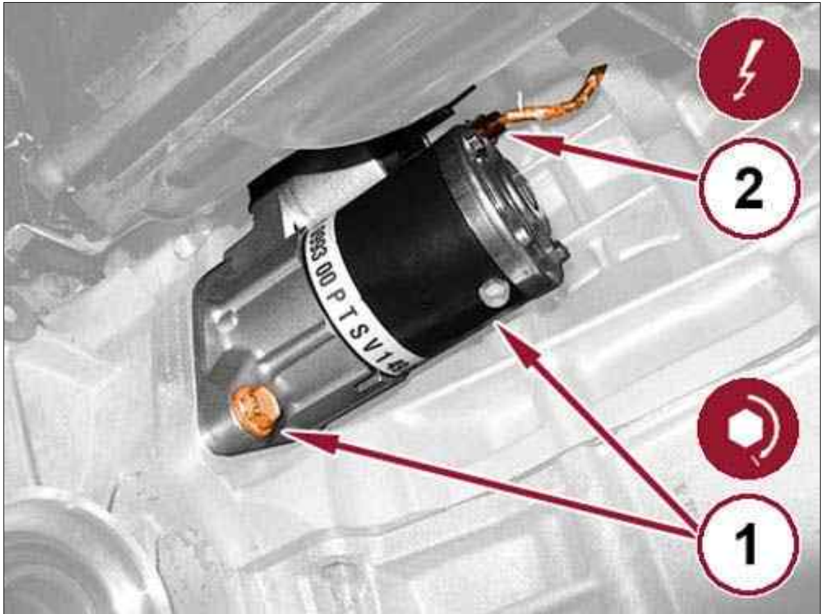
Fig 5: Starter Motor Wire Harness Connector & Lower Starter Bolt
