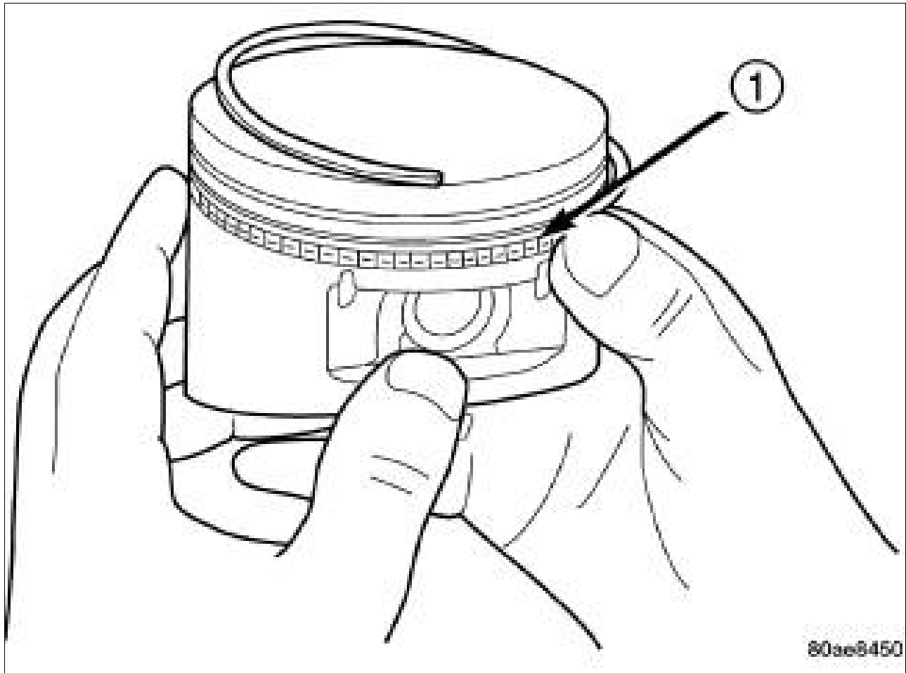
Fig 2: Installing Piston Ring Side Rail
