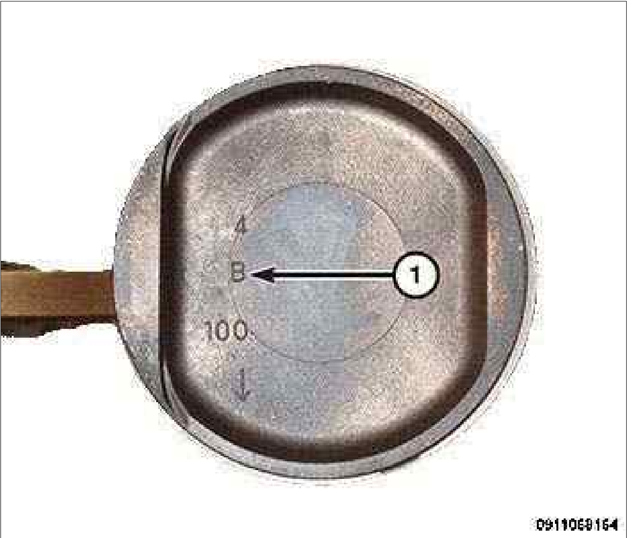
Fig 2: Piston Size Marked On Piston Crown
