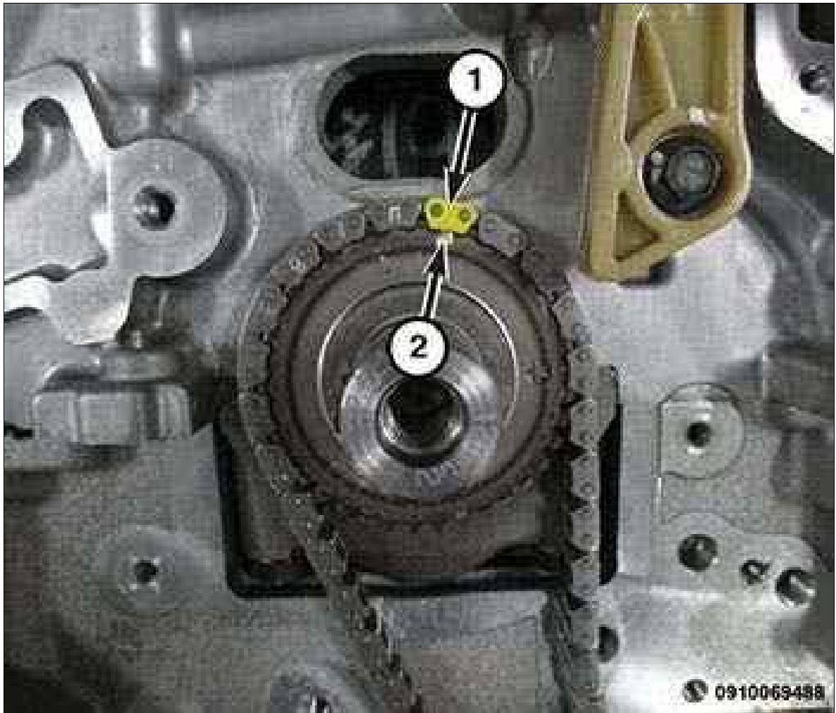
Fig 1: Marking Chain Link Corresponding To Crankshaft Sprocket Timing Mark
