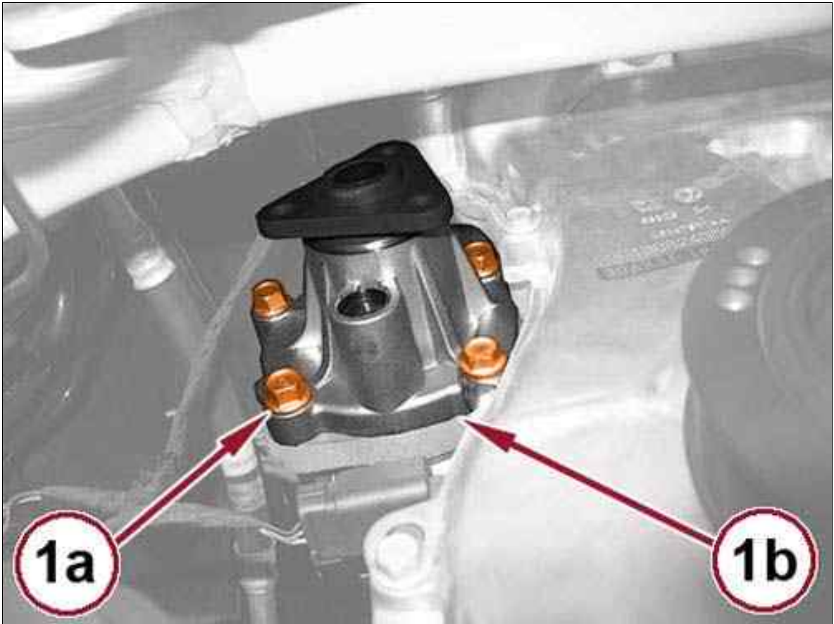
Fig 2: Water Pump & Bolts
