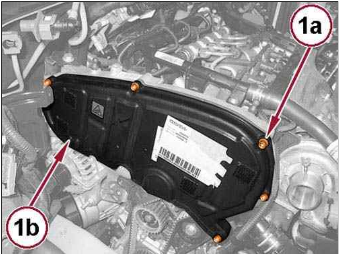
Fig 3: Timing Cover & Screws
