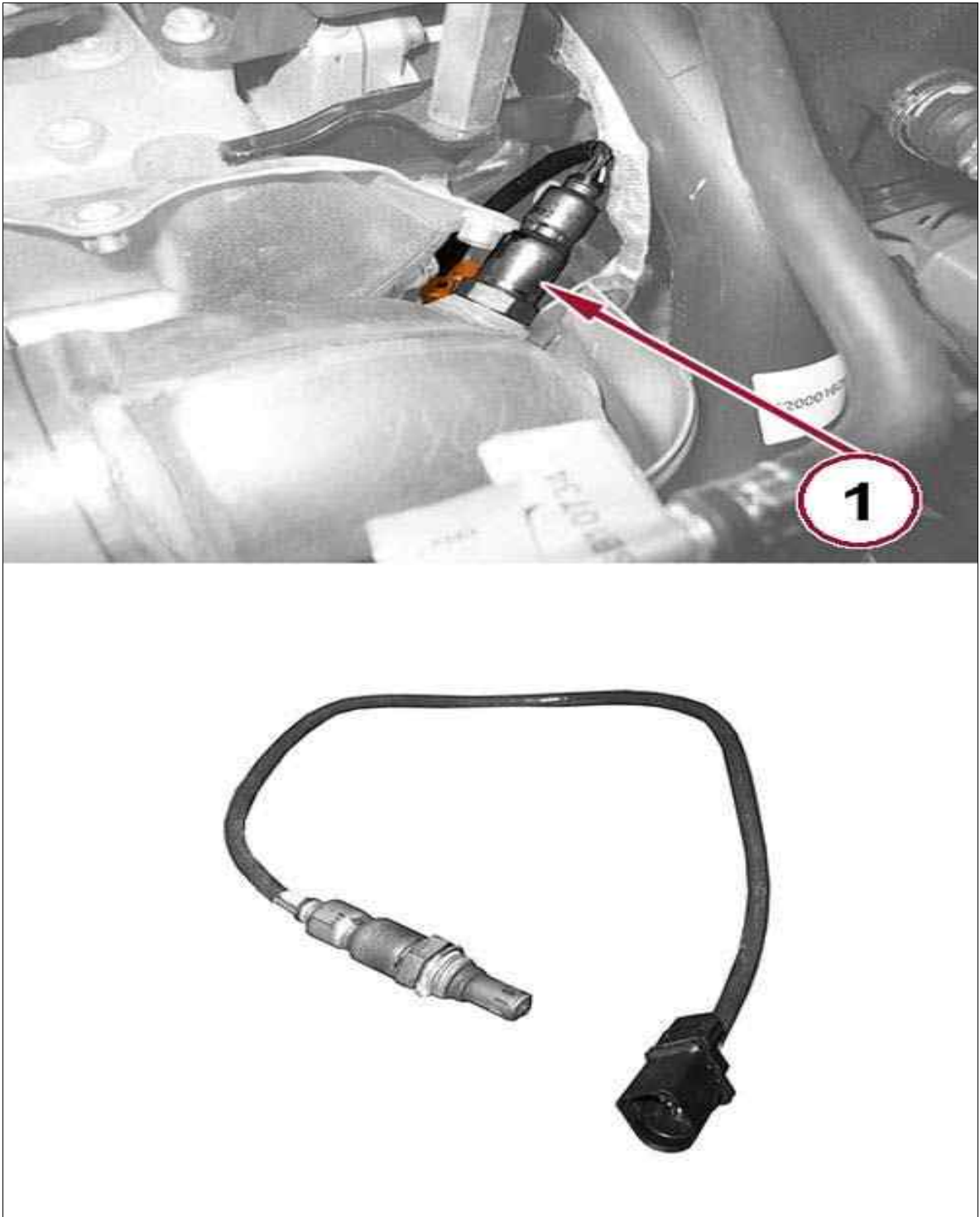
Fig 5: Upstream Oxygen Sensor At The Catalytic Converter
