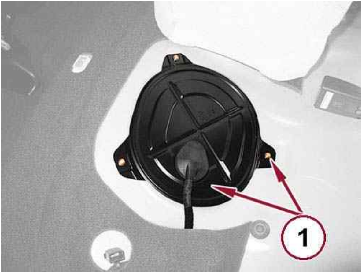
Fig 1: Fuel Pump Access Cover & Screws
