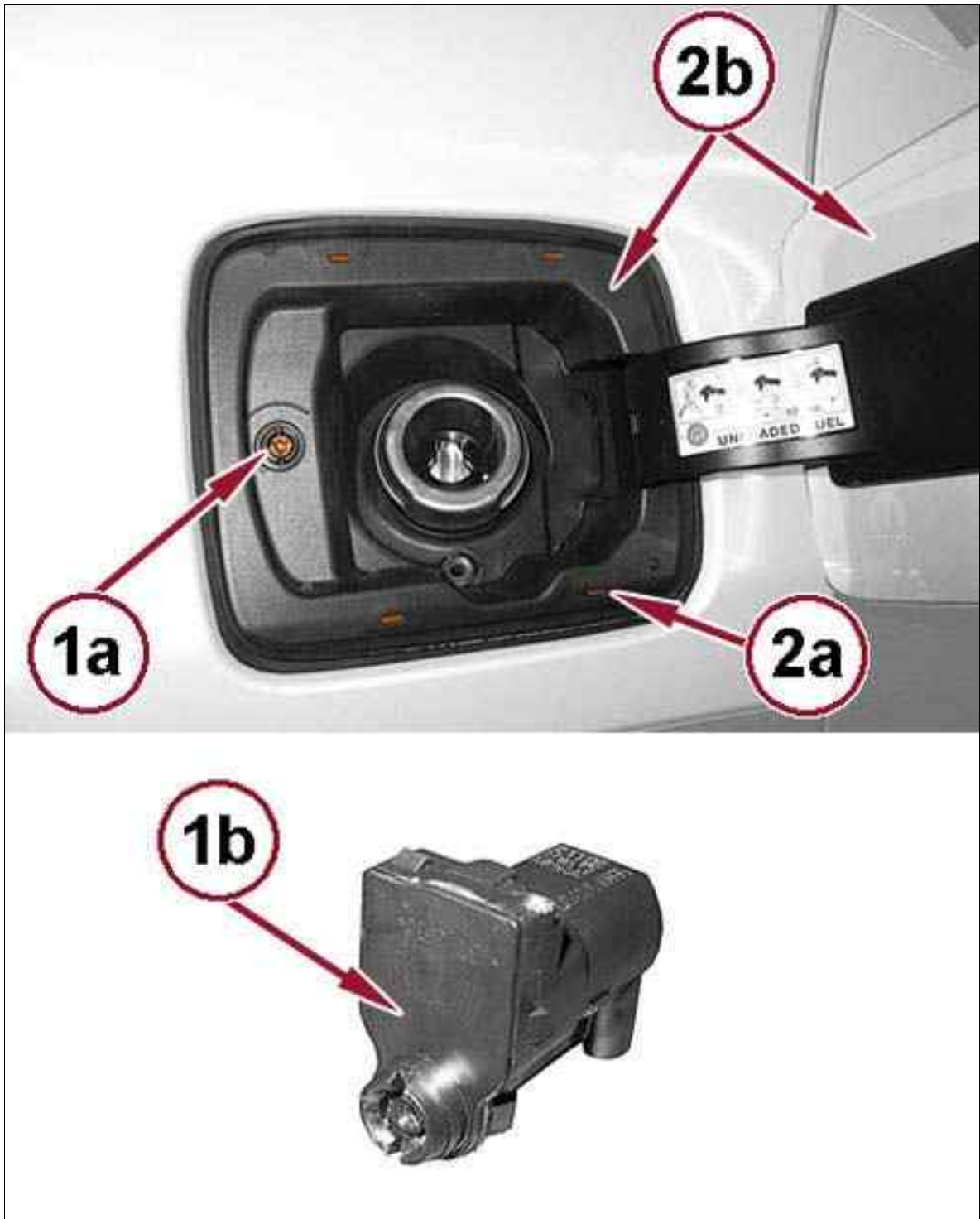
Fig 1: Door Retention Device, Fuel Door, Clips & Screw
