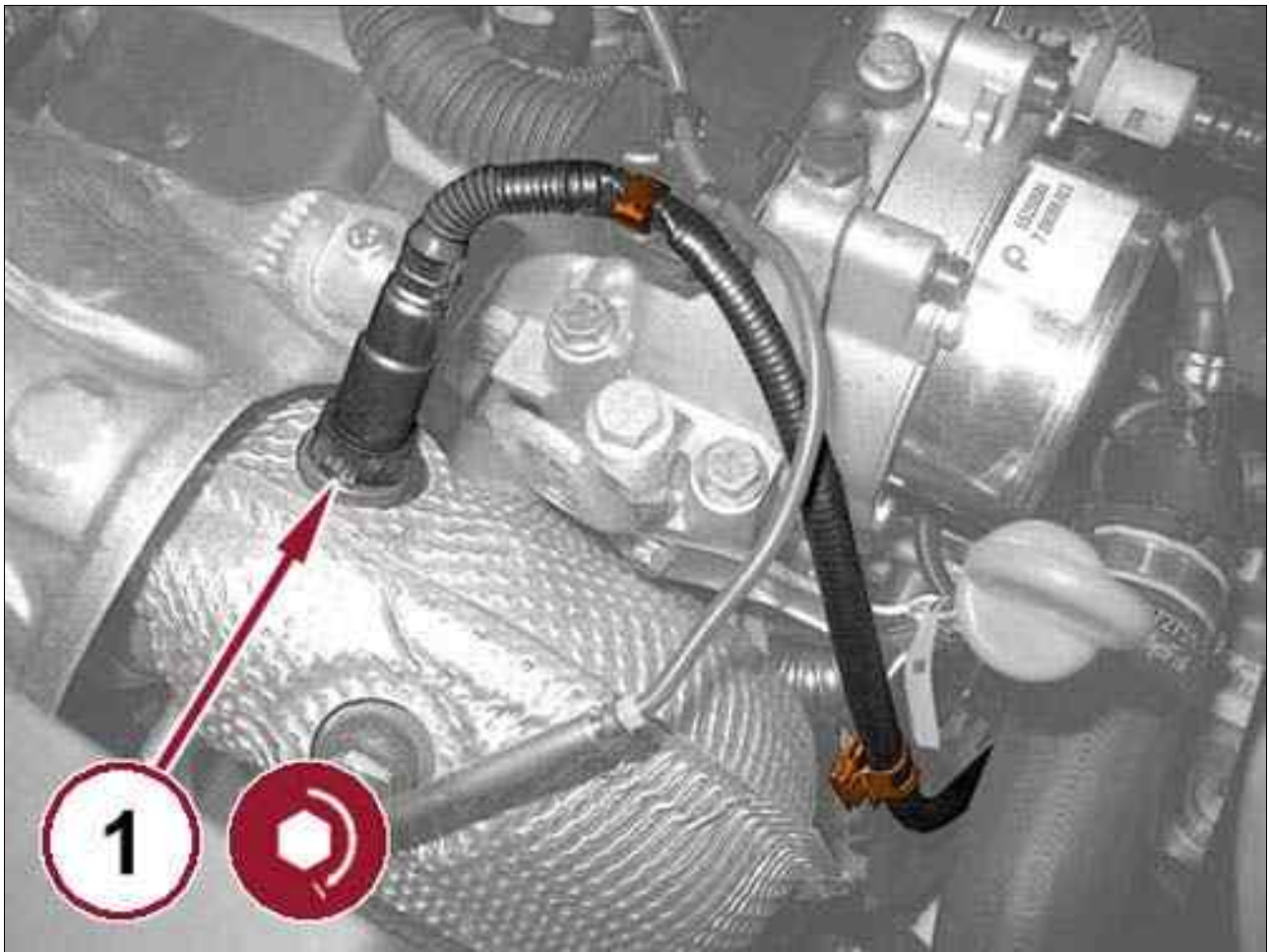
Fig 1: Upstream Oxygen Sensor & Retaining Clips
