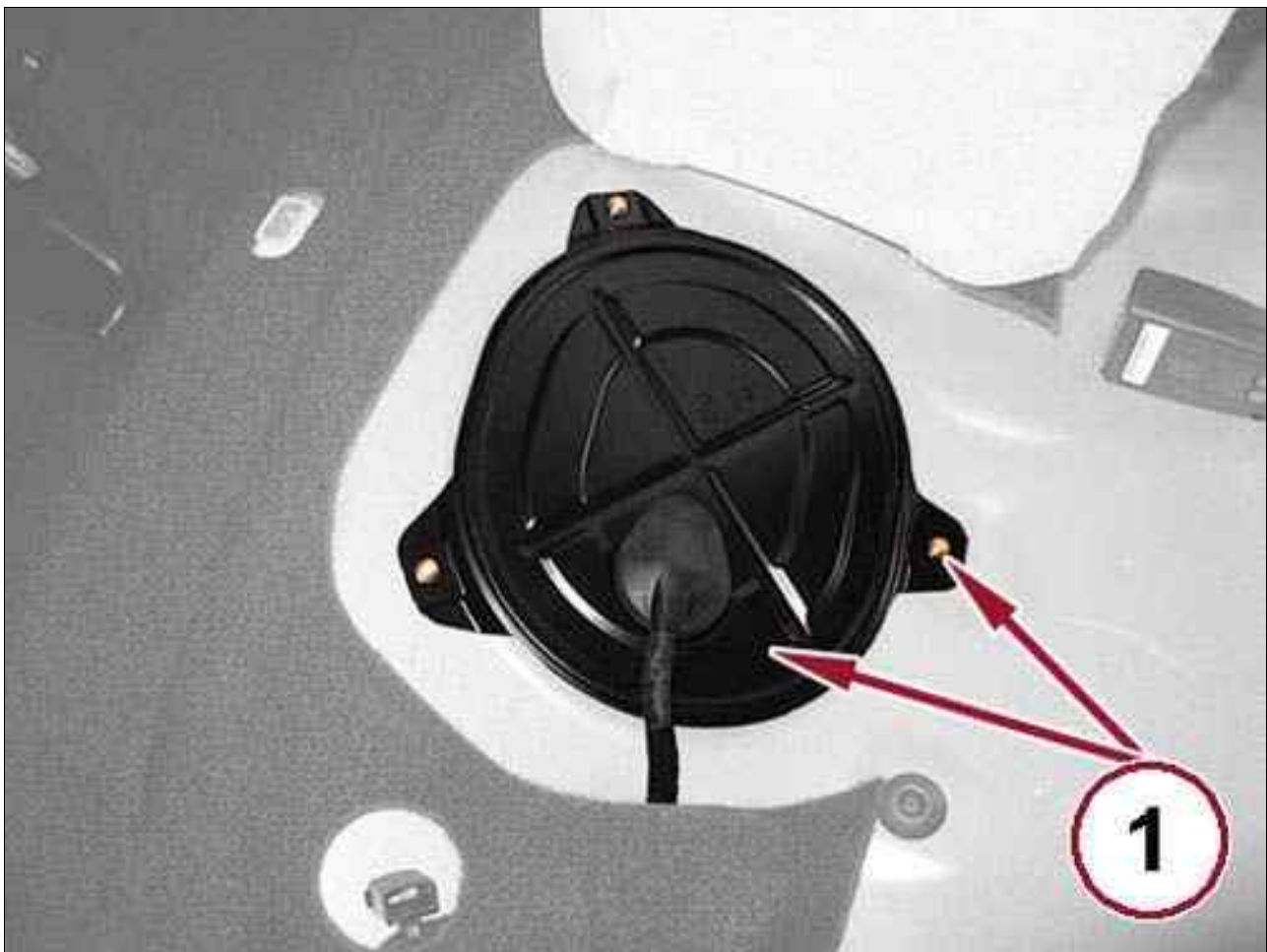
Fig 1: Fuel Pump Access Cover & Screws
