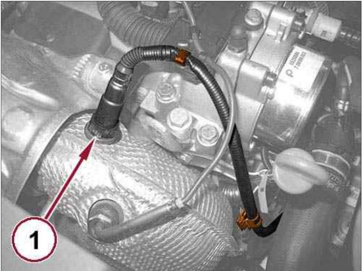
Fig 2: Upstream Oxygen Sensor & Retaining Clips
