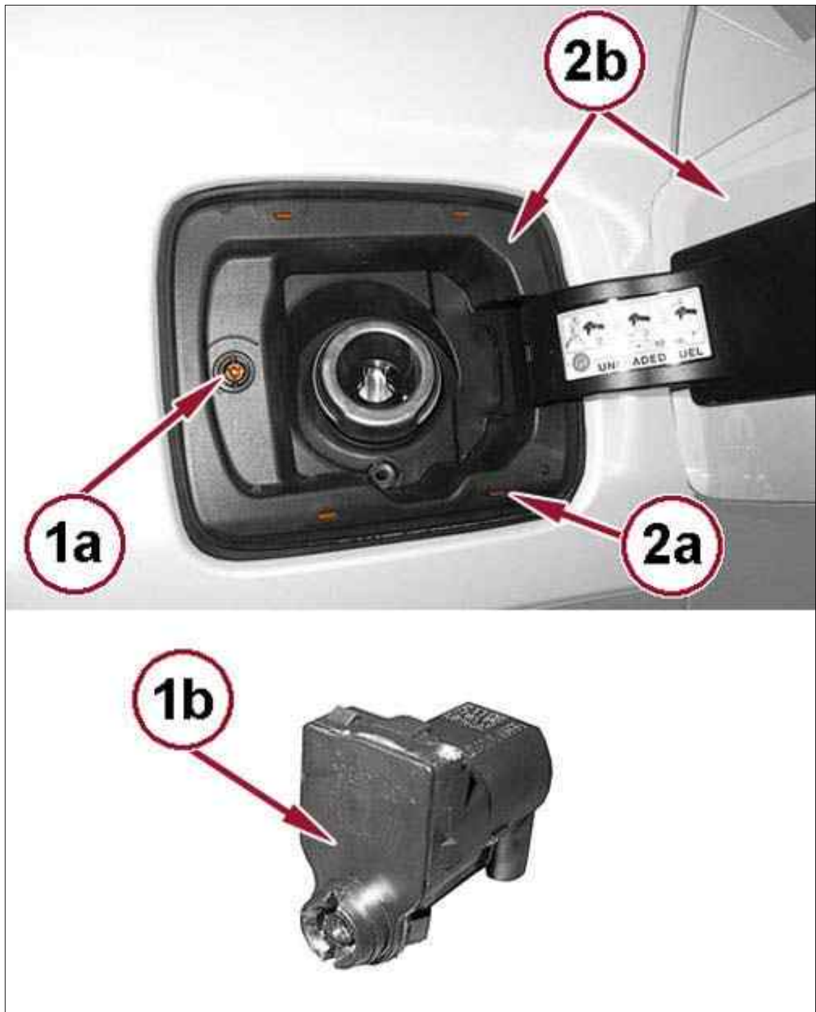
Fig 4: Door Retention Device, Fuel Door, Clips & Screw
