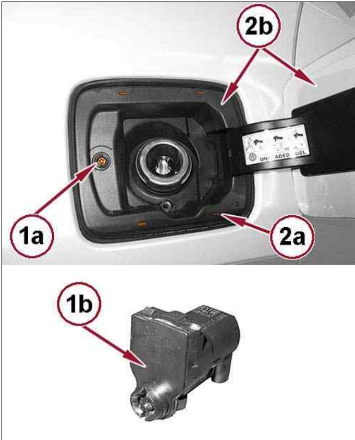
Fig 4: Door Retention Device, Fuel Door, Clips & Screw
