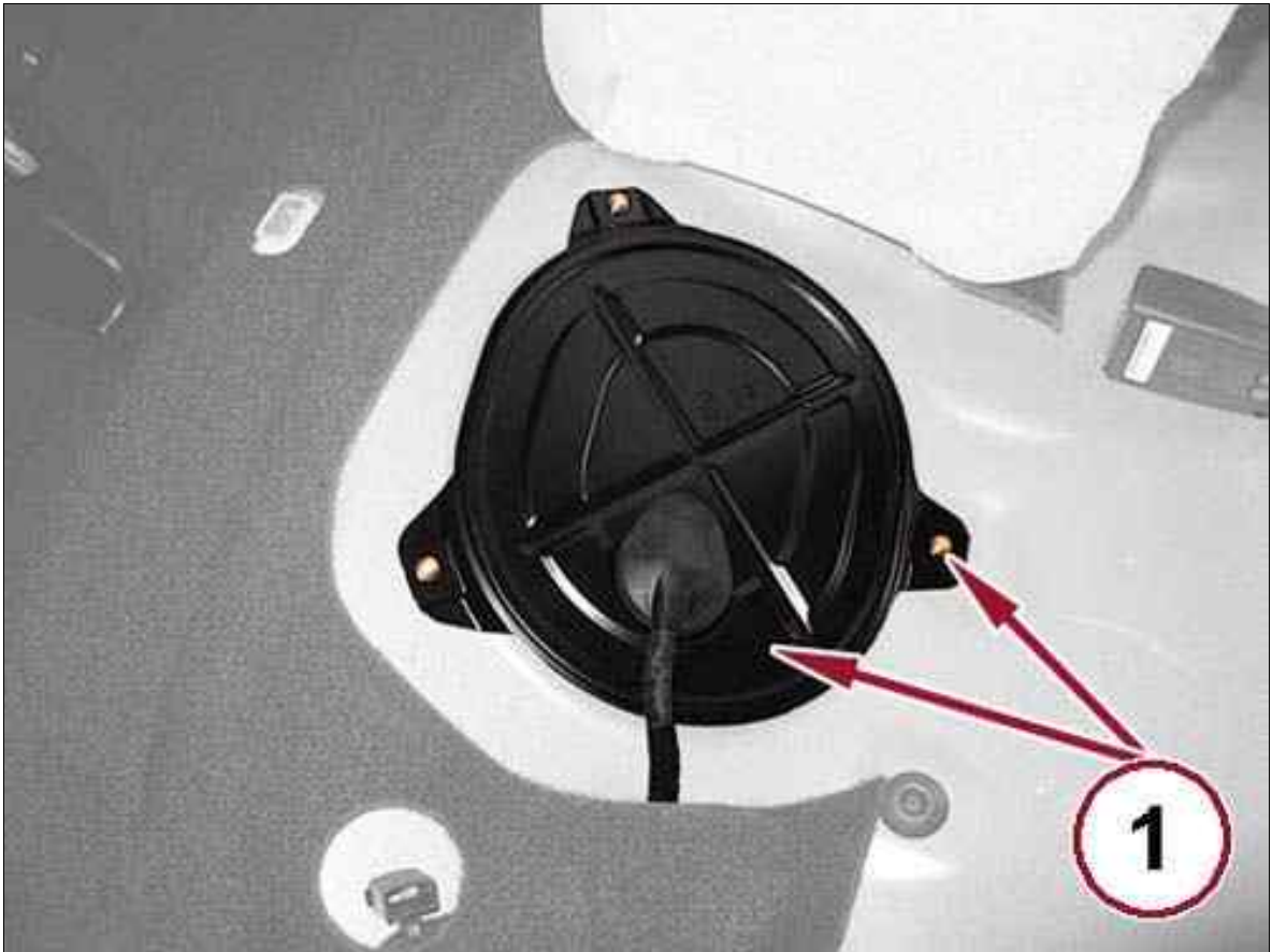
Fig 9: Fuel Pump Access Cover & Screws
