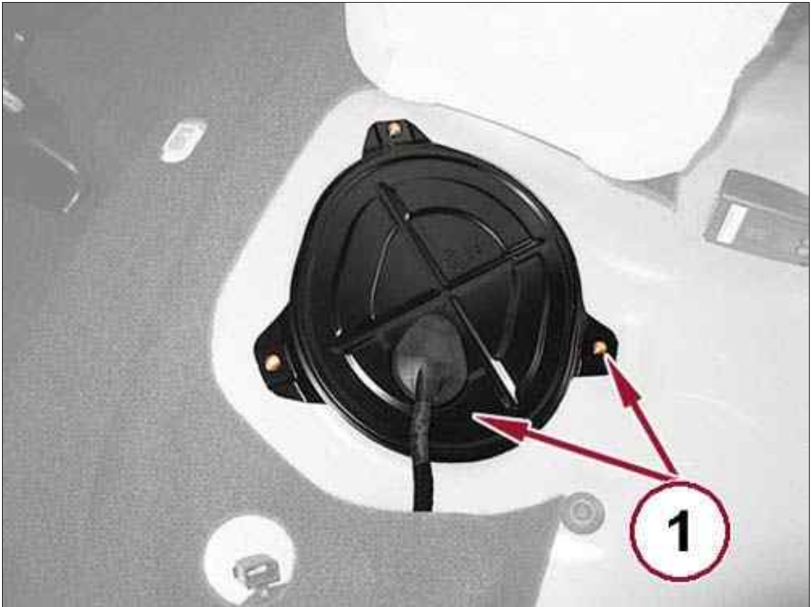
Fig 3: Fuel Pump Access Cover & Screws
