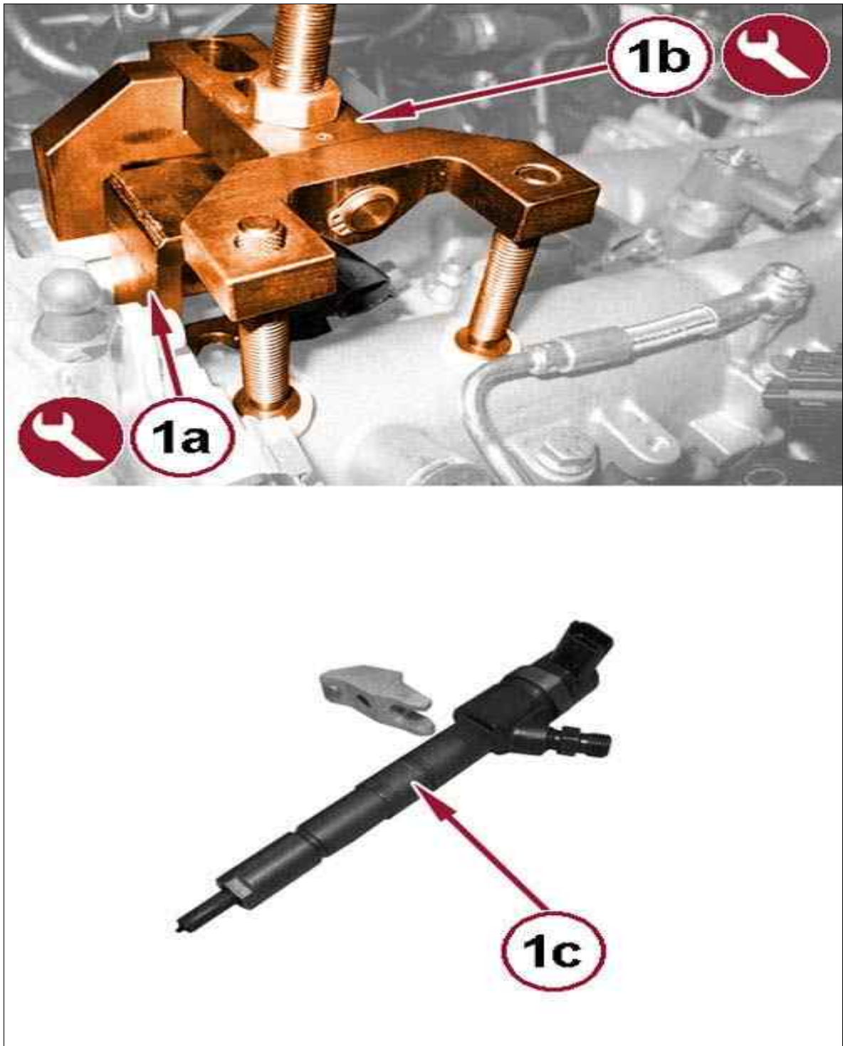
Fig 9: Extractor, Adapter & Fuel Injectors
