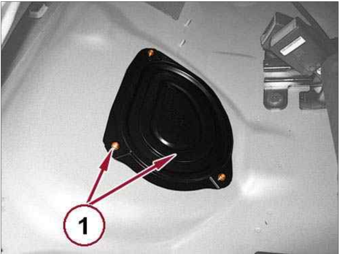
Fig 1: Fuel Pipes Access Cover & Screws
