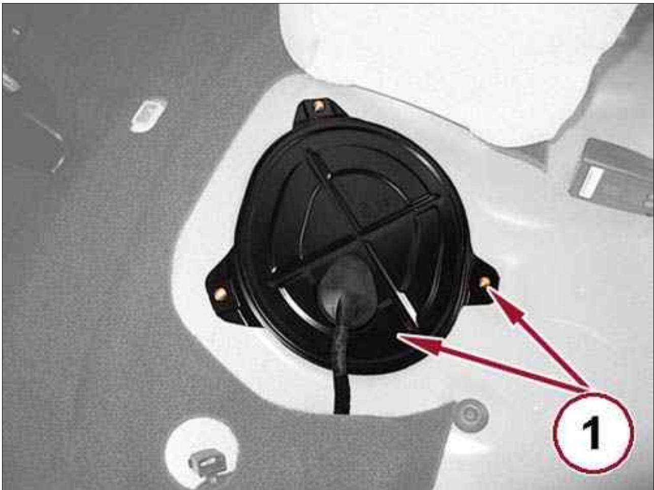
Fig 1: Fuel Pump Access Cover & Screws
