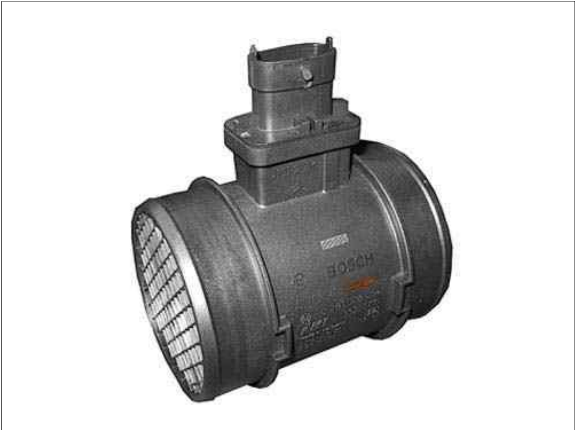
Fig 1: Mass Air Flow Sensor
