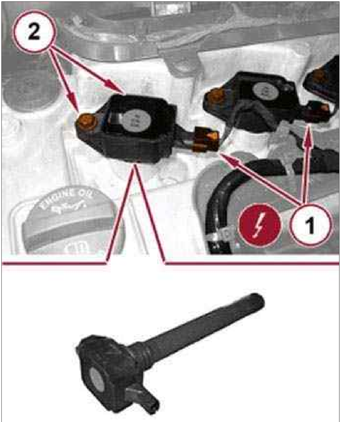
Fig 1: Ignition Coil Electrical Connectors & Mounting Bolts
