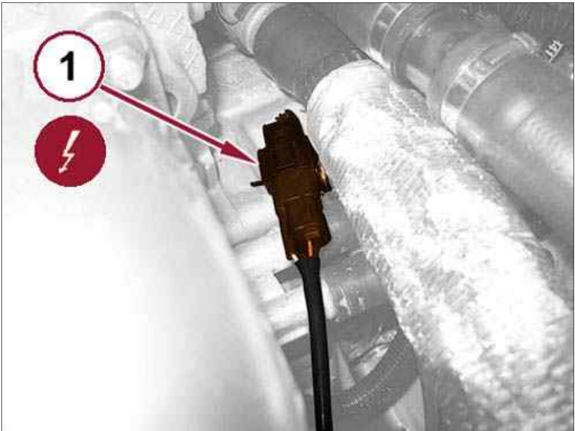
Fig 1: Upstream Oxygen Sensor Electrical Connection
