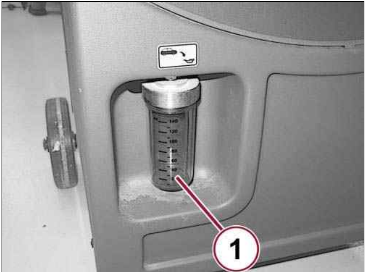
Fig 3: Compressor Oil Container
