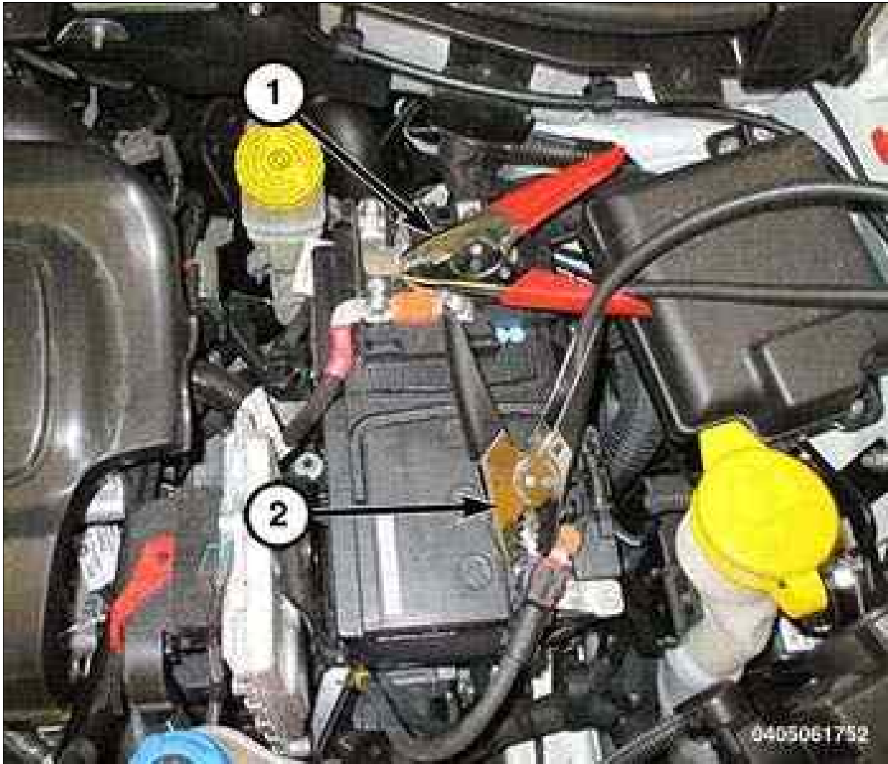
Fig 1: Positive (+) & Negative (-) Battery Jumper Cables
