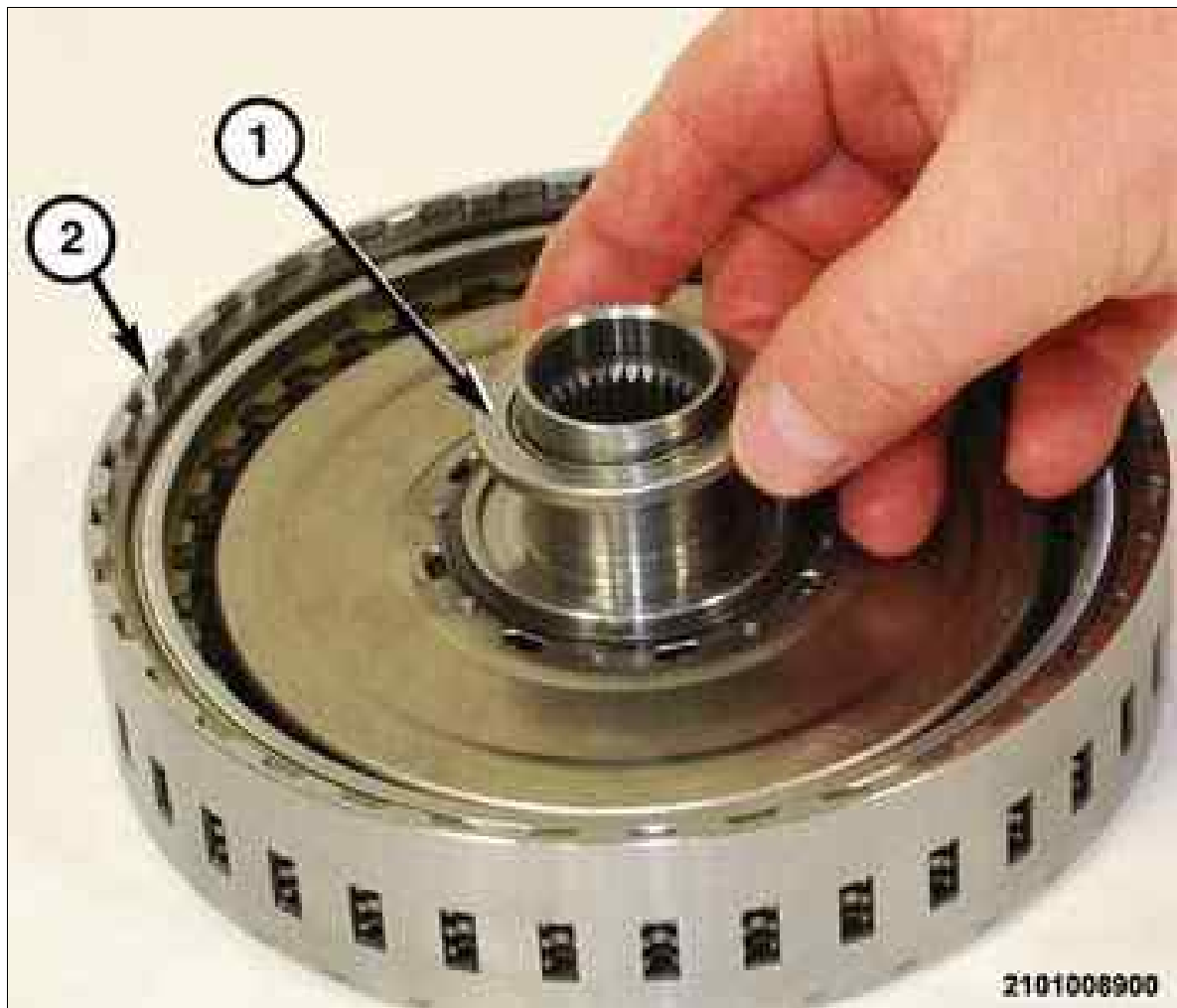
Fig 16: Removing/Installing Thrust Bearing At E-Clutch Assembly
