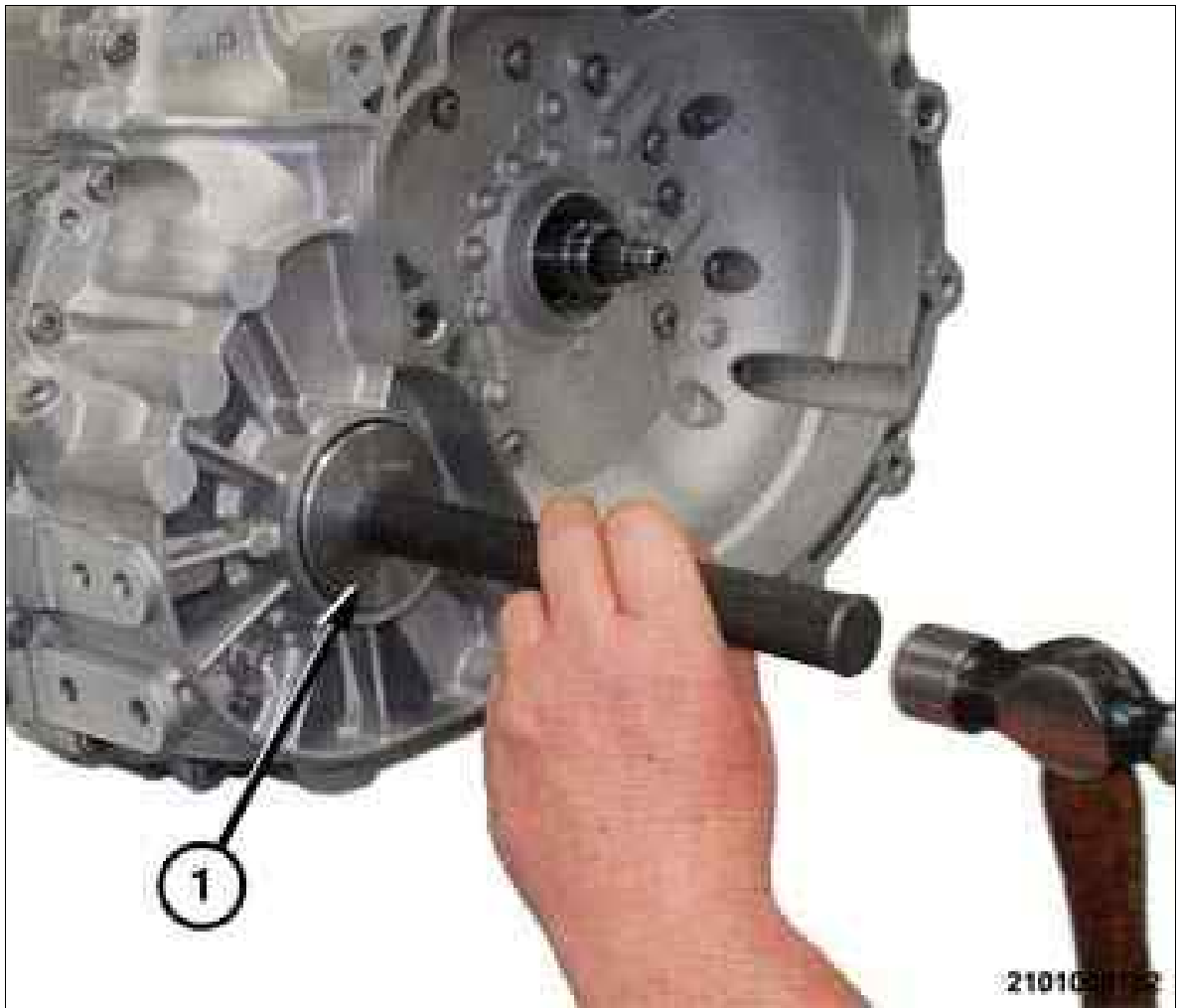
Fig 2: Installing Seal Into Transmission
