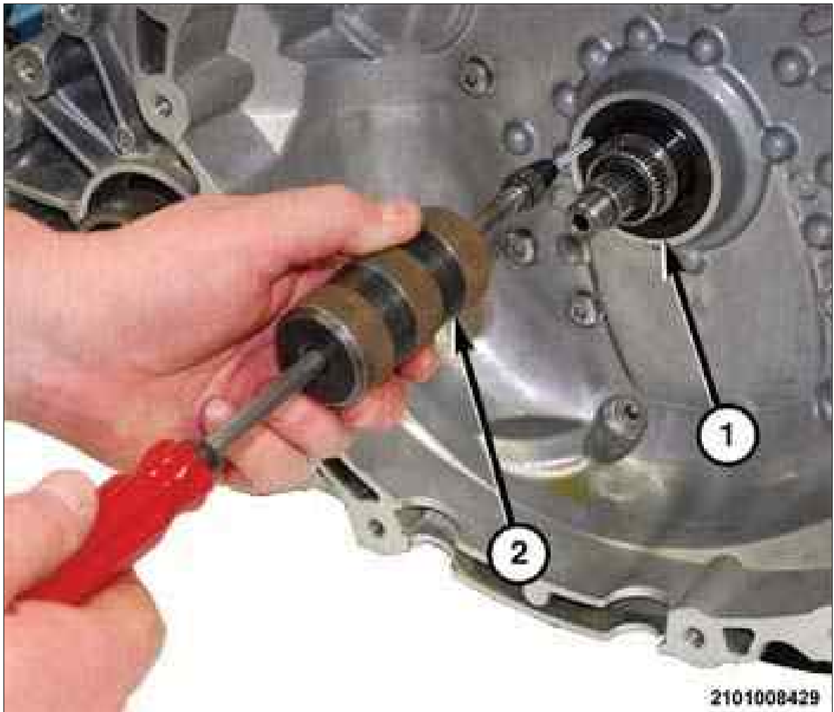
Fig 1: Removing Seal From Center Of Bellhousing
