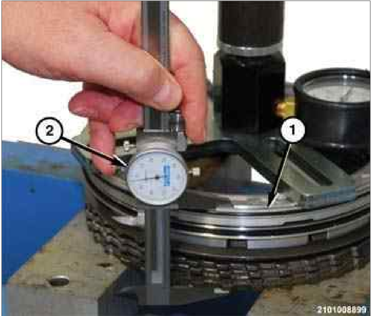
Fig 3: Measuring Thickness From Snap-Ring Step In D-Clutch Piston Retainer To Underside Of D-Clutch Reaction Plate Using Caliper
