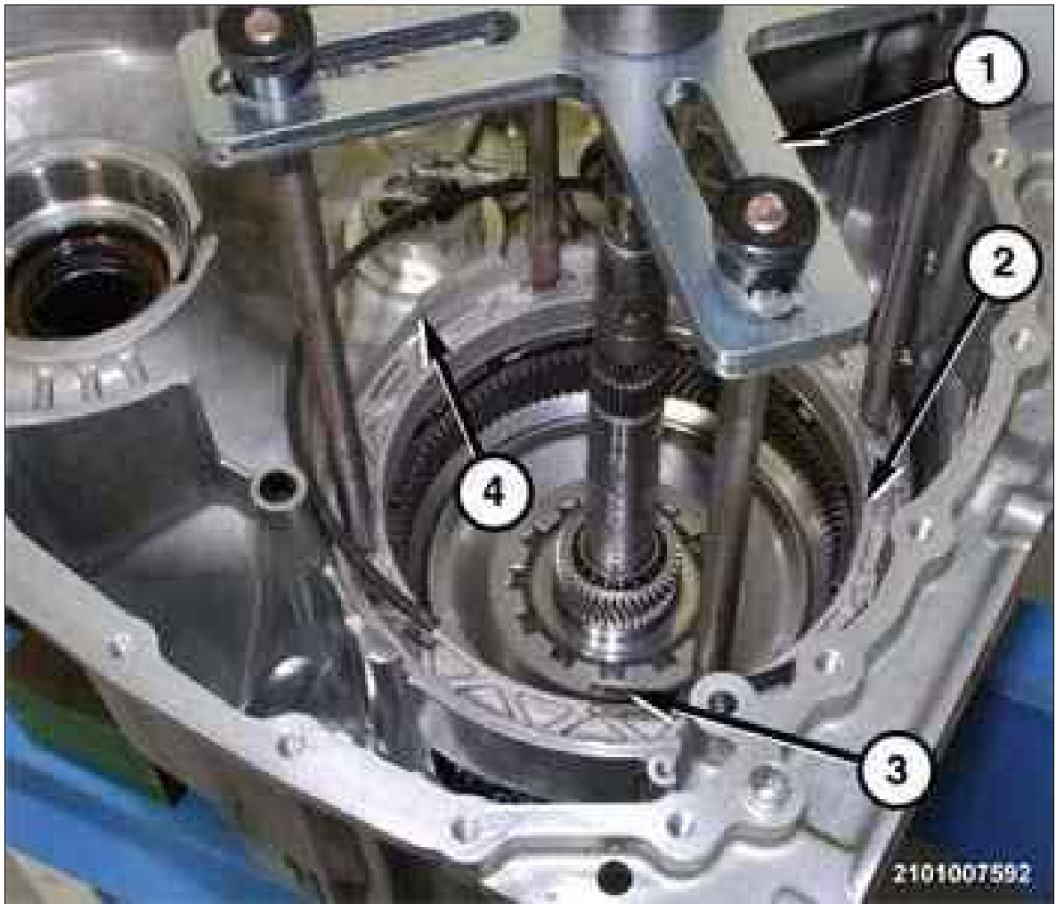
Fig 34: Snap Ring, D-clutch Piston Retainer, Transmission Housing & Special Tool
