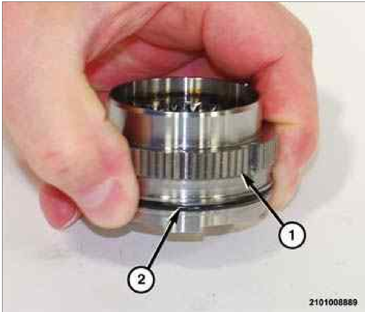
Fig 3: Installing New Outer O-Ring Seal Into The Dog F-Clutch Piston
