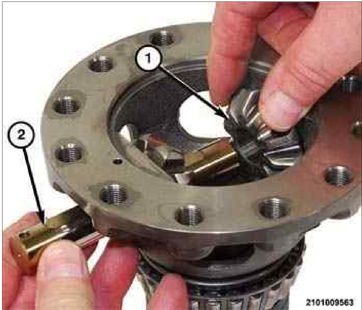
Fig 4: Removing/Installing Pinion Gear 1
