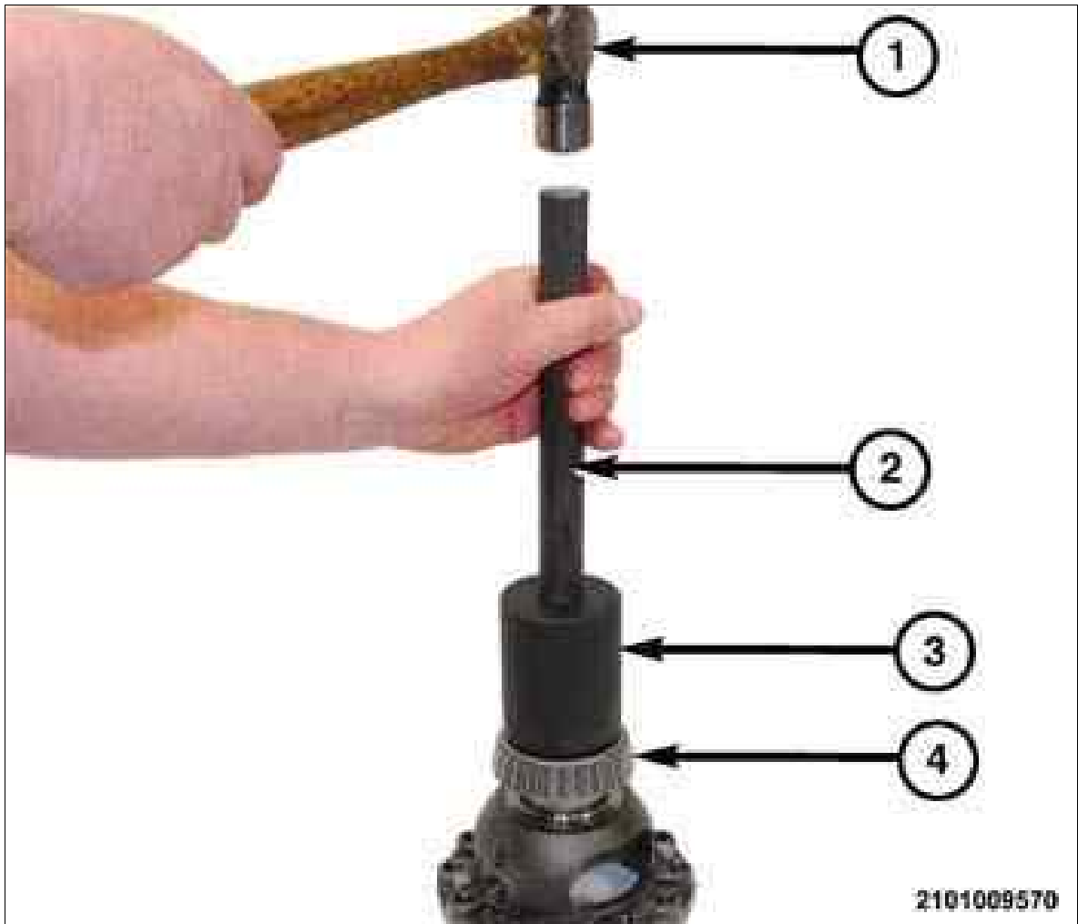
Fig 1: Installing Differential Side Bearing
