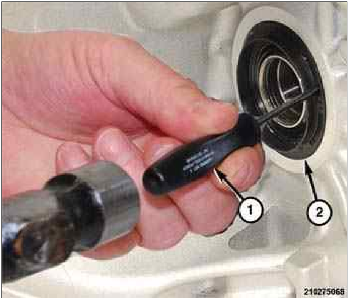
Fig 1: Punching Hole In Differential Seal
