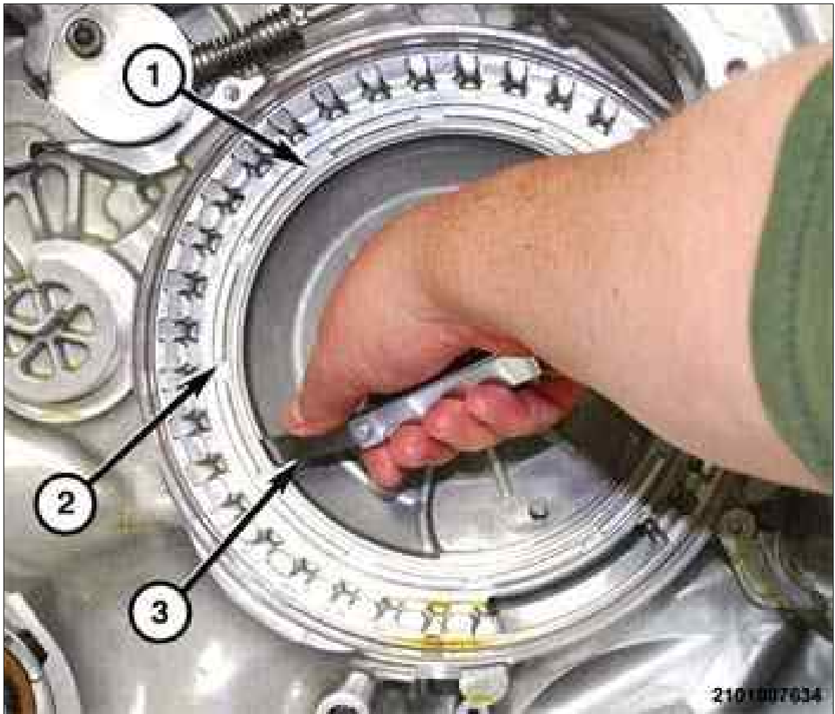
Fig 7: Using Feeler Gauge To Turn Lip On Seal
