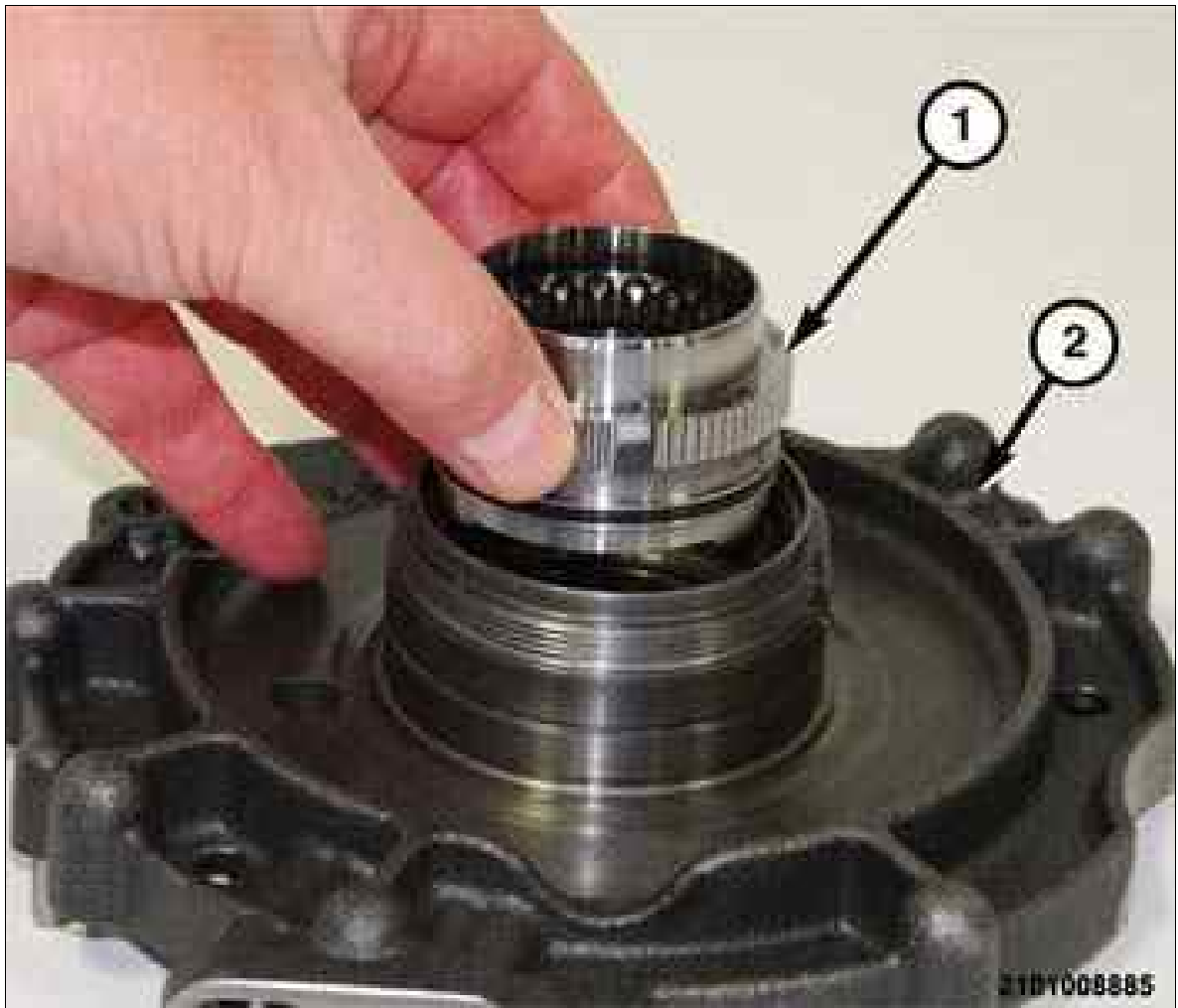
Fig 5: Installing Dog F-Clutch Piston Into The Output Gear Support Hub
