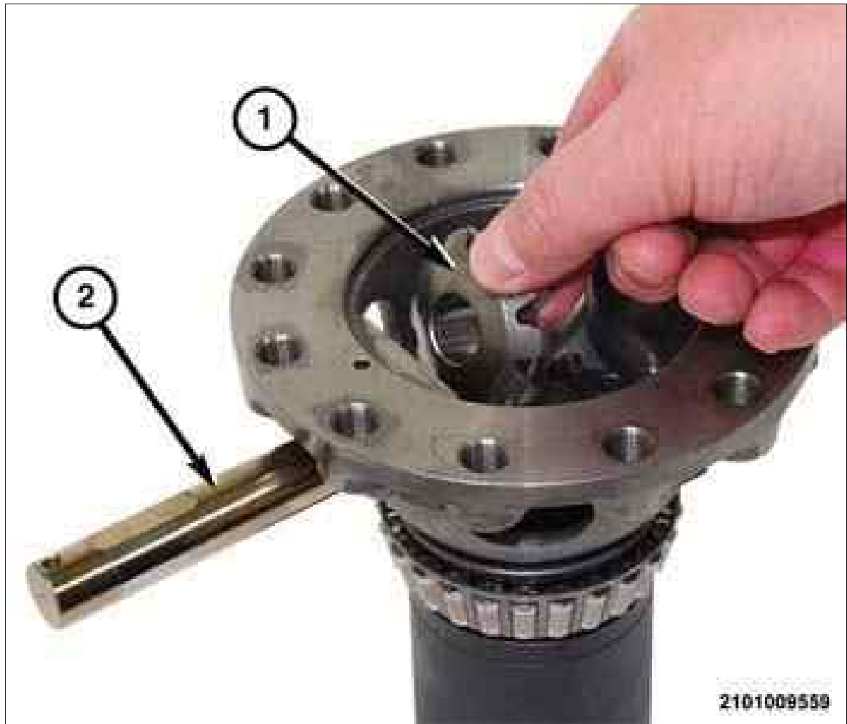
Fig 3: Removing/Installing Pinion Shaft & Pinion Gear 2
