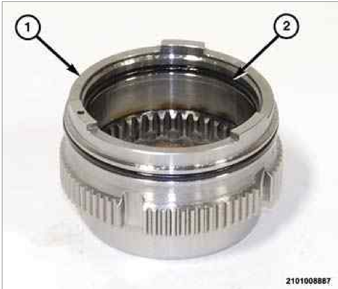
Fig 2: Installing New Inner O-Ring Seal Into The Dog F-Clutch Piston
