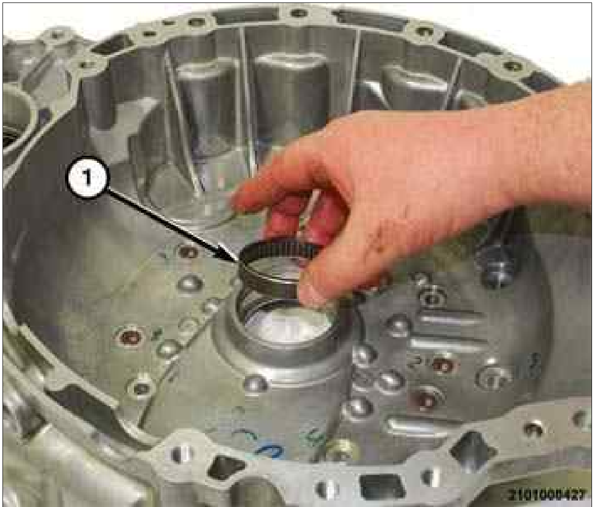
Fig 1: Installing Oil Pump Sprocket Needle Bearing Into Bellhousing
