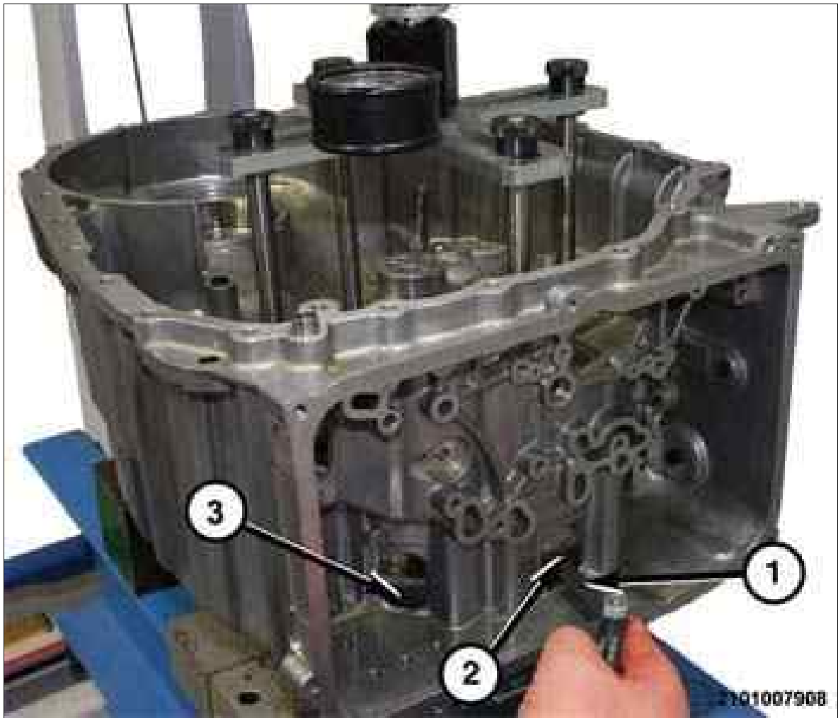
Fig 2: Measuring Gap Between C-Clutch Snap-Ring & Reaction Plate
