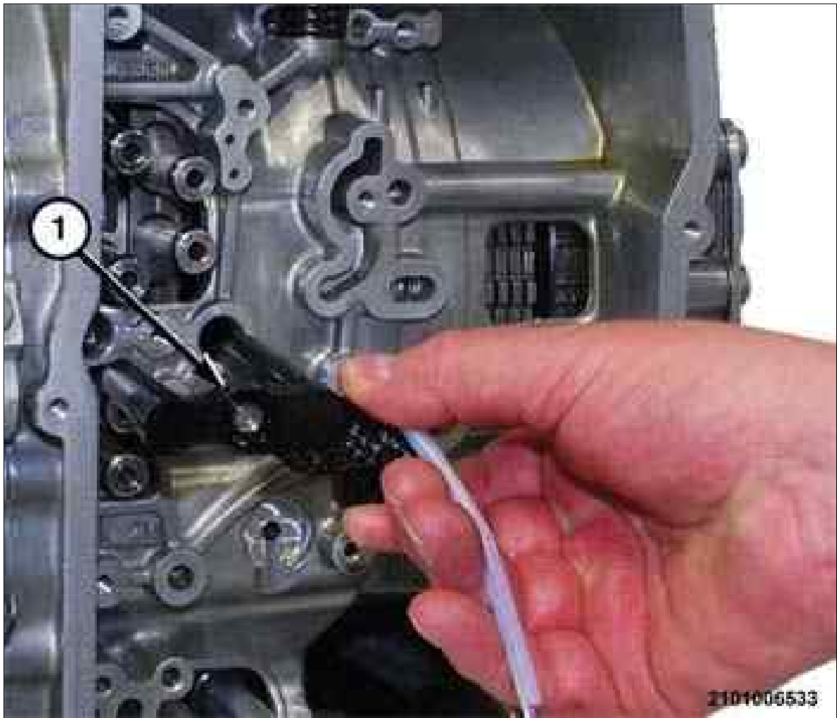
Fig 2: Removing/Installing Speed Sensor
