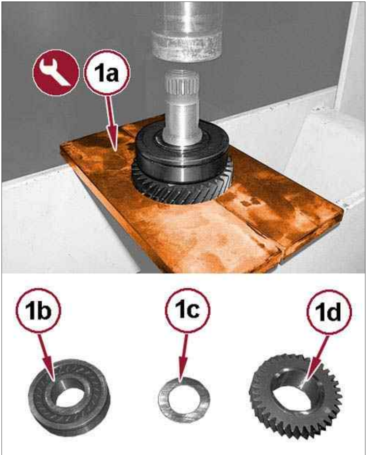
Fig 43: Rear Bearing, Spacer, 4th Gear Drive Gear & Special Tool
