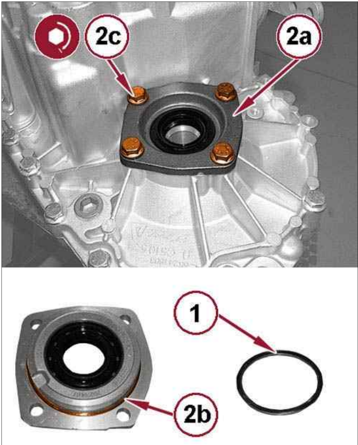
Fig 45: Thrust Washer, Left Axle Seal, Gasket & Bolts
